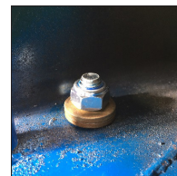
DO NOT FIT DISC SPRINGS LIKE THIS
