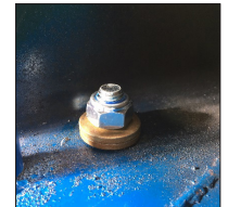
DO NOT FIT DISC SPRINGS LIKE THIS
