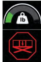
**NOTE:** *If the Overload Indicator is illuminated, further elevation will be prevented. Reduce the weight in the platform so as to not exceed the rated workload indicated on the capacity decal, then the controls will work again.*
