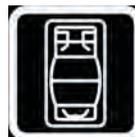
10. **System Fault Indicator** - When a system fault has been detected, the upper right hand corner of the display will show the DTC readout. Additionally, the system fault indicator will flash the appropriate distress code.
