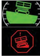
4. **Platform Load Gauge** - Displays the calculated load on the platform. The gauge bar remains green if platform load is less than the rated capacity. If the platform is determined to be overloaded, a red warning light on the display illuminates and an audible alarm sounds.
