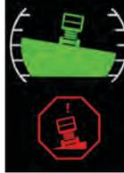
3. **Front to Back Tilt** - Shows the current level of front to back tilt. A red warning light on the display illuminates and an audible alarm sounds when the chassis is at or beyond the tilt cutout settings.
