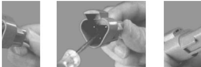
Figure 6-13. DT/DTP Contact Removal
