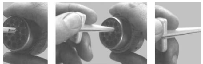
Figure 6-16. HD/HDP Contact Removal
