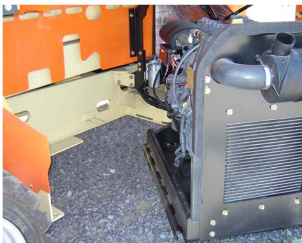
Figure 3-70. Engine Tray Swing
