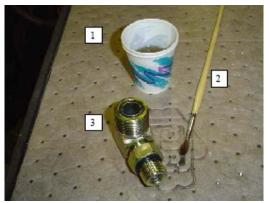
Hold the fitting in one hand while using the brush with the other hand to dip into the container. Remove excess hydraulic oil from the brush so an even film of oil is applied on the o-ring.
