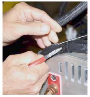
5. Cut wire 106 going to the Engine/Generator Controller after the existing connection point and install the conductors that lead to the new inline fuse holder. Use insulated butt splice connectors for these conductors.
