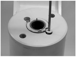
Using a 1/8" (3.18mm) drill bit, drill a hole in the center of each lock pin to a depth of approximately 3/ 16" (4.76mm).
