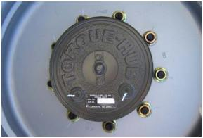
Lube Point(s) - Level/Fill Plug Capacity - 0.4 gal. (1.5 L) Lube - EPGL Interval - Check level every 3 months or 150 hrs of operation; change every 2 years or 1200 hours of operation
