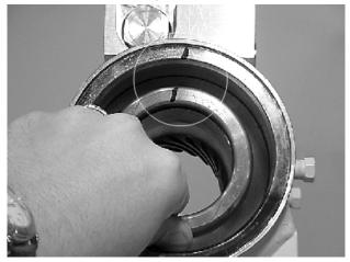
**14.** Remove the o-ring (204) and backup ring (207) from end cap (4) and set aside for inspection.
