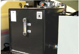
Lube Point(s) - Fill Cap Capacity -Prior to S/N 51941 - 15 gal. tank (56.7 L) S/N 51941 to present - 15.9 gal. system (56.7L) 12.4 gal. (46.9 L) to Full Mark Lube - HO Interval - Check Level daily; Change every 2 years or 1200 hours of operation. 4. Hydraulic Filter
