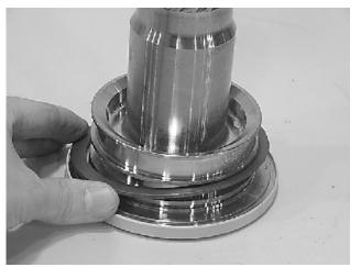
**3.** Install the wiper seal (304.1/green 0-ring) into it's groove on the shaft (2) and end cap (4) around the outside edge of the thrust washer (304).
