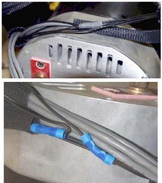
6. Re-install the harness with the new fuse in place.
