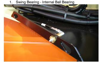
Lube Point(s) - 1 Grease Fittings Capacity - A/R Lube - MPG Interval - Every 3 months or 150 hrs of operation 2. Generator Engine (If Equipped)
