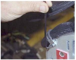
**4.** Cut and remove the Wire Ties holding the Harness label to the harness. Next, remove the Wire Ties so
