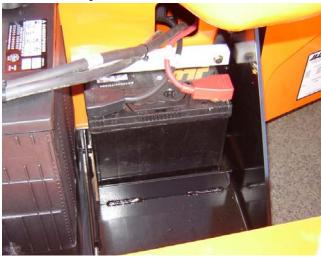
The RBS requires a 12V lead-acid start battery (not supplied with the system), which provides starting power and power for the RBS controls.
