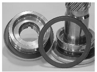
2. Install the thrust washer (304) onto shaft (2) and end cap (4).
