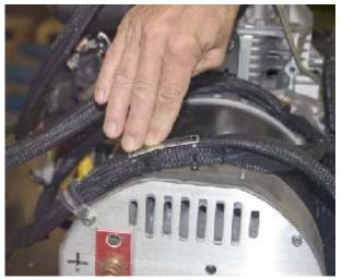
**3.** Remove the socket head drive screw with a 5/32" Allen key. Next remove the cable clamp from the harness.
