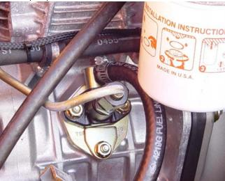
**4.** When fuel starts to flow out of the rubber line, reconnect the fuel line to the fuel injector pump.
