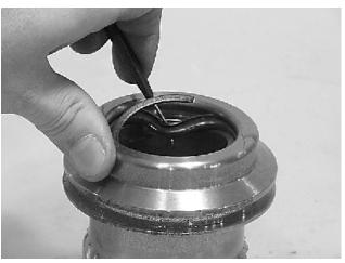
**18.** Remove the wiper seal (304.1) from its groove in the end cap (4) and shaft (2).
