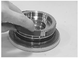
**6.** Install the inner T-seal (200) into the piston (3) using a circular motion.
