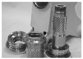
Inspect the thrust washers (304) for rough or worn edges and surfaces. Measure it's thickness to make sure it is within specifications (Not less than 0.092" or 2.34 mm).
