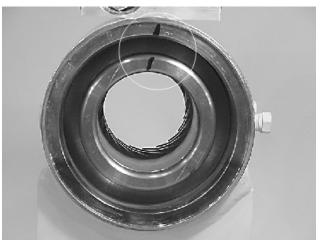
**9.** Looking from the opposite end of the housing (1) you can see if your timing marks are lining up. When they do, tap the piston (3) in until the gear teeth mesh together. Tap the piston into the housing the rest of the way until it bottoms out.
