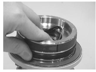
**16.** Thread the end cap (4) onto the shaft (2) end. Make sure the wear guide stays in place on the end cap as it is threaded into the housing (1).
