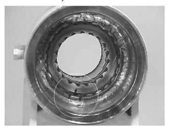
Install the shaft (2) into the piston (3). Be careful not to damage the seals. Do not engage the piston gear teeth yet.
