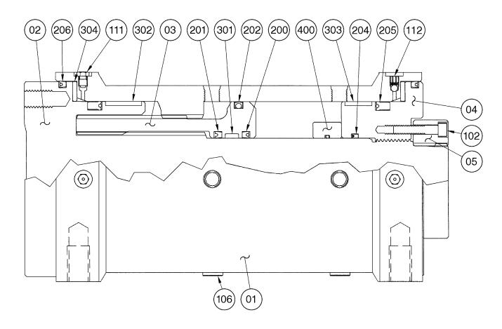
1. Housing 111. Grease Fitting 205. Bearing Seal 2. Shaft 206. Exclusion Seal 112. Grease Relief Valve 3. Piston Sleeve 400. Stop Tube 301. Piston Bearing 4. End Cap 200. Rod Seal 302. Shaft Bearing 5. Lockring 201. Rod Seal 303. Shaft Bearing 304. Thrust Washer 102. Socket Head Capscrew 202. Piston Seal 106. Port Plug 204. Cap Seal
