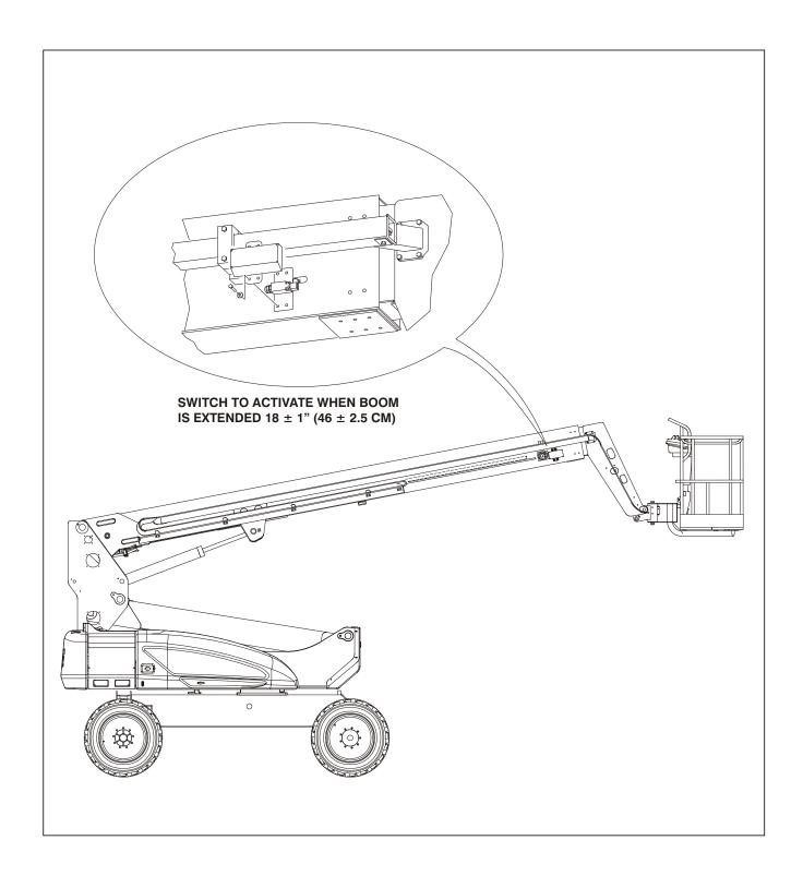
Figure 4-5. Transport Limit Switch (CE Only)
