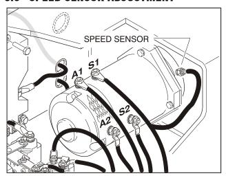
For proper drive operation, the speed sensors must be properly installed and adjusted. The sensor operates on a leading pulse to show direction. If installed wrong, the sensor will not be able to sense the proper direction.
