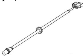
The engine speed sensor provides a signal proportional to the rotational speed of the engine to the engine/generator controller. This signal is used by the engine/generator controller to determine starter cut-out, overspeed fault and underspeed fault. If the signal is not present at the engine/generator controller, the unit will fault with a loss of speed signal indication.
