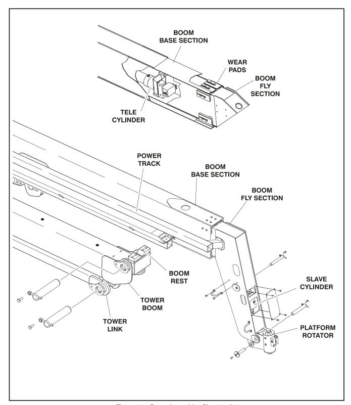
Figure 4-2. Boom Assembly - Sheet 2 of 3
