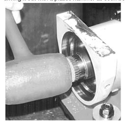
Before the shaft and piston gearing are completely disengaged, note the orientation between the spline teeth: small punch marks on the face of the piston
