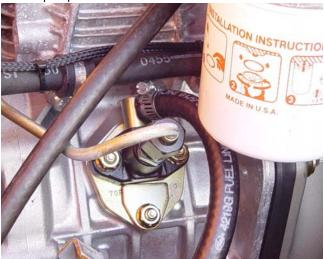
When fuel starts to flow out of the rubber line, reconnect the fuel line to the fuel injector pump.
