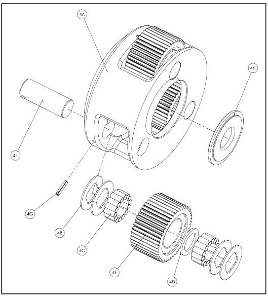
4A Output Carrier4B Thrust Washer4E Planet Shaft4F Planet Gear
