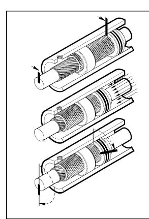
Bars indicate starting positions of piston and shaft. Arrows indicate direction they will rotate. The housing's ring gear remains stationary.
