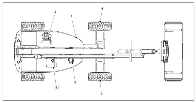
Figure 1-2. Operator Maintenance and Lubrication Diagram
