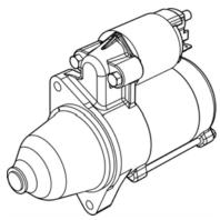
The engine is equipped with a 12VDC starter, which provides the mechanical power to crank the engine. Electrical power for the starter is provided by the start battery.
