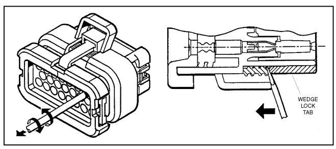
Figure 7-10. Connector Disassembly
