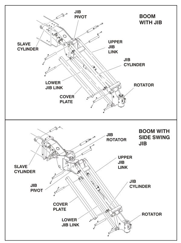
Figure 4-3. Boom Assembly - Sheet 3 of 3
