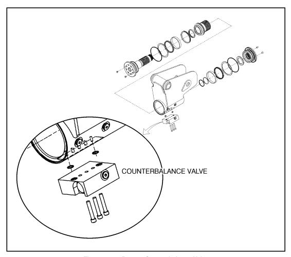
Figure 4-14. Rotator Counterbalance Valve
