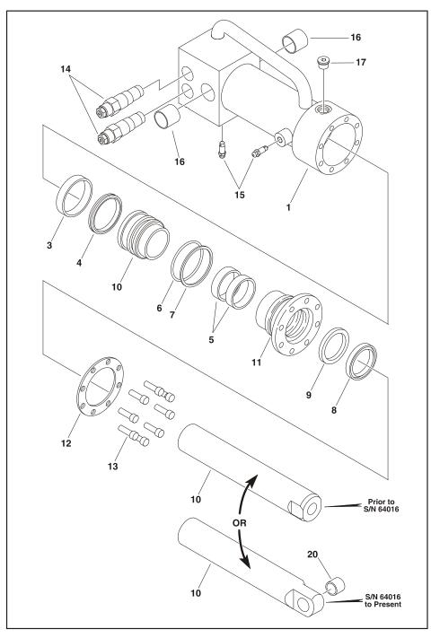
6. O-ring7. Backup Ring11. Cap12. Washer Ring 16. Bushing 1. Barrel 2. Not Used 17. O-ring Plug 3. Wear Ring 8. Wiper Ring 13. Bolt 18. Loctite #242 4. T-Seal 9. Seal 14. Counterbalance Valve 19. Locking Primer (Not Shown) 10. Rod 15. Bleeder Valve 20. Bushing 5. Wear Ring
