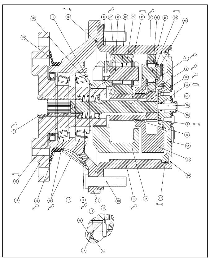
Figure 3-9. Hub Assembly - Sheet 1 of 2
