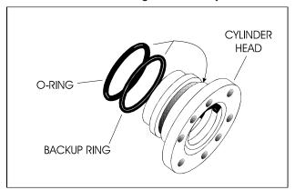
Figure 5-15. Installation of Head Seal Kit
