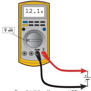
Figure 7-1. Voltage Measurement (DC)
