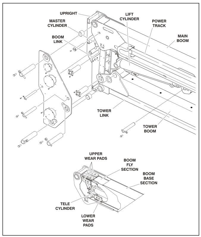
Figure 4-1. Boom Assembly - Sheet 1 of 3
