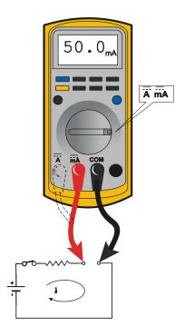
Figure 7-4. Current Measurement (DC)
