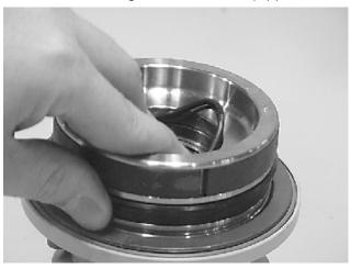
**16.** Thread the end cap (4) onto the shaft (2) end. Make sure the wear guide stays in place on the end cap as it is threaded into the housing (1).
