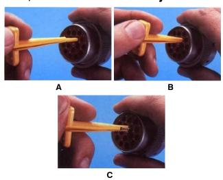
Figure 7-16. HD/HDP Contact Removal
