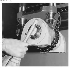
A considerable amount of torque may be required to loosen the end cap. Completely filling the length of the screws with a stack of washers or a bushing as seen in the illustration to the right will permit more force to be applied to the screws and prevent them from bending - be sure to thread the screws completely into the endcap. If the end cap is difficult to break loose, special tooling may be fabricated according to the drawing below.
