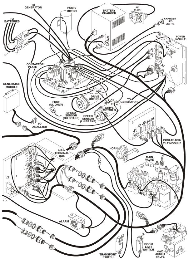
Figure 7-19. Electrical Components Installation - Sheet 2
