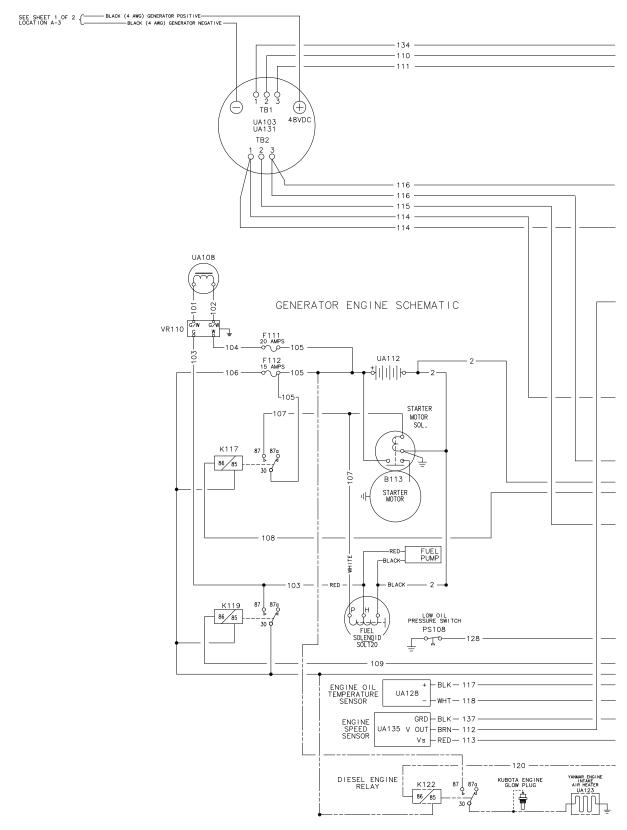
Figure 7-22. Electrical Schematic - Sheet 3 of 4
