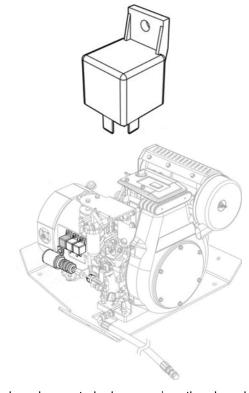
The glow plug control relay energizes the glow plug. It is energized by the engine/generator controller, pin J2-27.
