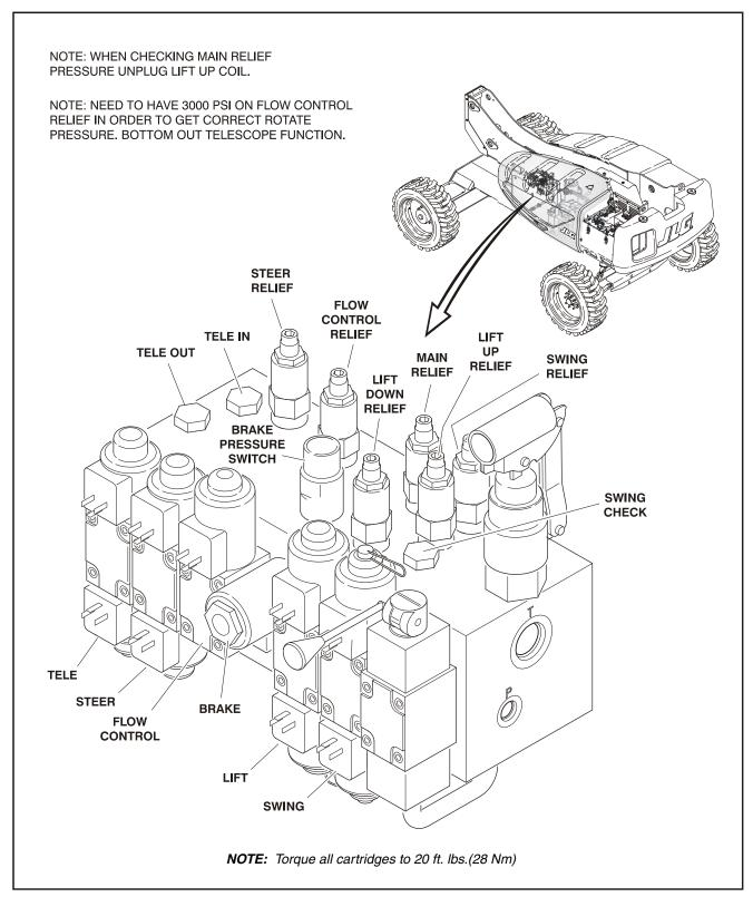
Figure 5-23. Hydraulic Control Valve - Main Valve
