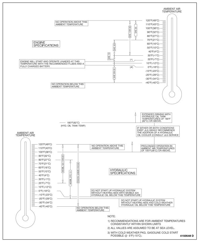
Figure 2-1. Operating Temperature Specifications - Kubota
