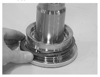
3. Install the wiper seal (304.1/green 0-ring) into it's groove on the shaft (2) and end cap (4) around the outside edge of the thrust washer (304).
