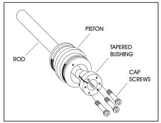
Figure 5-11. Tapered Bushing
