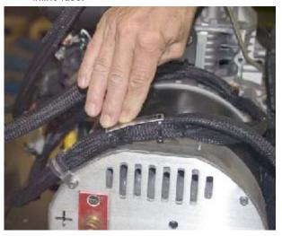
Remove the socket head drive screw with a 5/32" Allen key. Next remove the cable clamp from the harness.
