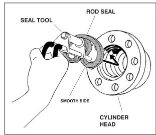
Figure 5-13. Rod Seal Installation
