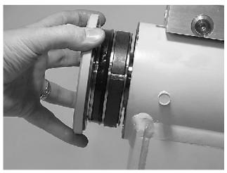
11. Before removing the piston (3), mark the housing (1) ring gear in relation to the piston O.D. gear. There should now be timing marks on the housing (1) ring gear, the piston (3) and the shaft (2).
