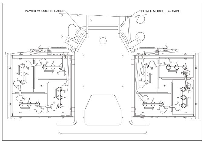
Figure 3-29. Battery Cable Routing
