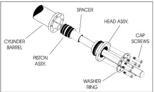
Figure 5-20. Rod Assembly Installation
