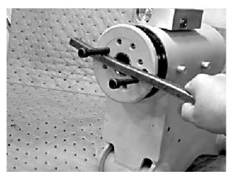
**13.** Install the stop tube onto the shaft end. Stop tube is an available option to limit the rotation of an actuator.
