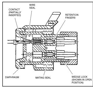
Figure 7-5. Connector Assembly Figure 1
