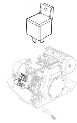
The start control relay energizes the solenoid of the engine starter and the pull coil of the engine fuel solenoid.
