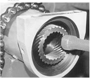
Support the piston sleeve as it is removed from the housing. Great care should be taken to insure that the gear teeth are not damaged and the piston sleeve does not damage the housing bore as it is removed.
