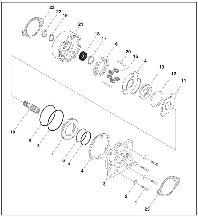
1. Capscrew 7. Piston 13. Rotor Disc 19. Retaining Ring 2. Washer 8. O-ring 14. Plate 20. Dowel Pin 3. Pressure Plate 9. Backup Ring 21. Cover 15. Spring 16. Spring Retainer 22. Rotary Oil Seal 4. Case Seal 10. Shaft 5. O-ring 11. Stator Disc 17. Retaining Ring 23. Gasket 12. Sensor Ring 18. Bearing
