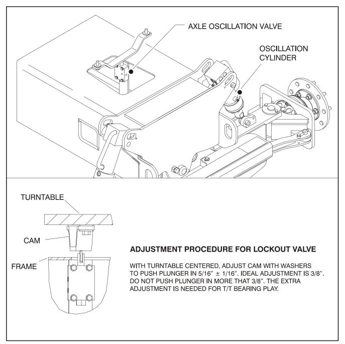
Figure 3-17. Axle Oscillation Lockout Valve
