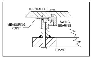
Figure 3-26. Swing Bearing Tolerance Measuring Point
