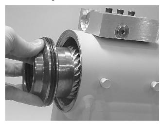
8. Looking from the angle shown, rotate the piston (3) until the marks you put on the piston and the housing (1) during disassembly line up as shown. Using a rubber mallet, tap the piston into the housing up to the point where the gear teeth meet.
