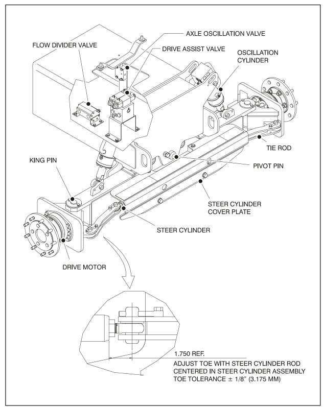
Figure 3-16. Oscillating Axle
