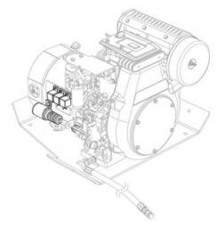
The engine is equipped with a low oil pressure switch. This switch is closed when the oil pressure is below 7psi. It is mounted on the side cover.
