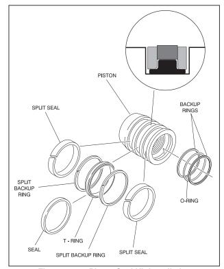
Figure 5-16. Piston Seal Kit Installation
