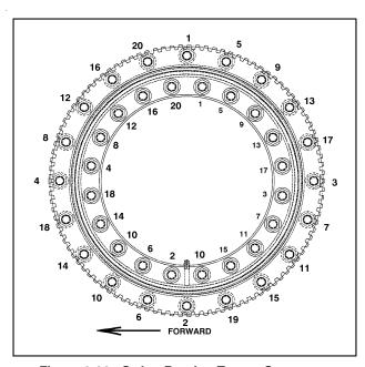
Figure 3-28. Swing Bearing Torque Sequence
