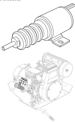
The fuel solenoid actuates the run/stop lever of the engine. This solenoid has a pull coil energized by the start control relay and a hold coil energized by the fuel control relay.
