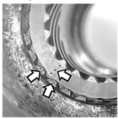
The adjacent weld can make the ring gear timing marks difficult to locate; using a light can help. Again, mark the teeth with a felt tip marker to make the marks easier to see and to simplify timing during reassembly. Drive the piston sleeve out of the hous-
