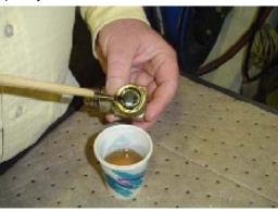
Turn the o-ring on the other side of the fitting and repeat the previous step, ensuring the entire o-ring is coated with hydraulic oil.
