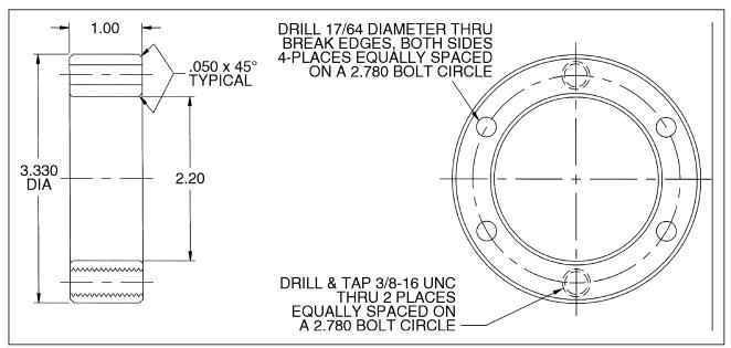
Figure 4-13. Tool for Removing End Cap
