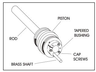
Figure 5-18. Seating the Tapered Bearing
