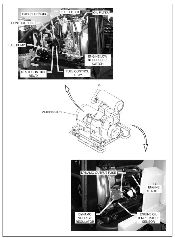
Figure 3-33. Generator Components
