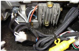
The engine is equipped with a dynamo and dynamo voltage regulator.
