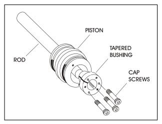
Figure 5-17. Tapered Bushing Installation
