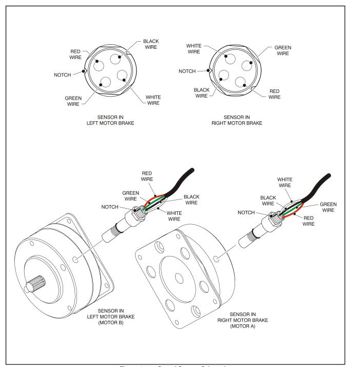
Figure 3-14. Speed Sensor Orientation
