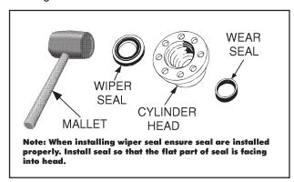
Figure 5-14. Wiper Seal Installation
