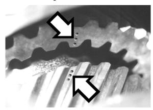
Marking the teeth at this time with a permanent felt tip marker will make the marks easier to see and greatly simplify actuator timing during reassembly. For 120° rotation actuators, remove the stop tube from the shaft before removing the shaft from the housing. Do not remove the 0-ring from the stoptube. It performs no sealing functions and should be reused when the actuator is reassembled.
