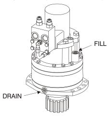
Capacity - 24 oz. (0.7 L) Lube - EPGL Interval - Check level every 3 months or 150 hrs of operation; change every 2 years or 1200 hours of operation
