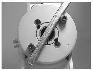
**18.** Place the lock pins (109) provided in the Helac seal kit in the holes with the dimple side up. Then, using a punch, tap the lock pins to the bottom of the hole.
