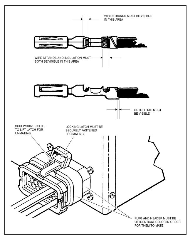
Figure 7-11. Connector Installation
