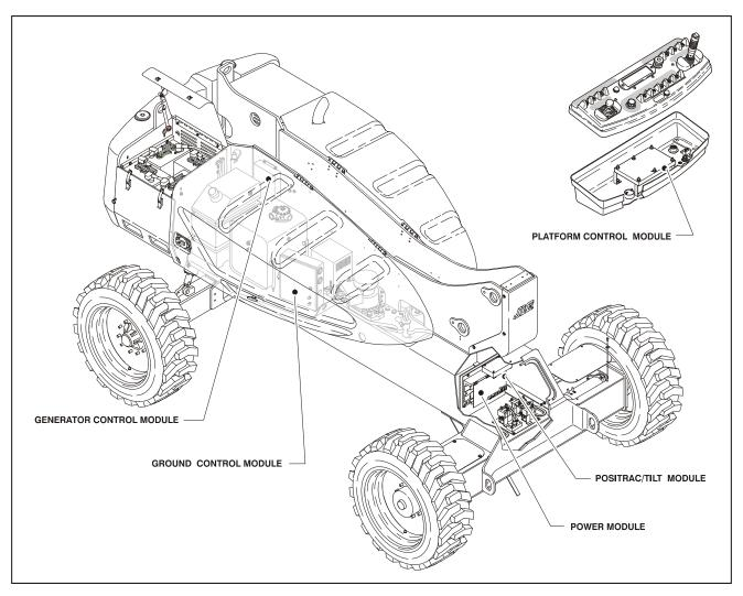
Figure 6-4. Control Module Location
