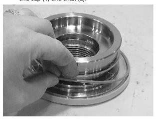
19. Remove the piston O.D. seal (202).
