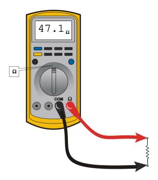
Figure 7-2. Resistance Measurement
