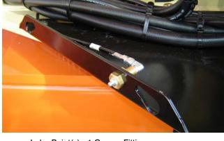
Lube Point(s) - 1 Grease Fittings Capacity - A/R Lube - MPG
