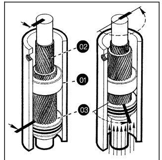
Bars indicate starting positions of piston and shaft. Arrows indicate direction they will rotate. The housing with integral ring gear remains stationary. As fluid pressure is applied, the piston is displaced axially while the helical gearing causes the piston and shaft to rotate simultaneously. The double helix design compounds rotation: shaft rotation is about twice that of the piston.
