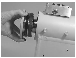
11. Looking from the view shown, use the existing timing marks to line up the gear teeth on the shaft (2) with the gear teeth on the inside of the piston (3). Now tap the flange end of the shaft with a rubber mallet until the gear teeth engage.
