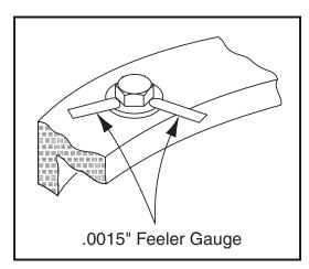
Figure 3-25. Swing Bearing Feeler Gauge Check
