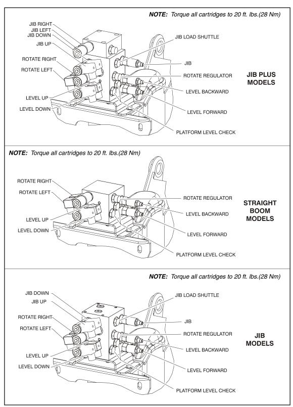
Figure 5-24. Hydraulic Control Valve - Platform Valve
