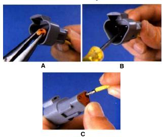
Figure 7-13. DT/DTP Contact Removal
