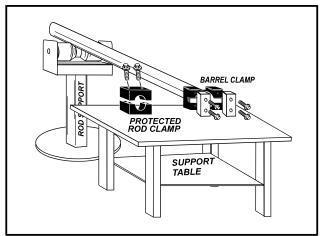
Figure 5-1. Cylinder Barrel Support
