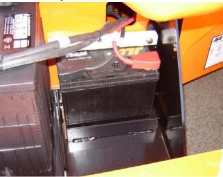
The RBS requires a 12V lead-acid start battery (not supplied with the system), which provides starting power and power for the RBS controls.
