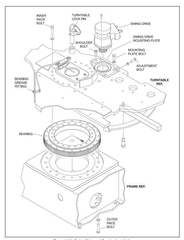
Figure 3-27. Swing Drive and Bearing Installation
