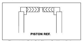
Figure 5-19. Poly-Pak Piston Seal Installation
