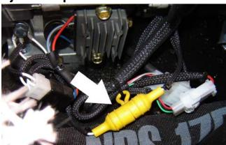
This fuse protects the dynamo output; it is located on the left side of the engine.
