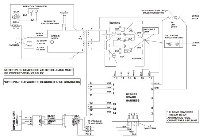
Figure 3-32. Battery Charger Schematic
