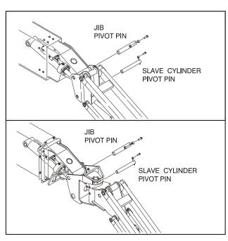
Remove the jib pivot pin and the slave cylinder pivot pin and remove the jib.
