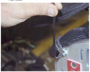
4. Cut and remove the Wire Ties holding the Harness label to the harness. Next, remove the Wire Ties so
