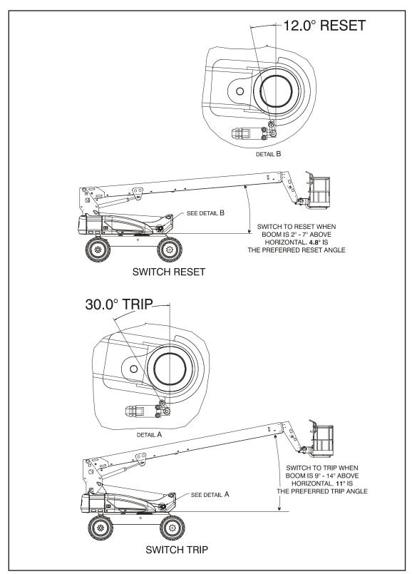
Figure 4-4. Boom Limit Switch Adjustment
