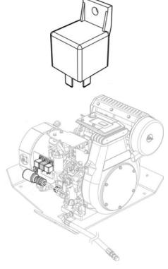
The fuel control relay energizes the hold coil of the fuel solenoid.
