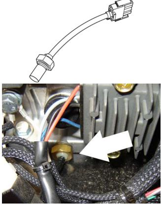
The engine oil temperature sensor is used to sense the temperature of the oil in the sump of the engine.
