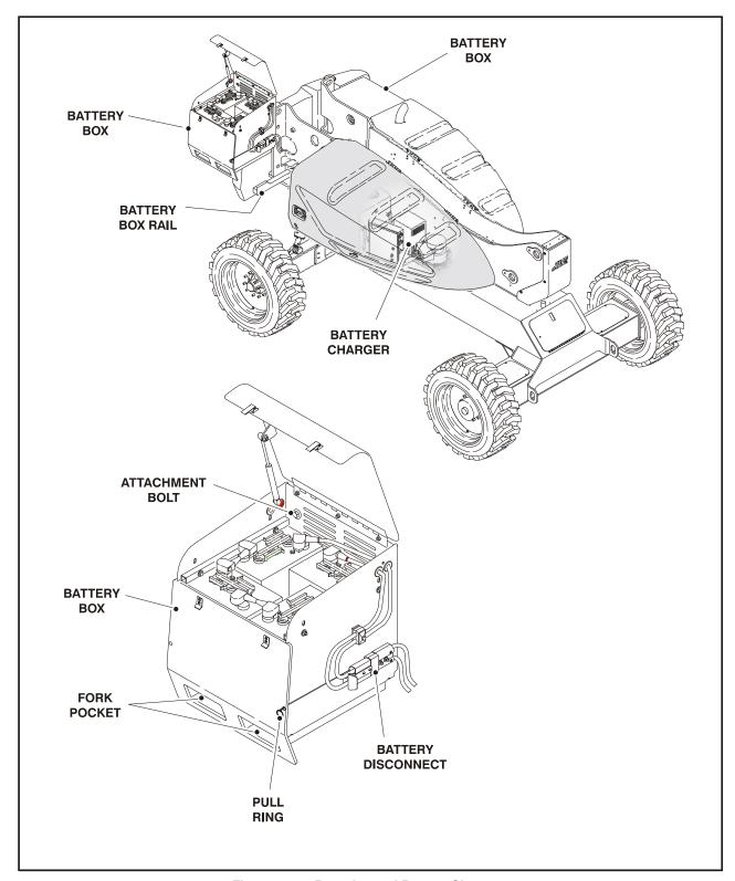
Figure 3-30. Batteries and Battery Charger
