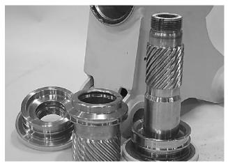
Inspect the thrust washers (304) for rough or worn edges and surfaces. Measure it's thickness to make sure it is within specifications (Not less than 0.092" or 2.34 mm).
