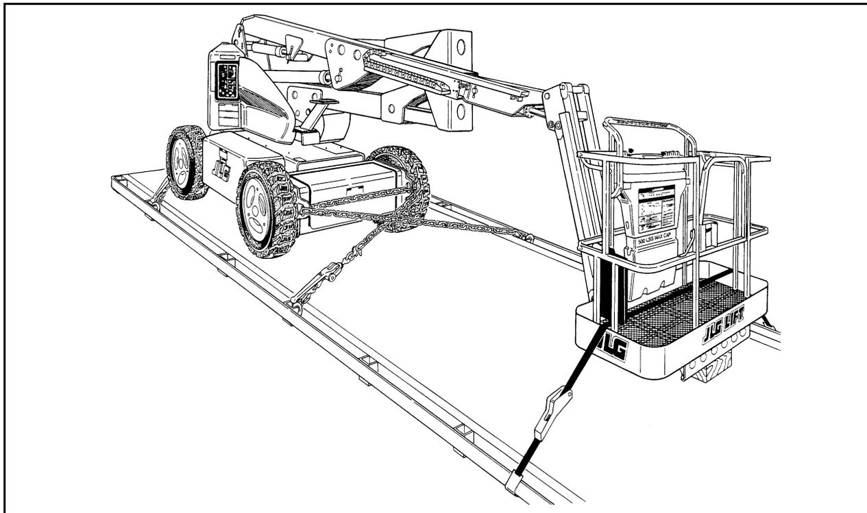
Figure 4-6. Chassis & Platform Tie Down - Sheet 2 of 2
