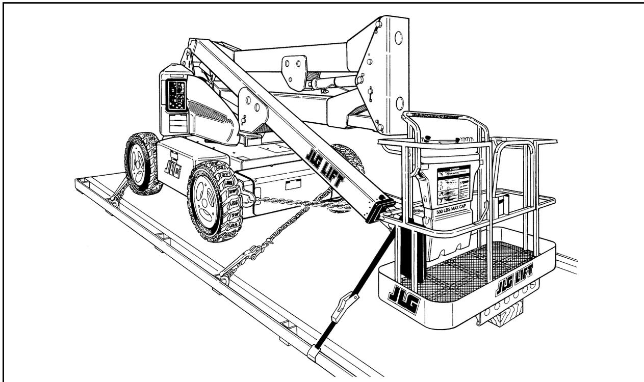
Figure 4-5. Chassis & Platform Tie Down - Sheet 1 of 2
