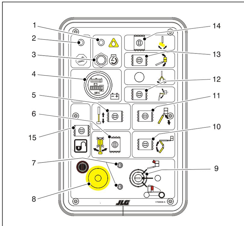
Figure 3-2. Ground Control Station w/ Function Enable
