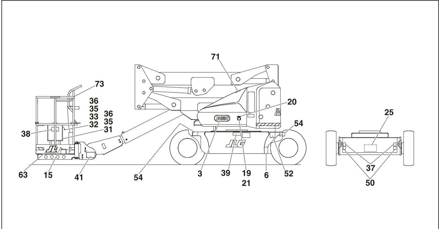
Figure 4-9. Decal Installation - Sheet 3 of 3
