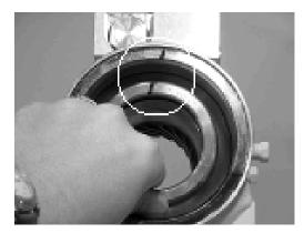
**13.** At the point when the piston gear teeth come out of engagement with the housing gear teeth, mark the piston and housing with a marker as shown.
