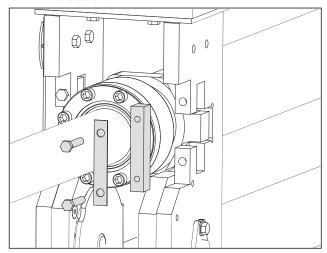
**7.** Remove the four bolts, shims, and mounting blocks that secure the telescope cylinder rod to the boom base section.
