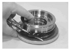
**4.** Using a seal tool install the main pressure seal (205) onto shaft (2) and end cap (4). Use the seal tool in a circular motion.
