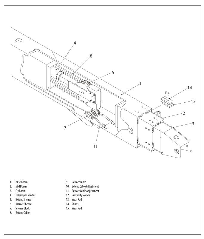
Figure 4-2. Boom Assembly Cutaway - Sheet 2 of 2
