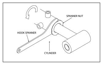
Figure 5-71. Spanner Nut Removal
