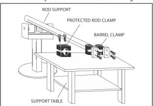
Figure 5-1. Cylinder Barrel Support
