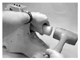
**12.** To remove the piston (3) use a rubber mallet and a plastic mandrel so the piston is no damaged.
