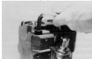
**3.** Remove the port plate together with the valve plate (hold the valve plate so that the plate can't fall down).
