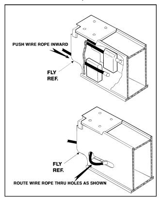
Figure 4-6. Disassembly Wire Rope Routing Procedure
