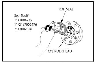
Figure 5-7. Rod Seal Installation
