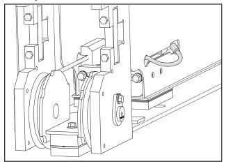
**13.** From the rear of the boom, pull out the boom retraction cables.
