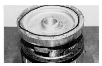
12. The cover (6) is now installed on this assembly. Taking care to correctly align pipe plug hole (20) with those in the hub (1J), usually 90° to one another.
