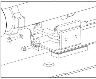
**6.** Remove the four bolts, shims, and attachment blocks that secure the telescope cylinder barrel to the boom mid section.
