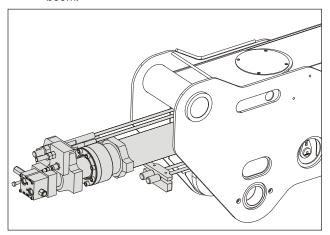
**20.** Apply JLG Threadlocker P/N 0100011 to the bolts and fasten the telescope cylinder rod to the boom base section with the bolts, shims, mounting blocks.
