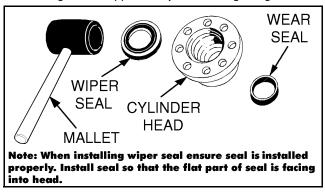
Figure 5-77. Wiper Seal Installation
