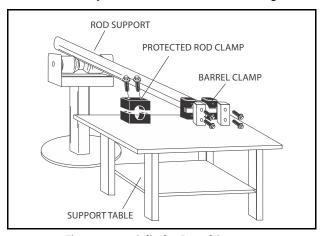
Figure 5-60. Cylinder Barrel Support
