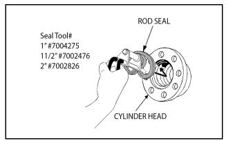
Figure 5-65. Rod Seal Installation
