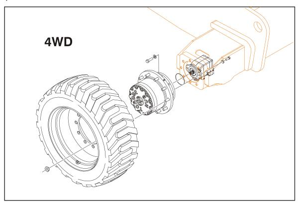
Figure 3-7. Drive Hub Installation - 4WD (Prior to SN 0300083331)
