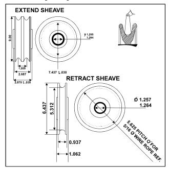
Figure 4-7. Dimension of Sheaves When New
