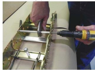
**4.** Hold the flat bar and remove the screws.
