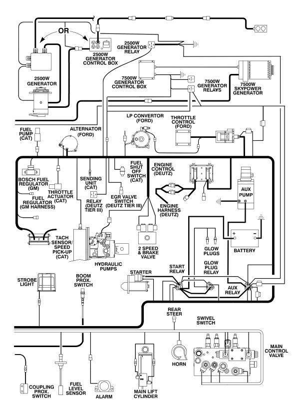
Figure 7-23. Electrical Components Installation (WITHOUT UGM) (SN 0300085332 through 0300140000) - Sheet 2 of 2
