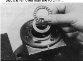
**NOTE:** Torqlinks<sup>™</sup> require one thrust washer (14) with thrust bearing (15).The coupling shaft will be seated directly against the thrust washer.
