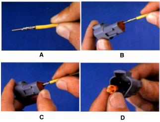
Figure 7-14. DT/DTP Contact Installation
