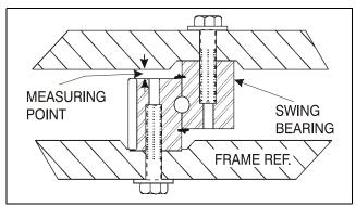
Figure 3-78. Swing Bearing Tolerance Measuring Point.
