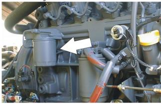
Lube Point(s) - Fill Cap/Spin-on Element Capacity - 11 Quarts(10.5 L) Crankcase; Lube - EO Interval - Every Year or 1200 hours of operation Comments - Check level daily/Change in accordance with engine manual. Refer to Figure 1-2., Deutz Engine Dipstick.
