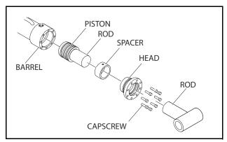
Figure 5-44. Rod Assembly Installation
