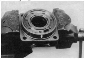
**5.** On the Torqlinks<sup>™</sup> assemble a new backup washer (17) and new seal (16) with the seal lip facing toward the inside of Torqlink<sup>™</sup>, into their respective counterbores in housing (18) if they were not assembled in procedure 2.
