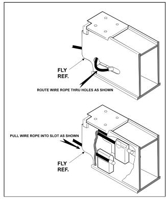
Figure 4-9. Routing Installation of Retract Wire Ropes
