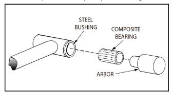
Figure 5-64. Composite Bearing Installation
