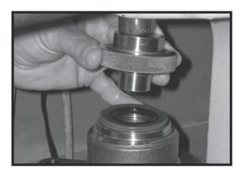
**4.** Place housing (18) assembly into a soft jawed vise with the coupling shaft bore down, clamping against the mounting flange.
