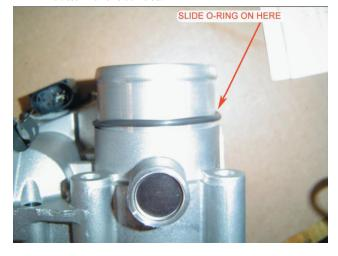
Install the two quad seals. Install one seal at a time to insure the seal does not roll. The seal must sit flat on the throttle body.
