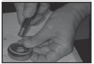
9. Remove manifold (7) and inspect for cracks surface scoring, brinelling or spalling. Replace manifold if any of these conditions exist. A polished pattern on the ground surface from commutator or rotor rotation is normal. Remove and discard the seal rings (4) that are on both sides of the manifold.
