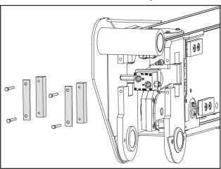
**11.** Apply JLG Threadlocker P/N 0100011 to the bolts and fasten the telescope cylinder barrel to the boom mid section with the bolts, shims, mounting blocks.
