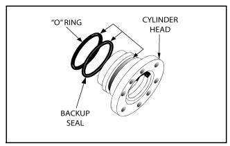
Figure 5-89. Installation of Head Seal Kit
