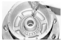
**8.** Place internal gear (12) onto end of spindle.
