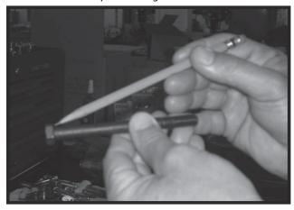
**10.** Remove end cover assembly (2) and seal ring (4). Discard seal ring.
