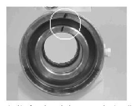
9. Looking from the angle shown, rotate the piston (3) until the marks you put on the piston and the housing (1) during disassembly line up as shown. Using a rubber mallet, tap the piston into the housing up to the point where the gear teeth meet.
