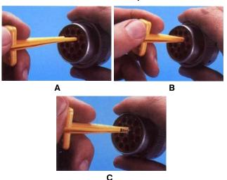
Figure 7-18. HD/HDP Contact Removal
