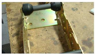
**8.** Remove the snap ring from one side of the bracket.
