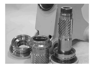
1. Clean all parts in a solvent tank and dry with compressed air prior to inspecting. Carefully inspect all critical areas for any surface finish abnormalities: Seal grooves, bearing grooves, thrust surfaces, rod surface, housing bore and gear teeth.
