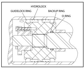
Figure 5-58. Piston Seal Kit Installation
