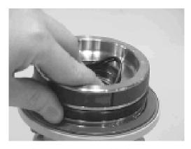
**5.** Install the o-ring (204) and backup ring (207) into the inner seal groove on the end cap (4).
