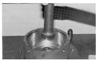
This completes the hub shaft sub-assembly —items (1A) through (1J). If this assembly is not going to be used right away, it should be oiled and covered to help prevent rusting,
