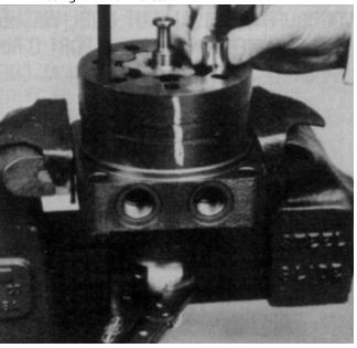
**6.** Remove the two assembled bolts (1) if used to retain stator and wear plate.
