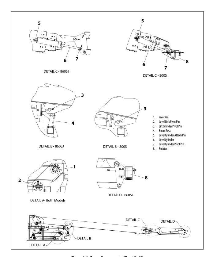
Figure 4-4. Boom Components - Sheet 2 of 2
