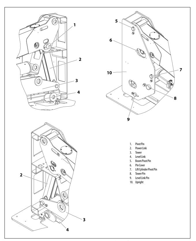
Figure 4-3. Boom Components - Sheet 1 of 2
