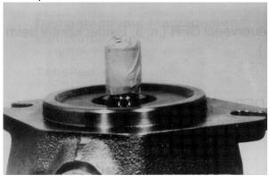
**4.** Assemble the sealing ring, fitting tool holds the correct position of the sealing ring in the pump housing.
