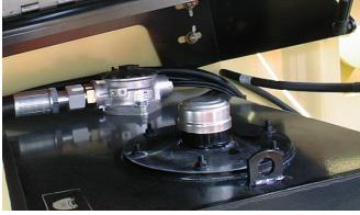
Lube Point(s) - Fill Cap Capacity - 116 liters Tank 124 liters System Lube - HO Interval - Check Level daily; Change every 2 years or 1200 hours of operation.
