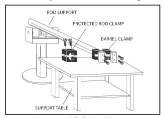
Figure 5-70. Cylinder Barrel Support
