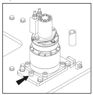
4. Remove the turntable lock pin.
