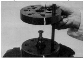
**NOTE:** It may be necessary to turn one alignment stud out of the housing (18) temporarily to assemble rotor set (8) or manifold (7) over the drive link.
