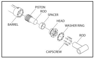
Figure 5-29. Rod Assembly Installation
