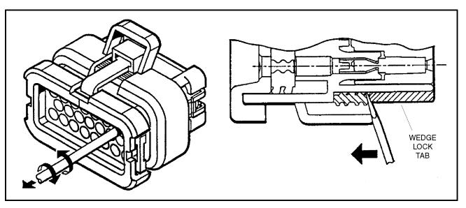
Figure 7-12. Connector Disassembly
