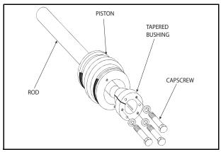
Figure 5-34. Tapered Bushing Removal
