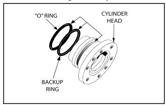
Figure 5-39. Installation of Head Seal Kit
