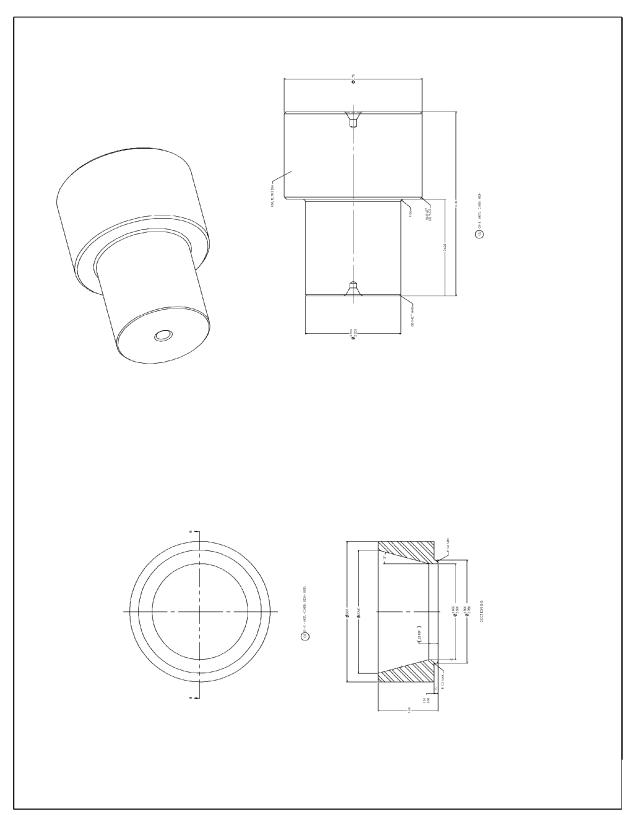
Figure 3-59. Assembly Tools - Brake Retaining Ring Installation
