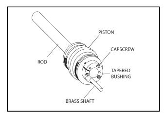
Figure 5-41. Seating the Tapered Bearing
