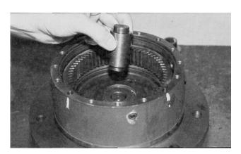
5. Place carrier assembly (3) on a flat surface with the large gears (3F) up and positioned as shown. Find the punch marked tooth on each large gear (3F) and locate at 12 0'clock (straight-up) from each planet pin. Marked tooth will be located just under the carrier (3A) on upper two gears (3F).
