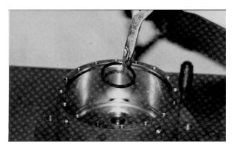
**10.** A soft metal punch should be used to ensure that this retaining ring (1I) is completely seated in the groove of the output shaft (1A).
