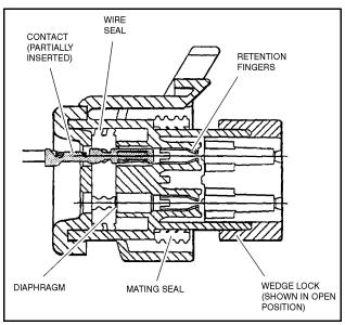
Figure 7-7. Connector Assembly Figure 1
