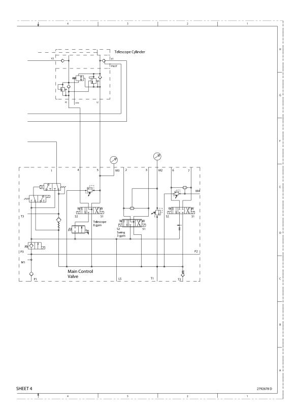
Figure 5-106. Hydraulic Schematic - Sheet 8 of 8
