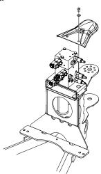
**4.** Remove tag and reconnect the hydraulic lines to the platform control valve.
