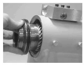
**8.** Insert the piston (3) into the housing (1) as shown, until the outer piston seal (202) is touching inside the housing bore.
