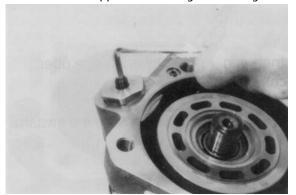
**10.** Disassemble the rotary group in horizontal position.
