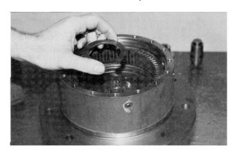
**3.** Place o-ring (5) into hub counterbore. Use petroleum jelly to hold o-ring in place. Also at this time locate and mark the 4 counter beamed holes in the face of the hub (1G). This is for identification later in the assembly.
