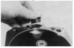
**14.** Disassemble the control plate while moving the swash-plate.
