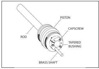
Figure 5-26. Seating the Tapered Bearing
