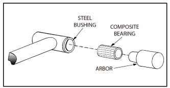
Figure 5-50. Composite Bearing Installation
