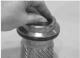
Beginning with the inner seal (200) insert one end of b/u ring in the lower groove and feed the rest in using a circular motion. Make sure the wedged ends overlap correctly. Repeat this step for the outer seal (202).
