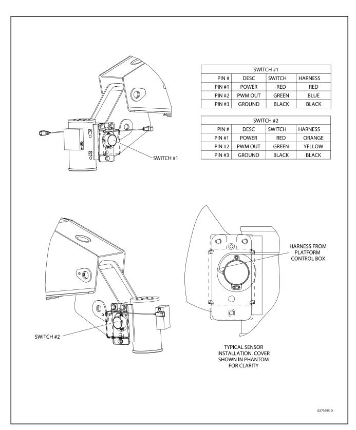
Figure 4-21. Level Switches - 800S
