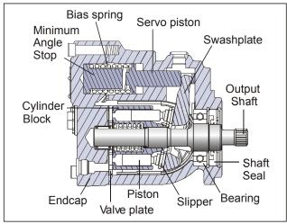
Figure 3-15. Drive Motor Cross Section
