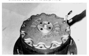
**24.** Install bolts (41) in remaining holes. Torque bolts to 47 ft. lbs. (64 Nm).
