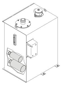
Lube Point(s) - 2 Interval - Every 2 years or 1200 hours of operation, remove and clean at time of hydraulic oil change.
