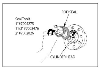
Figure 5-36. Rod Seal Installation
