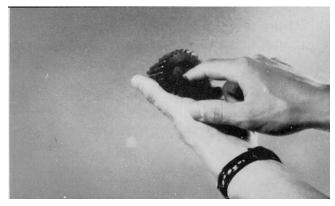
2. Place sixteen needle rollers into cluster gear bore.
