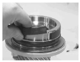
**15.** Remove the wear guides (302) from the end cap (4) and shaft (2).
