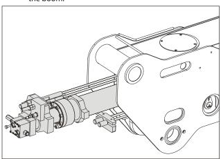
Push the boom fly sections back in to gain access to the boom retraction cable. **10.** Remove the screws securing the sheave guards to the boom mid section and remove the sheave guards.
