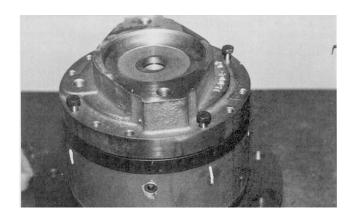
13. Install regular grade 8 bolts (12) into remaining holes.
