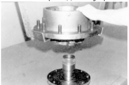
**5.** Place bearing cone (6) over end of spindle and into bearing cup.
