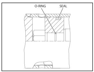
Figure 5-69. Piston Seal Kit Installation
