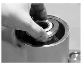
**7.** Remove the stop tube if included. The stop tube is an available option to limit the rotation of the actuator.
