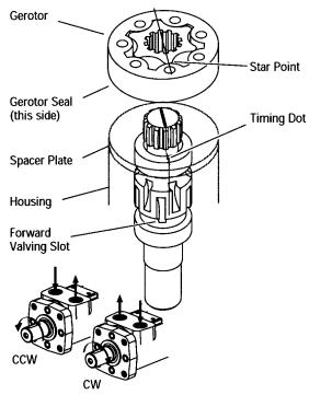
Reverse rotation align any star valley with marked tooth (see figure below).
