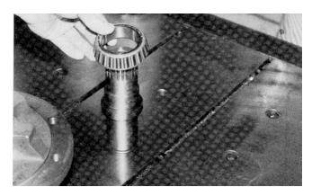
**2.** Press bearing cup (1C) into hub (1G) taking care to insure cup start square with the bore of the hub.
