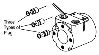
17. A metal plug, with seal, plugs a machining hole in the housing. It is not necessary to remove plug and replace seal unless leakage occurs around plug. To remove plug, insert 5 mm (.187 in.) hex key through port opening and push it out. The 009 plug is not interchangeable with 007 and 008 plugs.
