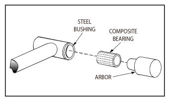
Figure 5-85. Composite Bearing Installation
