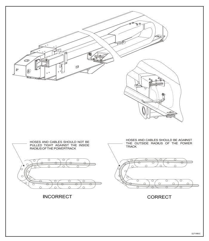
Figure 4-15. Powertrack Installation Main Boom - (Sheet 2 of 2)
