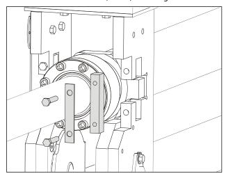
**12.** Using a 3/8 drive extension approximately 4 ft (1.2 m) long, install the bolts and washers securing the cable mount block to the boom fly section. Tape the bolts to the socket at the end of the extension to prevent it from coming out of the socket before it engages the mounting threads.
