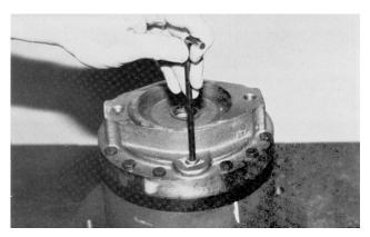
**15.** Torque shoulder bolts (13) to 23-27 ft. lbs. (31-37 Nm) and regular grade 8 bolts (12) to 23-27 ft. lbs. (31-37 Nm).
