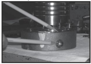
**NOTE:** A polished pattern (not scratches) on the cover from rotation of the commutator (5) is normal. Discoloration would indicate excess fluid temperature, thermal shock, or excess speed and require system investigation for cause and close
