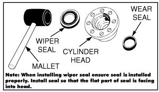
Figure 5-23. Wiper Seal Installation
