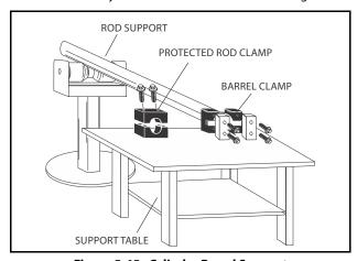
Figure 5-45. Cylinder Barrel Support
