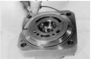
**24.** A usual commercial bearing puller is used to disassemble the external bearing ring of the taper roller bearing inside the port plate. Take care of the surface of the port plate.
