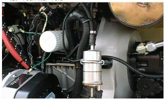
Lube Point(s) - Replaceable Element Interval - Every Year or 1200 hours of operation
