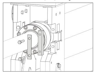
**22.** Using a 3/8 drive extension approximately 4 ft (1.2 m) long, install the bolts and washers securing the cable mount block to the boom fly section. Tape the bolts to the socket at the end of the extension to prevent it from coming out of the socket before it engages the mounting threads.
