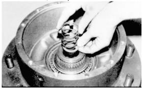
**e.** Install retaining ring into input shaft groove to secure spacers and spring to shaft.
