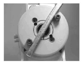
**17.** Tighten the end cap (4). In most cases the original holes for the lock pins will line up.
