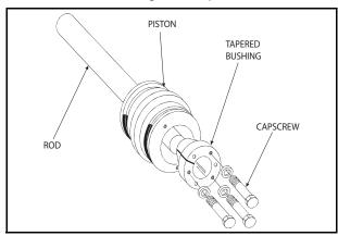
Figure 5-19. Tapered Bushing Removal
