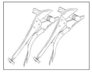
Figure 4-16. Clamping Wire Ropes
