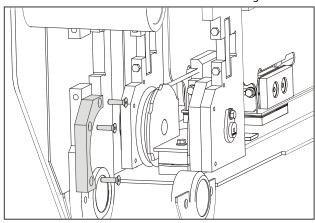
11. Remove the adjusting nuts and lock nuts from the opposite end of the retraction cables at the front of the boom base section. To aid in installing new retraction cables, fasten a length of tie wire as long as the retraction cables to the ends of the cables.
