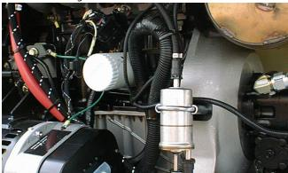
Lube Point(s) - Fill Cap/Spin-on Element
