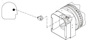
Every 500 hours of service, blow out the inside of the generator. If operating in a hostile environment, clean monthly.
