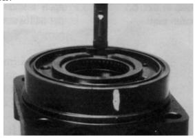
2. The Torqlink™ inner housing bearing/bushing (13) can now be pressed into its counterbore in housing (18) flush to 0.03 in. (.76 mm) below the housing wear plate contact face. Use the opposite end of the bearing mandrel that was used to press in the outer bearing/bushing (19).
