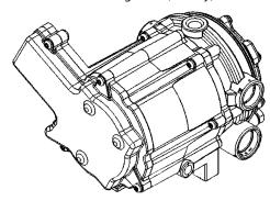
Interval - 3 Months or 150 hours of operation Comments - Drain oil build up. Refer to Draining Oil Build Up From The Propane Regulator
