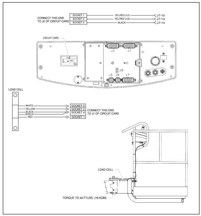
Figure 4-26. Load Sensing Device
