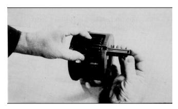
**8.** Drive anti-roll pin flush into carrier hole, thereby locking planet shaft into place.
