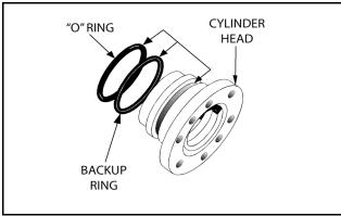
Figure 5-10. Installation of Head Seal Kit
