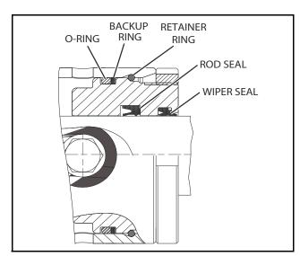
Figure 5-76. Cylinder Head Seal Installation
