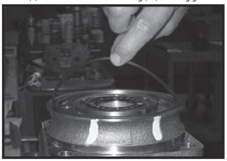
NOTE: One or two alignment studs screwed finger tight into housing (18) bolt holes, approximately 180 degrees apart, will facilitate the assembly and alignment of components as required in the following procedures. The studs can be made by cutting off the heads of either 3/8-24 UNF 2A or 5/16-24 UNF 2A bolts as required that are over 0.5 in.
