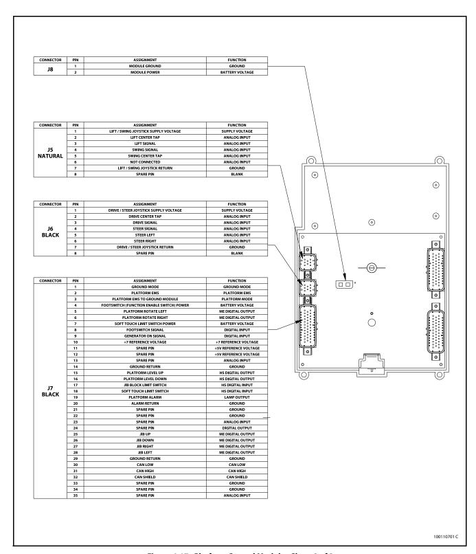
Figure 6-17. Platform Control Module - Sheet 2 of 2
