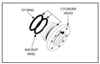
Figure 5-54. Installation of Head Seal Kit
