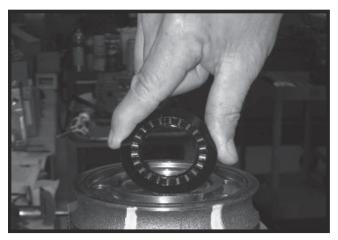
Apply a small amount of clean grease to a new seal ring
