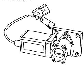
The electronic governor consists of a throttle body, an electronically-actuated throttle plate, and a built-in throttle position (TP) sensor. There are two pigtails that exit the governor body. The 3-wire pigtail connects the TP sensor to the ECM. Refer to "Throttle Position (TP) Sensor" for more information.
