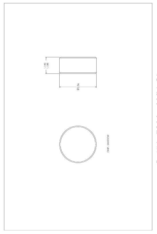
Figure 3-58. Assembly Tools - Spacer - Brake Disc Installation
