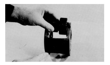
**7.** Line up cluster gear and thrust washer with hole in carrier and slide planet shaft through. Line up chamfered side of hole in planet shaft with pin hole in carrier.
