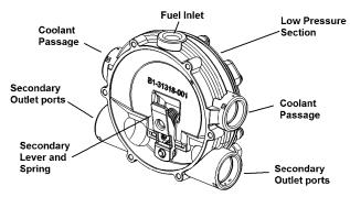
Figure 3-116. Pressure Regulator Section
