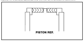
Figure 5-57. Hydrolock Piston Seal Installation
