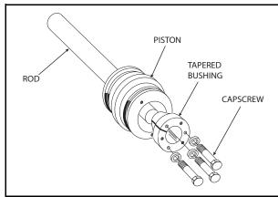
Figure 5-25. Tapered Bushing Installation
