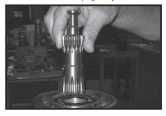
**NOTE:** Use any alignment marks put on the coupling shaft and drive link before disassembly to assemble the drive link splines in their original position in the mating coupling shaft splines.
