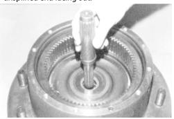
**12.** Place thrust spacer (36) over input shaft (35) with counterbore side facing spindle.
