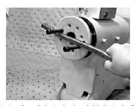
**13.** Install two bolts in the threaded holes in the flange. Using a bar, rotate the shaft in a clockwise direction until the wear guides are seated inside the housing bore.
