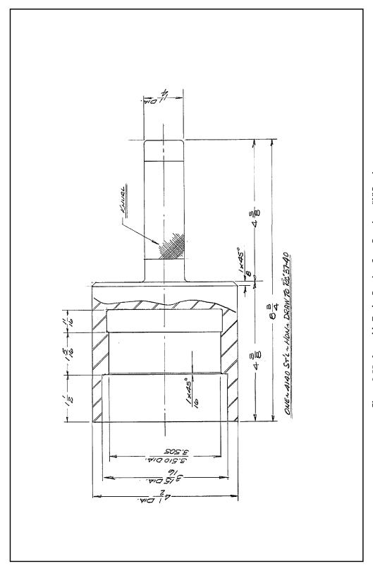
Figure 3-55. Assembly Tools - Bearing Cone Pressing - "A" Bearing
