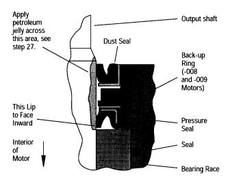
**10.** Before installing flange and seal assembly over shaft, place protective sleeve or bullet over shaft. Then lubricate space between exclusion seal and pressure seal, as well as lips of both seals.
