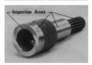
**NOTE:** Minor shaft wear in seal area is permissible. If wear exceeds 0.020 in. (0.51 mm) diametrically, replace coupling shaft.
