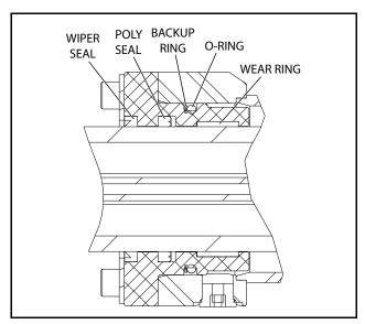
Figure 5-87. Cylinder Head Seal Installation
