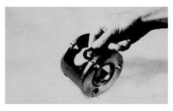
**6.** While keeping thrust washers in place, slide cluster gear into carrier with the larger gear on the side with the small pin hole.
