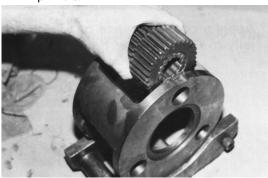
**n.** Line up cluster gear and thrust washers with hole in carrier and slide planet shaft through. Ensure cham-
