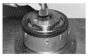
**9.** Thrust washer (10) is installed onto the input gear (8) and should locate on the gear teeth shoulder.
