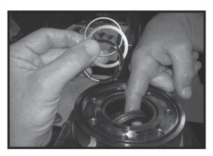
**20.** Remove housing (18) from vise, invert it and remove and discard seal. A blind hole bearing or seal puller is required.
