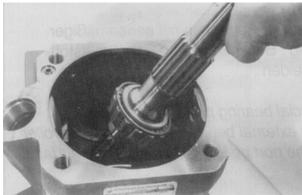
**20.** Disassemble the snap ring.
