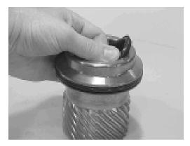
7. Install the inner T-seal (200) into the piston (3) using a circular motion. Install the outer T-seal (202) by stretching it around the groove in a circular motion. Each T-seal has 2 backup rings (see drawing for orientation).
