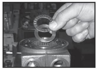
**NOTE:** Torqmotors<sup>™</sup> require one thrust washer (14) with thrust bearing (15).The coupling shaft will be seated directly against the thrust.
