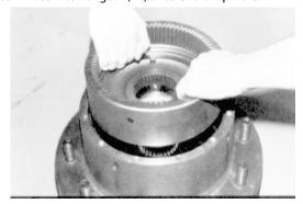
Install thrust washers and thrust bearing (39, 40) on the portion of the spindle which extends into the internal gear.
