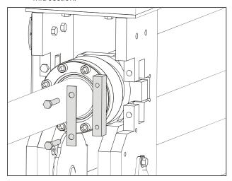
Remove the four bolts, shims, and mounting blocks that secure the telescope cylinder rod to the boom base section.
