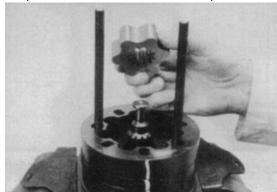
**NOTE:** If the manifold side of the rotor was etched during Torqlink disassembly, this side should be up. If the rotor is not etched and does not have a counterbore, use the drive link spline contact pattern apparent on the rotor splines to determine the rotor side that must be against the wear plate.
