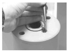
**18.** Place the lock pins (109) provided in the Helac seal kit in the holes with the dimple side up. Then, using a punch, tap the lock pins to the bottom of the hole.
