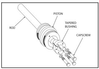
Figure 5-55. Tapered Bushing Installation
