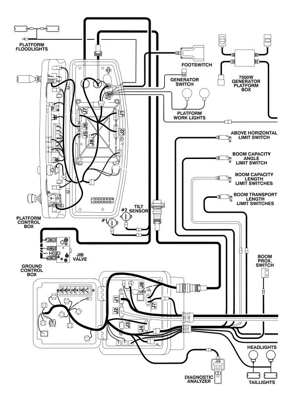
Figure 7-22. Electrical Components Installation (WITHOUT UGM) (SN 0300085332 through 0300140000) - Sheet 1 of 2
