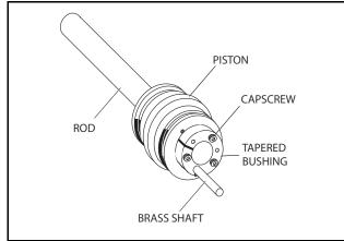
Figure 5-12. Seating the Tapered Bushing
