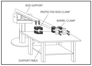
Figure 5-80. Cylinder Barrel Support
