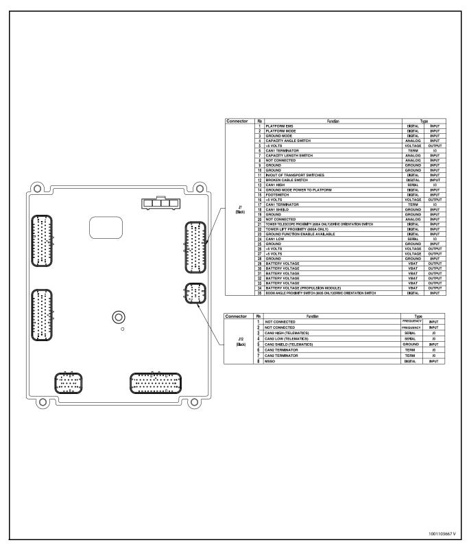
Figure 6-14. Ground Control Module - Sheet 2 of 3
