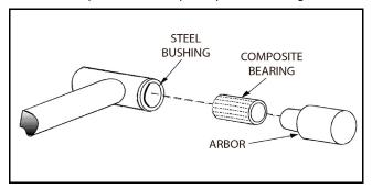
Figure 5-35. Composite Bearing Installation
