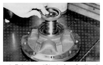
**6.** The bearing cone (1F) is an interference fit and has to be pressed or tapped on.
