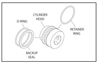
Figure 5-78. Installation of Head Seal Kit
