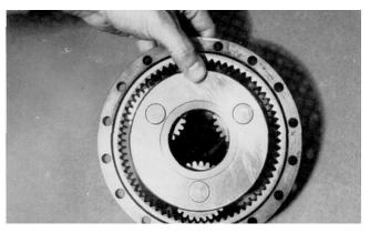
7. While holding ring gear (4) and cluster gears (3F) in mesh, place small side of cluster gears (3F) into mesh with the internal gear (2) and input gear (13). On the ring gear locate the hole marked "x" over one of the marked counterbore holes (step 3) in hub (1G).
