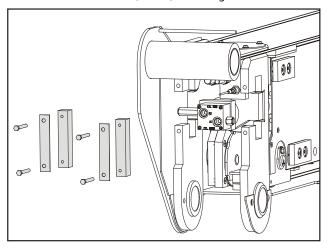
**21.** Apply JLG Threadlocker P/N 0100011 to the bolts and fasten the telescope cylinder barrel to the boom mid section with the bolts, shims, mounting blocks.
