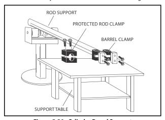
Figure 5-30. Cylinder Barrel Support
