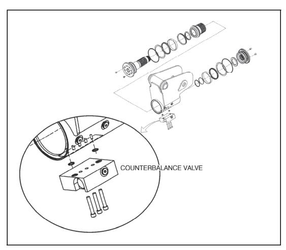
Figure 4-25. Rotator Counterbalance Valve
