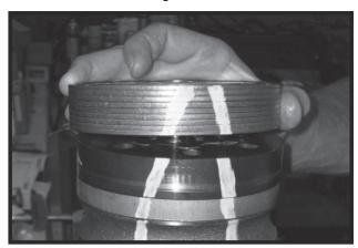
**16.** Apply grease to a new seal ring (4) and insert it in the seal ring groove exposed on the manifold.
