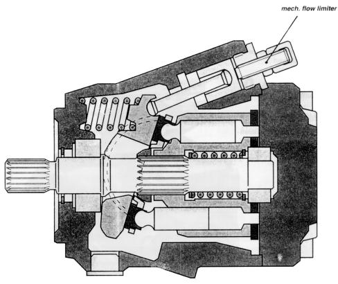
Figure 3-11. Drive Motor Cutaway
