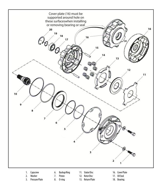
Figure 3-9. Drive Brake, 2WD - Mico (Prior to SN 0300083331)
