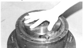
**20.** Install thrust washers and thrust bearing (39, 40) into carrier counterbore.
