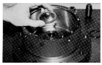
**9.** Retaining ring (1I) installed into groove provided in the output shaft (1A). This retaining ring (1I) should never be reused in a repair or rebuild.
