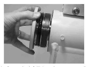
**10.** Remove the shaft (2). It may be necessary to strike the threaded end of the shaft with a rubber mallet.
