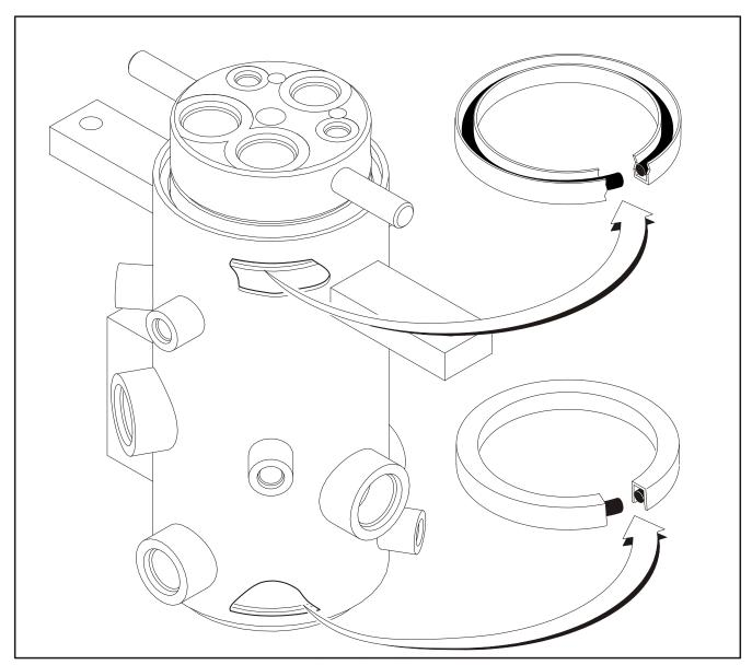
Figure 3-81. Rotary Coupling Seal Installation (Prior to SN 0300083331)
