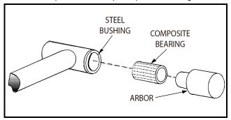
Figure 5-6. Composite Bearing Installation
