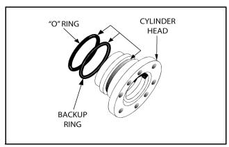
Figure 5-24. Installation of Head Seal Kit
