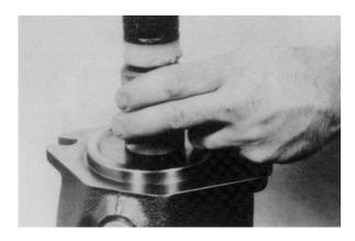
NOTE: This description shows how to change the drive shaft sealing ring but isn't the way of serial assembly. the sealing ring is assembled together with the taper roller bearing from inside the pump housing normally to get a secure condition. If you decide to repair the pump in the shown way be very careful while handling so that the drive shaft will not be damaged during disassembly of the shaft sealing ring.
