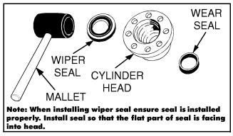
Figure 5-88. Wiper Seal Installation
