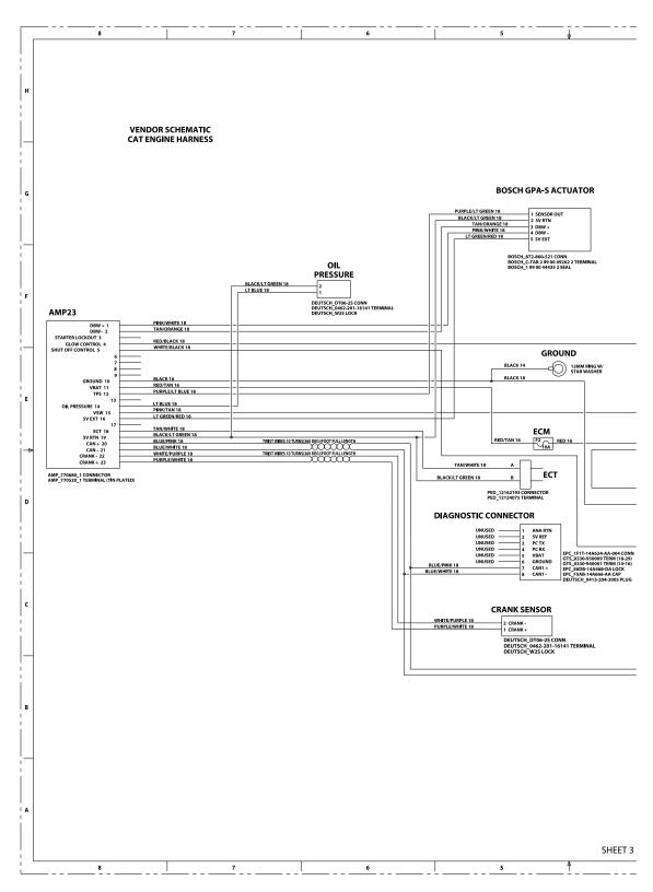
Figure 7-37. Electrical Schematics Caterpillar, Deutz EMR2 and GM (SN 0300139080 through 0300161729 and SN B300000100 through B300000639) - Sheet 5 of 10
