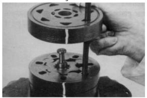
**16.** Apply grease to a new seal ring (4) and insert it in the seal ring groove exposed on the manifold.
