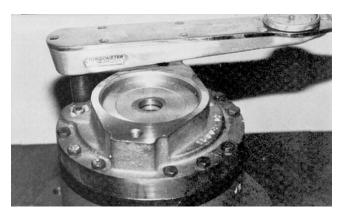
This completes the assembly. The unit must be filled one-half full of EP 90 lubricant before operation if the unit is mounted horizontally, and completely filled if mounted vertically. In vertical mounting application case oil circulation is recommended.
