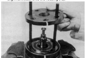
**12.** Apply a small amount of clean grease to a new seal ring (4) and assemble it into the seal ring groove on the wear plate side of the rotor set stator (8B).
