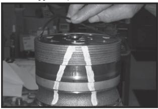
**17.** Assemble the commutator ring (6) over alignment studs onto the manifold.
