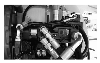
**b.** Next, using the 6 mm wrench adjust the main adjustment clockwise to increase or counter-clockwise to decrease. The pressure should read between 400-440 psi (27.5 to 30 Bar).
