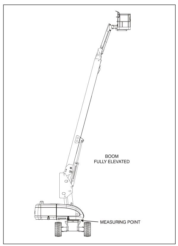
Figure 3-75. Swing Bearing Tolerance Boom Placement. (Sheet 1 of 2)
