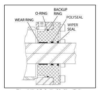
Figure 5-52. Cylinder Head Seal Installation
