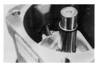
**3.** Pumps clockwise driven must have a position of the valve plate 4° out of center in the same direction decentered like drive direction.
