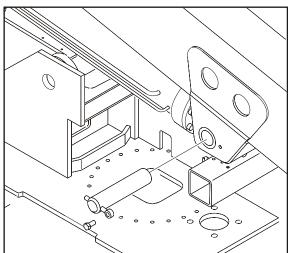
Remove the bolt and keeper pin securing the lower lift cylinder pivot pin and remove the pivot pin.
