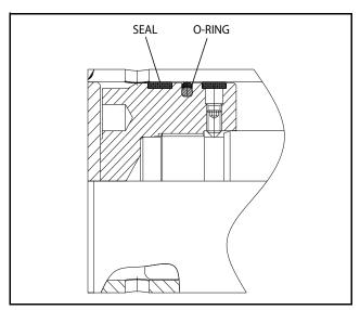
Figure 5-79. Piston Seal Kit Installation (Prior to SN 0300142664)
