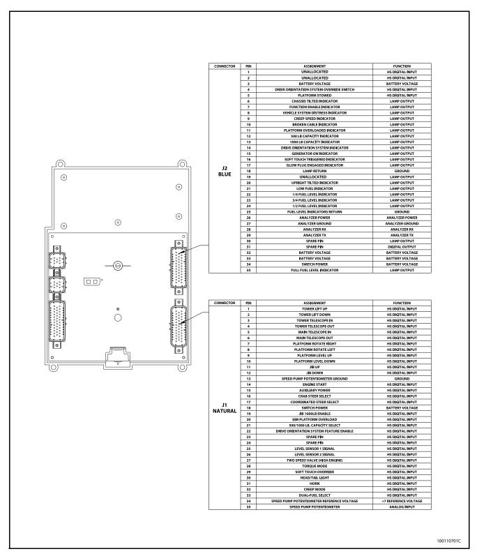
Figure 6-16. Platform Control Module - Sheet 1 of 2
