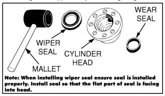
Figure 5-38. Wiper Seal Installation
