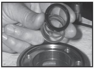
**19.** Remove seal (16), backup ring (17) and backup washer (25) from large frame, housing by working them around unseated thrust washers (14) and thrust bearing (15) and out of the housing. Discard seal and washers.
