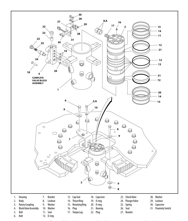
Figure 3-88. Rotary Coupling Installation (SN 0300083331 through 0300182743, B300000100 through B300001091)
