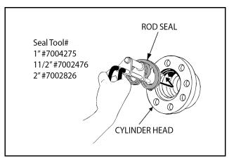
Figure 5-75. Rod Seal Installation
