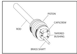
Figure 5-56. Seating the Tapered Bearing
