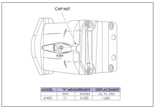
Figure 3-14. Drive Motor Adjustment
