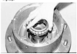
**6.** Place bearing shim (8) over end of spindle and against bearing cone.
