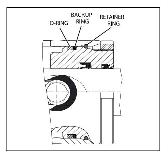
Figure 5-66. Cylinder Head Seal Installation
