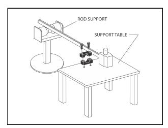
Figure 5-72. Cylinder Rod Support
