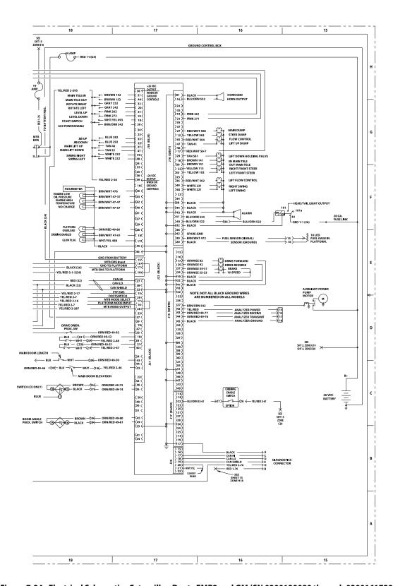
Figure 7-34. Electrical Schematics Caterpillar, Deutz EMR2 and GM (SN 0300139080 through 0300161729 and SN B300000100 through B300000639) - Sheet 2 of 10
