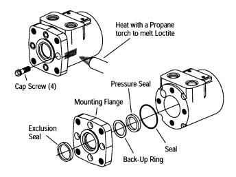
15. Carefully remove flange from housing.
