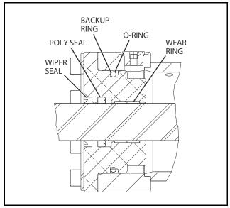
Figure 5-8. Cylinder Head Seal Installation
