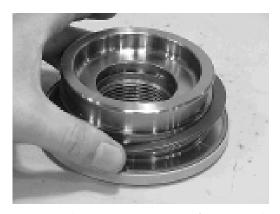
**17.** Remove the thrust washers (304), from the end cap (4) and shaft (2).
