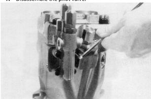
**2.** Mark the position of the port plate and remove the socket screw of the port plate.
