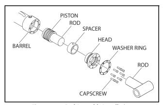
Figure 5-93. Rod Assembly Installation
