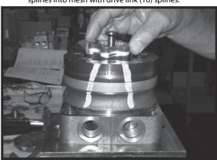
**NOTE:** If the manifold side of the rotor was etched during Torqmotor disassembly, this side should be up. If the rotor is not etched and does not have a counterbore, use the drive link spline contact pattern apparent on the rotor splines to determine the rotor side that must be against the wear plate.
