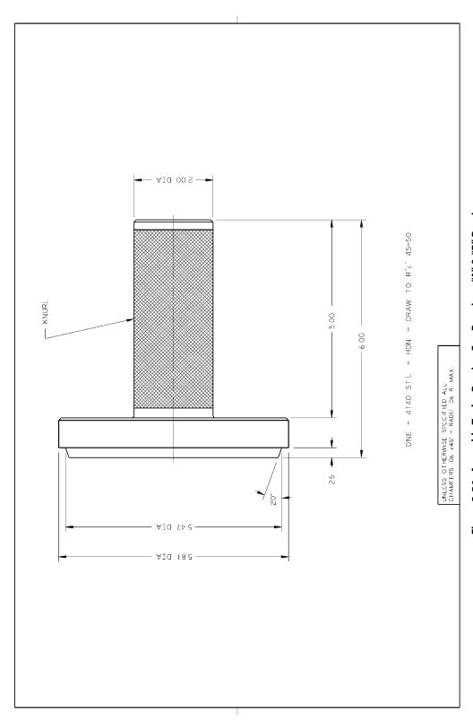
Figure 3-56. Assembly Tools - Bearing Cup Pressing - "A" & "B" Bearings
