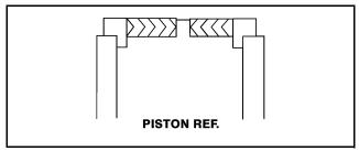
Figure 5-42. Hydrolock Piston Seal Installation
