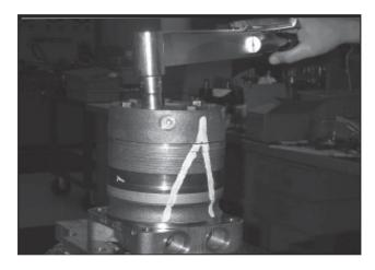
**9.** Remove the five, six, or seven special ring head bolts (1) using an appropriate 1/2 or 9/16 in. size socket. Inspect bolts for damaged threads, or sealing rings, under the bolt head. Replace damaged bolts.
