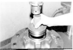
2. Place bearing cone (4) into bearing cup (3) in small end of hub.
