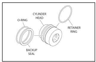
Figure 5-68. Installation of Head Seal Kit
