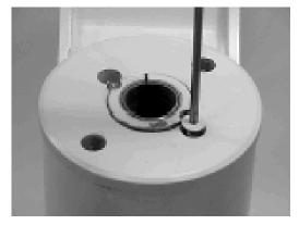
Remove the capscrews (113) over end caplock pins (109).
