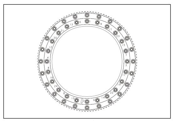
**NOTE:** Swing Bearing Torque Sequence is typical for both inner and outer races.
