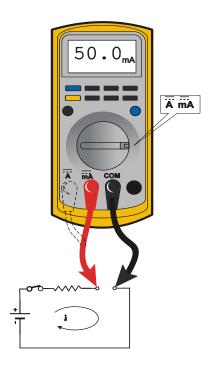
Figure 7-4. Current Measurement (DC)
