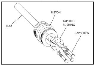
Figure 5-5. Tapered Bushing Removal
