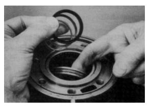
**19.** Remove housing (18) from vise, invert it and remove and discard seal (20). A blind hole bearing or seal puller is required.
