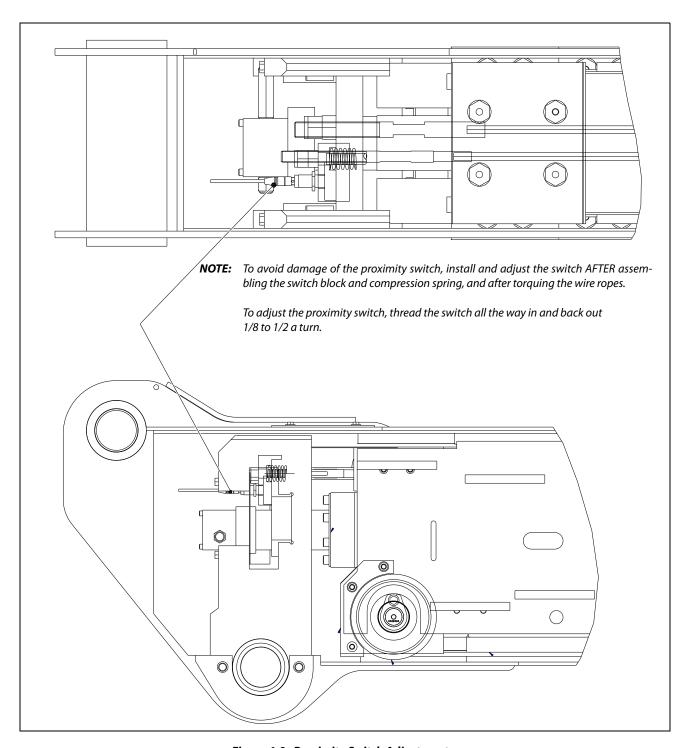
Figure 4-8. Proximity Switch Adjustment
