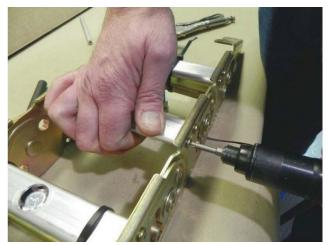
5. Remove the snap rings and pins.
