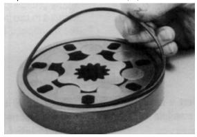
**13.** Install the assembled rotor set (8) onto wear plate (9) with rotor (8A) counterbore and seal ring side down and the splines into mesh with the drive link splines.
