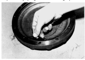
22. Place cover assembly over ring gear with oil level check plug in cover located approximately 90 degrees from oil fill plug in hub.
