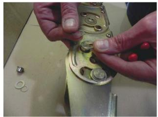
**6.** Remove the screws from the bar. Remove the snap ring and pin.
