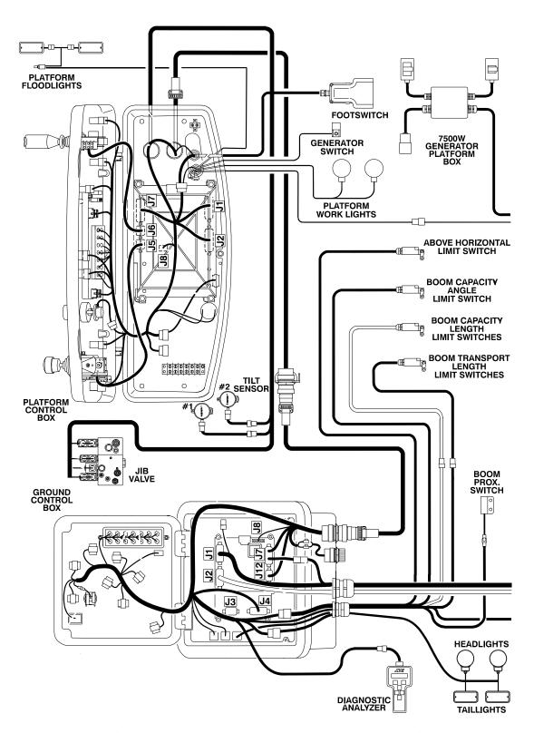
Figure 7-25. Electrical Components Installation (WITH UGM) (SN 0300140000 through 0300182743 and SN B300000100 through B300001091) - Sheet 1 of 2
