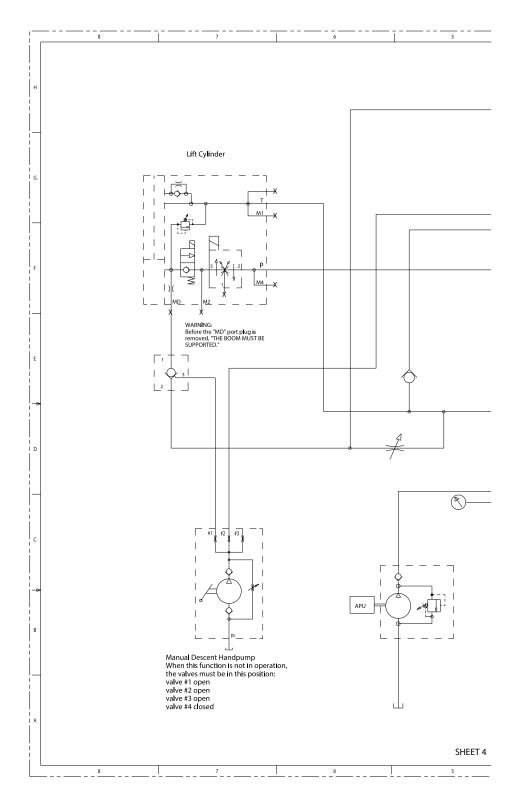
Figure 5-105. Hydraulic Schematic - Sheet 7 of 8
