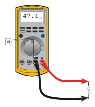
Figure 7-2. Resistance Measurement
