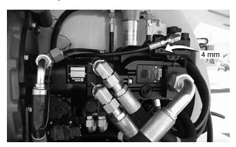
b. Next, using the 6 mm wrench adjust the main adjustment clockwise to increase or counter-clockwise to decrease. This adjustment will be re-set at the end of this procedure to 2500 psi (172 Bar). This is the <u>maximum</u> relief pressure for all functions governed by this pump.
