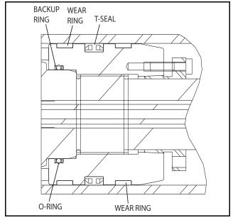
Figure 5-92. Piston Seal Kit Installation
