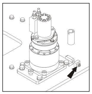
**9.** Torque the capscrews shown in step 5 to 340 footpounds (569 Nm).
