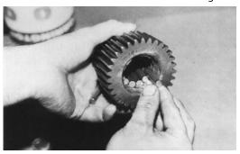
j. Place spacer into opposite side of cluster gear and against needle rollers.
