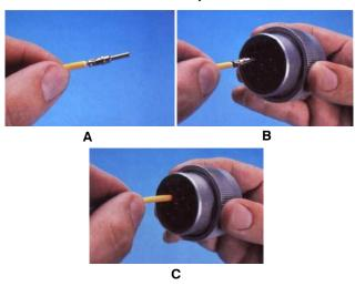
Figure 7-16. HD/HDP Contact Installation
