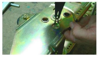
**9.** Remove the snap ring from the other side of the bracket.
