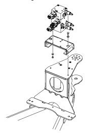
**3.** Install cover onto the platform support securing the hardware.
