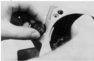
**15.** The swashplate must be lifted a little bit to disassemble the piston rod.
