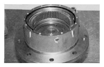
**4.** Thrust spacer (9) is installed into the bore of the output shaft (1A). This should be a slip fit and thrust spaces should rotate in this location.
