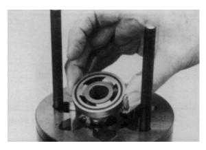
**19.** If shuttle valve components items #21, were removed from the end cover (2) turn a plug (21), loosely into one end of the valve cavity in the end cover. A 3/16 in. Allen wrench is required.
