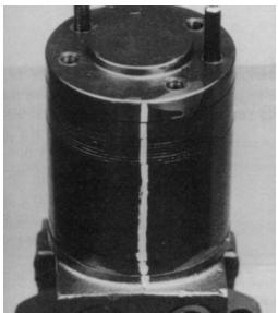
**NOTE:** If the end cover has a valve (24) or has five bolt holes, use the line you previously scribed on the cover to radially align the end cover into its original position.
