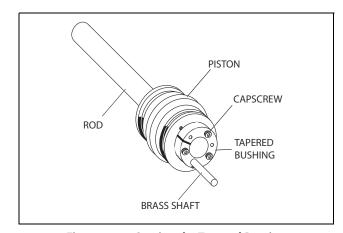
Figure 5-91. Seating the Tapered Bearing
