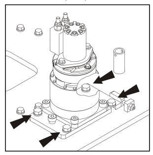
**6.** Tighten the setscrew (shown below) until the pinion is completely snug against the shim and bearing and then back off the setscrew.
