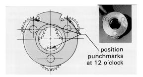
**6.** With shoulder side of ring gear (4) facing down, place ring gear over (into mesh with) large gears. Be sure that punch marks remain in correct location during ring gear installation. The side of the ring gear with an X stamped on it should be up.
