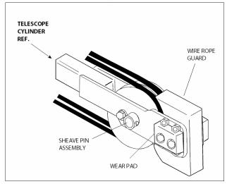
Figure 4-5. Disassembly of Sheave Assembly
