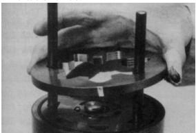
**18.** Assemble a new seal ring (3) flat side up, into commutator (5) and assemble commutator over the end of drive link (10) onto manifold (7) with seal ring side up.
