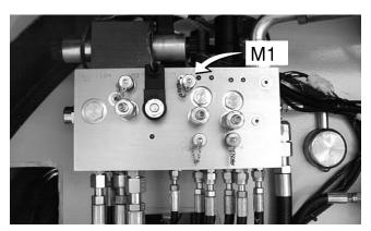
2. Start the engine from the ground control. The gauge should read between 400-440 psi (27.5 to 30 Bar). To make an adjustment to this pressure, go to the engine compartment, locate the function pump.
