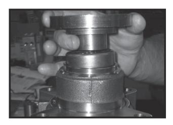
**NOTE:** Bearing mandrel must be pressed against the lettered end of bearing shell. Take care that the housing bore is square with the press base and the bearing/bushing is not cocked when pressing a bearing/bushing into the housing.
