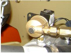
Interval - 3 Months or 150 hours of operation Comments - Replace filter. Refer to Propane Fuel Filter Replacement
