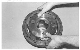
**17.** While holding ring gear, input gear, and cluster gears in mesh, place small side of cluster gears into mesh with
