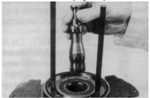
**NOTE:** Use any alignment marks put on the coupling shaft and drive link before disassembly to assemble the drive link splines in their original position in the mating coupling shaft splines.
