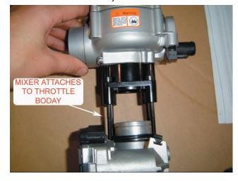
Place gasket on intake manifold and attach mixer/throttle assembly to manifold.
