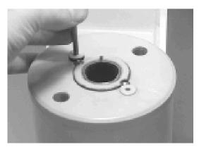
**19.** Insert the set screws (113) over the lock pins. Tighten them to 25 in. lbs. (2.825 Nm).
