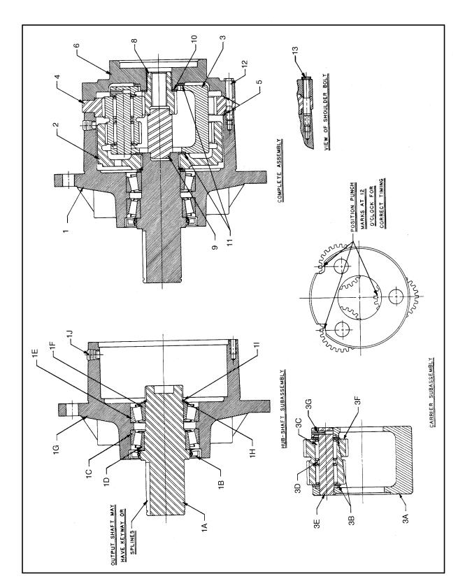
Figure 3-61. Swing Drive (Prior to SN 0300066417)
