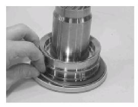
3. Install the wiper seal (304.1/green o-ring) into it's groove on the shaft (2) and end cap (4) around the outside edge of the thrust washer (304).
