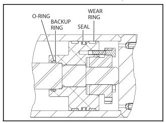
Figure 5-13. Piston Seal Kit Installation
