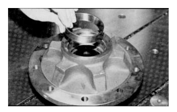
**3.** Invert hub (1G) and press bearing cup (1E) into inter counterbore of hub (1G).
