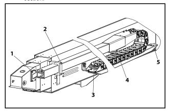
Figure 4-13. Main Boom Powertrack Components
