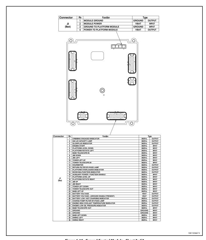
Figure 6-15. Ground Control Module - Sheet 3 of 3
