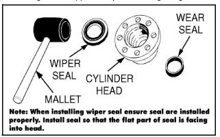
Figure 5-9. Wiper Seal Installation
