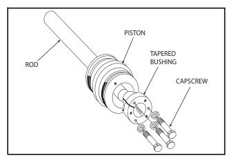
Figure 5-90. Tapered Bushing Installation
