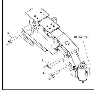
Figure 4-12. Reassembly of Components-Rotator and Leveling Cylinder
