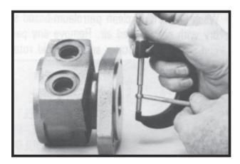
**NOTE:** The depth or location of bearing/bushing (13) in relation to the housing wear plate surface and the depth or location of bearing/bushing (19) in relation to the beginning of bearing/bushing counterbore should be measured and noted before removing the bearings/ bushings. This will facilitate the correct reassembly of new bearings/bushings.
