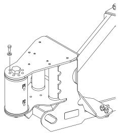
**4.** Torque the nut on the rotator center bolt to 586 ft. lbs. (795 Nm). Torque the retaining bolts to 40 ft. lbs. (55 Nm).
