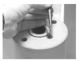
19. Remove the piston O.D. seal (202).
