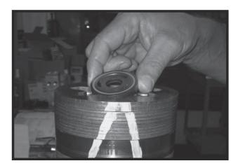
**19.** Assemble a new seal ring (4) into end cover (2) and assemble end cover over the alignment studs and onto the commutator set. If the end cover has only 5 bolt holes be sure the cover holes are aligned with the 5 threaded holes in housing (18). The correct 5 bolt end cover bolt hole relationship to housing port bosses.
