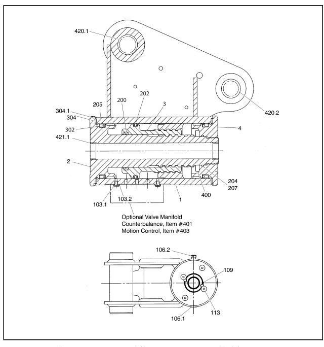
1. 109. Lock Pin 302. Wear Guide Housing 304. Thrust Washer 2. Shaft 113. Cap Screw 200. T-Seal 304.1. WiperSeal 3. Piston Sleeve End Cap 400. Stop Tube (Optional) 4. 202. T-Seal 103.1. Screw (Optional) 204. 0-ring 420.1. Bushing 103.2. Washer (Optional) 205. Cup Seal 420.2. Bushing (Optional) 106.1. Port Plug 207. Backup Ring 421.1. Bushing (Optional) 106.2. Port Plug
