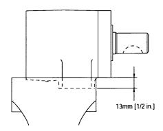
11. After removing bullet, clamp motor in vise as shown above. Make sure shaft cannot fall out. Install dry screws and alternately torque them immediately to 250 in. lbs. (28 Nm). If you use primer, allow to cure 10 to 15 minutes. Without primer, allow 6 hours curing time before subjecting to high torque reversals. On all other applications, you can run motor immediately.
