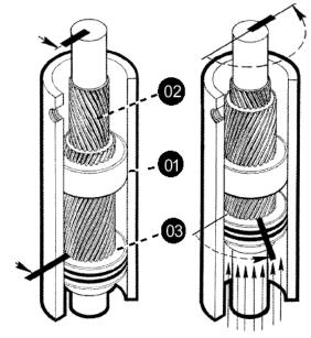
**NOTE:** Bars indicate starting positions of piston and shaft. Arrows indicate direction they will rotate. The housing with integral ring gear remains stationary.
