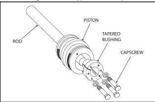
Figure 5-40. Tapered Bushing Installation
