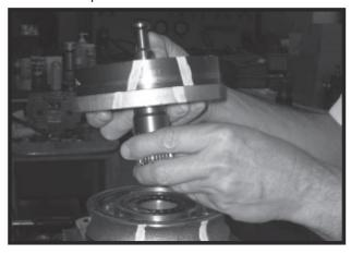
**NOTE:** Series TG and TH may have a rotor set with two stator halves (8B & 8D) with a seal ring (4) between them and two sets of seven vanes (8C & 8E). Discard seal ring only if stator halves become disassembled during the service procedures.
