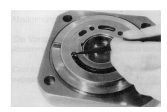
**4.** Pumps anti-clockwise driven must have a position of the valve plate 4° decentered in counter-clockwise position.
