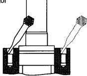
9. Apply 3 or 4 drops of Loctite sealant at top of threads for each of the four holes in housing. Do not allow parts with Loctite applied to come on contact with metal parts other than those for assembly. Wipe off excess Loctite from housing face, using a non petroleum base solvent.
