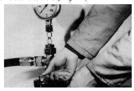
FR: If swivel angle is in the mid position adjust differential pressure 14 bar adjustable orifice is partly closed).
