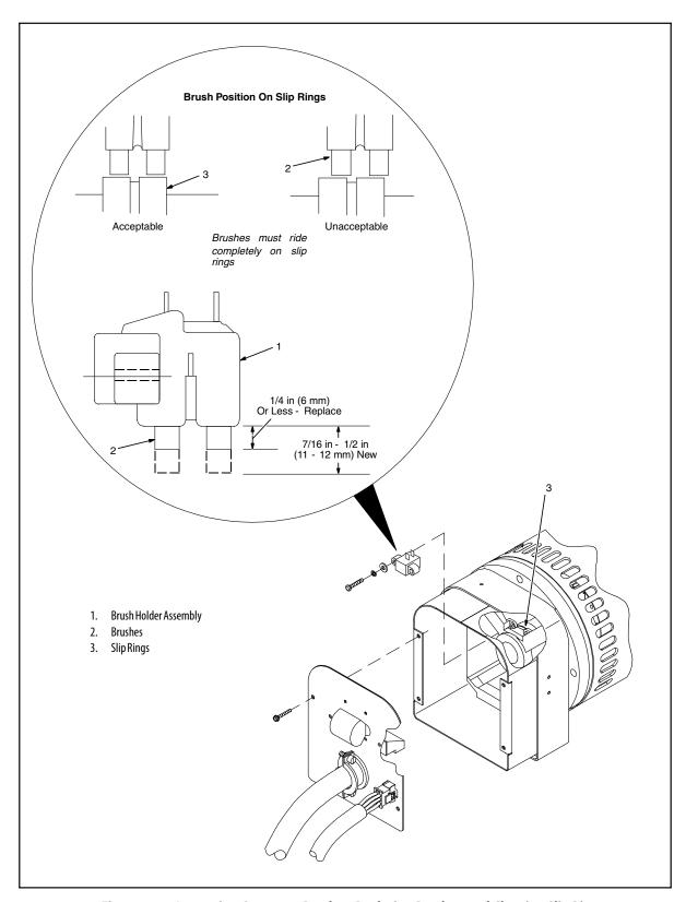
Figure 3-89. Inspecting Generator Brushes, Replacing Brushes, and Cleaning Slip Rings
