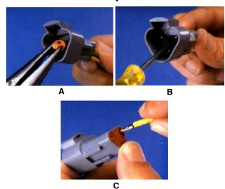
Figure 7-15. DT/DTP Contact Removal
