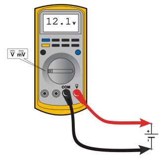
Figure 7-1. Voltage Measurement (DC)
