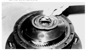
**21.** Place o-ring (22) into cover assembly counterbore. Use petroleum jelly or grease to hold o-ring in place.
