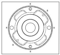
**NOTE:** Start with the red springs and space them as evenly as possible throughout the spring retainer, then take the first blue spring and put it in any one of the remaining empty holes, second blue spring should be placed as directly across from the first blue spring as possible.
