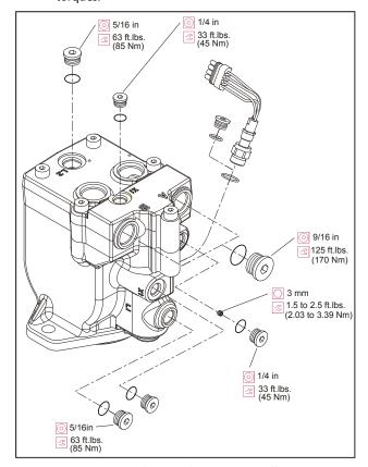
Figure 3-36. Plugs and Fittings Installation
