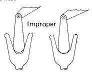
Observe the groove so that it may be clearly seen whether the contour of the gauge matches the contour of the bottom of the groove.
