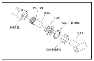
Figure 5-14. Rod Assembly Installation
