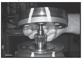
NOTE: The rotor set (8) components may become disassembled during service procedures. Marking the surface of the rotor and stator that is facing UP, with etching ink or grease pencil before removal from Torqmotor™ will ensure correct reassembly of rotor into stator and rotor set intoTorqmotor™.Marking all rotor components and mating spline components for exact repositioning at assembly will ensure maximum wear life and performance of rotor set and Torqmotor™.
