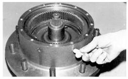
**14.** Place o-ring (22) into hub counterbore. Use petroleum or grease to hold o-ring in place. Slight stretching of o-ring may be necessary to insure proper seating.
