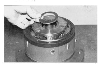
**11.** Place o-ring (5) into cover (6) counterbore. Use petroleum jelly to hold o-ring in place.
