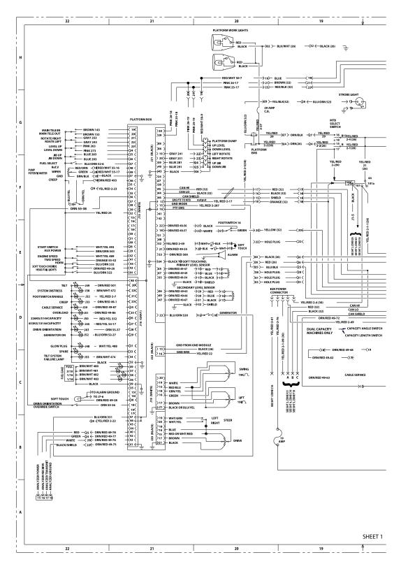
Figure 7-33. Electrical Schematics Caterpillar, Deutz EMR2 and GM (SN 0300139080 through 0300161729 and SN B300000100 through B300000639)- Sheet 1 of 10
