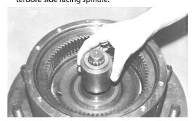
**13.** Locate the four counter reamed holes in the face of the hub, mark them for later identification.
