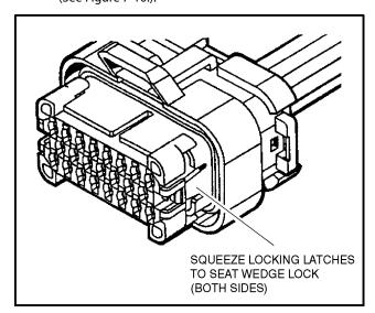
Figure 7-10. Connector Assembly Figure 3
