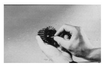
**3.** Place spacer washer into opposite side of cluster gear and against needle rollers.
