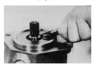
**6.** Assemble the snap ring in the correct position.
