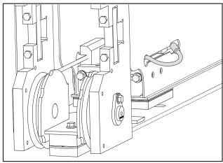
**4.** Install the sheave guards and secure them in place with the retaining screws.
