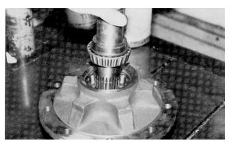
5. The shaft seal (1B) is installed over the output shaft (1A) and into the counterbore of the hub (1G). Care should be taken to insure the seal (1B) is being correctly installed (smooth face up and located just flush with the counterbore face).
