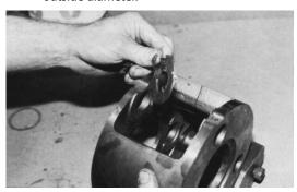
m. While keeping thrust washers in place, slide cluster gear into carrier with larger gear on side with small pin hole.
