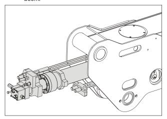
**10.** Apply JLG Threadlocker P/N 0100011 to the bolts and fasten the telescope cylinder rod to the boom base section with the bolts, shims, mounting blocks.
