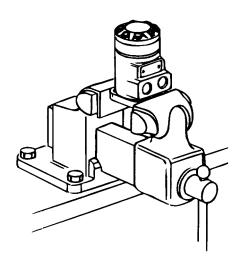
1. Place motor in vice and clamp across edge of flange with output shaft down. When clamping, use protective device on vice such as special soft jaws, pieces of hard rubber or board.
