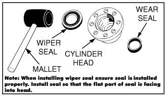
Figure 5-53. Wiper Seal Installation
