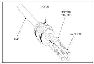
Figure 5-84. Tapered Bushing Removal
