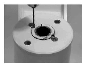
Using a 1/8" (3.18mm) drill bit, drill a hole in the center of each lock pin to a depth of approximately 3/ 16" (4.76mm).
