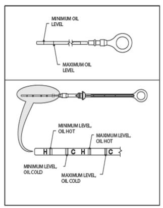
Figure 1-2. Deutz Engine Dipstick
