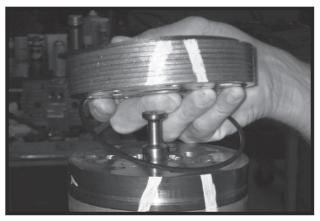
**NOTE:** The manifold is constructed of plates bonded together to form an integral component not subject to further disassembly for service. Compare configuration of both sides oft hem an if old to ensure that same surface is reassembled against the rotor set.
