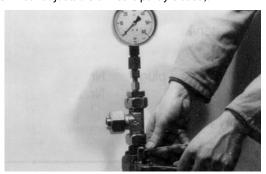
Mechanical flow limiter: While screwing in the threaded pin you will be able to reduce the flow from Vg max to 50% of Vg max.
