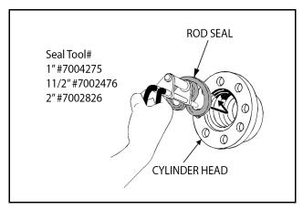
Figure 5-51. Rod Seal Installation
