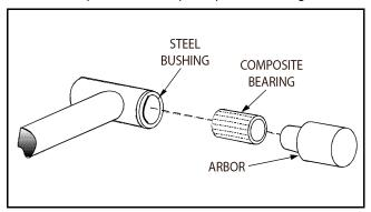
Figure 5-20. Composite Bearing Installation
