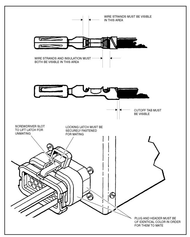
Figure 7-13. Connector Installation
