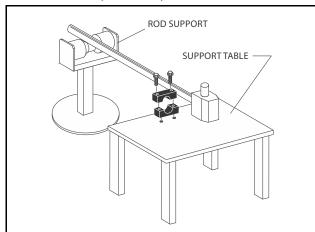
Figure 5-17. Cylinder Rod Support
