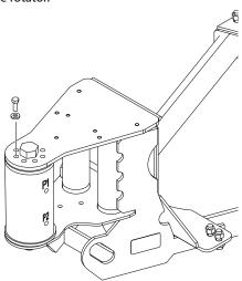
**5.** Using a suitable brass drift and hammer, remove the rotator center bolt, then remove the support from the rotator.
