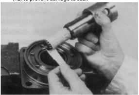
**8.** Be sure that a generous amount of clean corrosion resistant grease has been applied to the lower (outer) housing bearing/bushing (19). Install the coupling shaft (12) into housing (18), seating it against the thrust bearing (15) in the housings.
