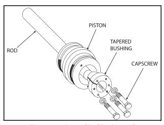
Figure 5-49. Tapered Bushing Removal
