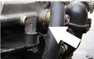
**NOTE:** Have a small container ready to collect oil that will drain freely from the regulator at this point.
