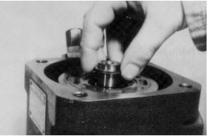
7. Unscrew the cap nut and remove it.
