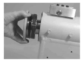
**11.** Install the shaft (2) into the piston (3). Be careful not to damage the seals. Do not engage the piston gear teeth yet.
