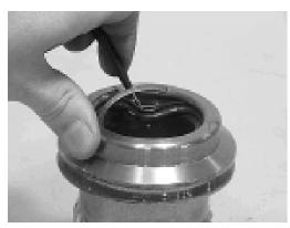
**20.** Remove the piston I.D. seal (200). You may now proceed to the inspection process.
