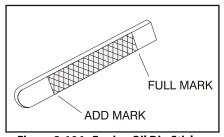
Figure 3-104. Engine Oil Dip Stick
