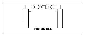
Figure 5-27. Hydrolock Piston Seal Installation
