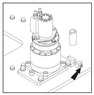
**7.** Apply JLG Threadlocker P/N 0100019 to the setscrew and torque to 50 ft.lbs. (68 Nm).
