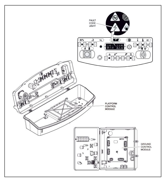
Figure 6-11. Fault Code Light and module Location
