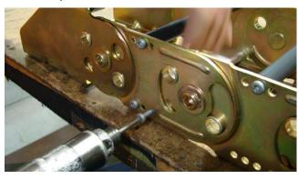
**4.** Pull up on the loose side of the round bar to allow the poly roller to slide off.
