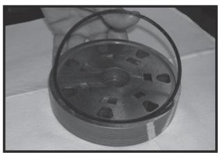
**NOTE:** The manifold (7) is made up of several plates bonded together permanently to form an integral component. The manifold surface that must contact the rotor set has it's series of irregular shaped cavities on the largest circumference or circle around the inside diameter. The polished impression left on the manifold by the rotor set is another indication of which surface must contact the rotor set.
