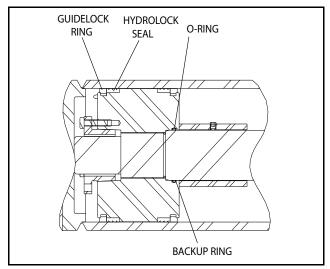
Figure 5-43. Piston Seal Kit Installation
