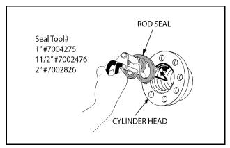
Figure 5-21. Rod Seal Installation
