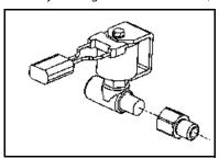
Figure 3-105. Electric Fuel Lock Off
