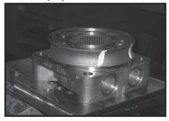
5. On the Torqmotor™ assemble a new backup washer (17) and new seal (16) with the seal lip facing toward the inside of Torqmotor™, into their respective counterbores in housing (18) if they were not assembled in procedure 2
