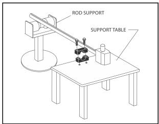
Figure 5-3. Cylinder Rod Support
