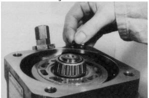
**5.** Disassemble the taper roller bearing (near by port plate).
