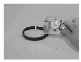
**3.** Inspect the wear guide condition and measure thickness (not less than 0.123" or 3.12 mm).
