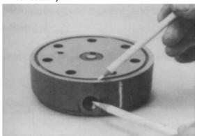
**NOTE:** A polished pattern (not scratches) on the cover from rotation of the commutator (5) is normal. Discoloration would indicate excess fluid temperature, thermal shock, or excess speed and require system investigation for cause and close inspection of end cover, commutator, manifold, and rotor set.
