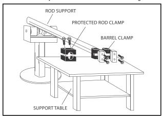
Figure 5-15. Cylinder Barrel Support
