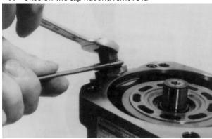
**8.** Loosen the fixing nut of the stopper max flow and disassemble it.
