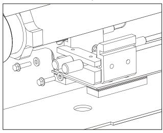
Remove the four bolts, shims, and attachment blocks that secure the telescope cylinder barrel to the boom mid section.
