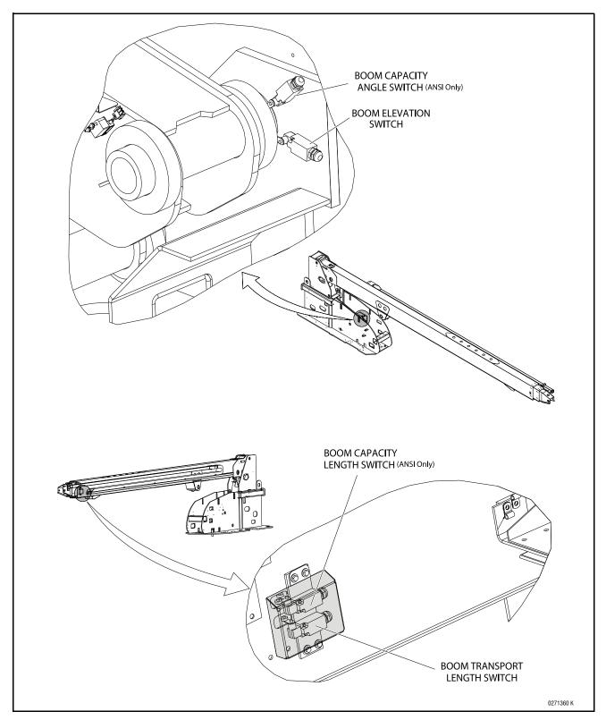
Figure 4-18. Elevation, Dual Capacity and Transport Switch Installation - 800S
