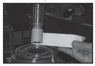
**8.** Be sure that a generous amount of clean corrosion resistant grease has been applied to the lower (outer) housing bearing/bushing (19). Install the coupling shaft (12) into housing (18), seating it against the thrust bearing (15) in the housings.
