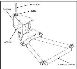
Figure 4-10. Location of Components Platform Support
