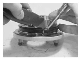
**16.** To remove the main pressure seals (205), it is easiest to cut them using a sharp razor blade being careful not to damage the seal groove.
