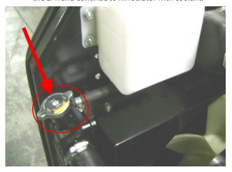
3. With the radiator cap still removed, start the engine and run until the thermostat opens. The thermostat opens at 170° F (77° C), which can be checked using the JLG handheld analyzer.
