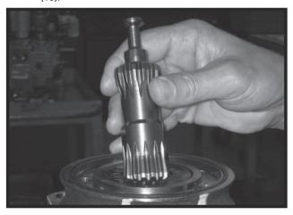
**13.** Remove thrust bearing (11) from top of coupling shaft (12). Inspect for wear, brinelling, corrosion and a full complement of retained rollers.
