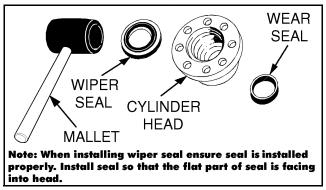
Figure 5-67. Wiper Seal Installation
