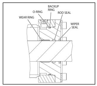
Figure 5-37. Cylinder Head Seal Installation
