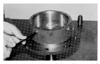
**8.** Bearing spacer (1H) is installed around the output shaft (1A) and locates on bearing cone (1F).
