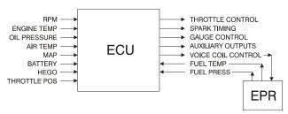
Figure 3-110. LPG Engine Control Unit (ECM)
