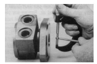
**NOTE:** The depth or location of bearing/bushing (13) in relation to the housing wear plate surface and the depth or location of bearing/bushing (19) in relation to the beginning of bearing/bushing counterbore should be measured and
