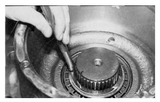
**11.** Upon completion of step 10, rap the internal end of the output shaft (1A) twice with a piece of soft metal rod. This will release the preload which was on the bearings.
