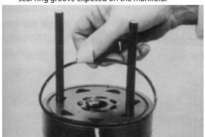
**17.** Assemble the commutator ring (6) over alignment studs onto the manifold.
