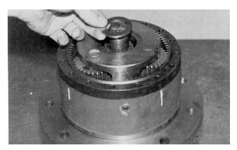
**10.** Thrust washer (11) is installed into the counterbore of the carrier (3).
