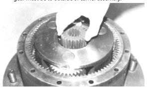
**19.** After inserting at least one shoulder bolt in the proper location, rotate the carrier. Check freedom of rotation and timing.
