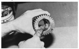
i. Place sixteen needle rollers into cluster gear bore.
