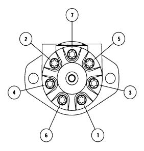
**4.** Install capscrews and seal washers (if applicable) in end cap. Pre-tighten screws to 40 in. lbs. (7.4 Nm). Make sure seal washers are properly seated. Then torque screws to 235-250 in. lbs. (27-28 Nm) in sequence, as shown above.
