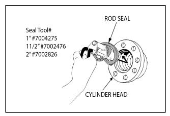
Figure 5-86. Rod Seal Installation
