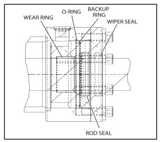
Figure 5-22. Cylinder Head Seal Installation
