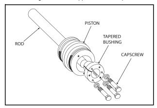
Figure 5-11. Tapered Bushing Installation
