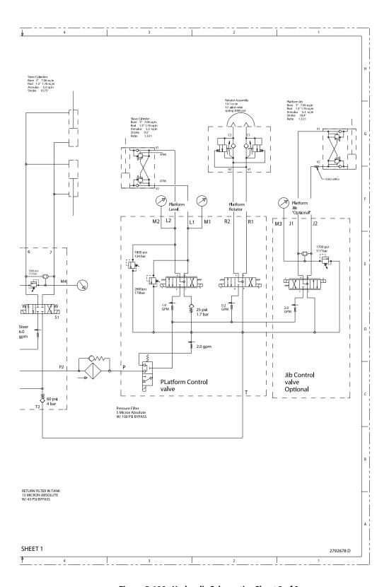
Figure 5-100. Hydraulic Schematic - Sheet 2 of 8
