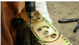
**3.** Remove the screws from the flat bar on the other side of the powertrack.
