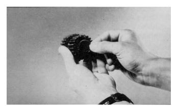
**5.** Apply grease or petroleum jelly to the tang side of two thrust washers. Place thrust washers against bosses in carrier with washer tang fitting into slot in carrier outside diameter.
