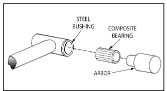
Figure 5-74. Composite Bearing Installation
