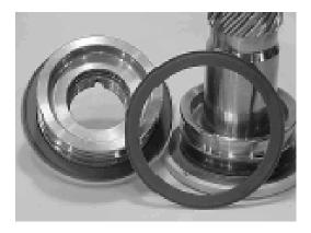
1. Gather all the components and tools into one location prior to re-assembly. Use the cut away drawing to reference the seal orientations.
