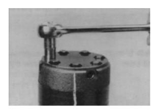
**3.** Remove the five, six, or seven special ring head bolts (1) using an appropriate 1/2 or 9/16 in. (12.7 or 14.28 mm) size socket. Inspect bolts for damaged threads, or sealing rings, under the bolt head. Replace damaged bolts.
