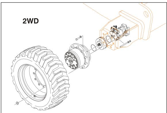
Figure 3-5. Drive Hub Installation - 2WD (Prior to SN 0300083331)
