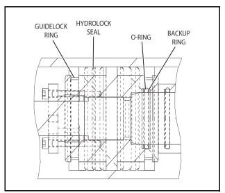
Figure 5-28. Piston Seal Kit Installation
