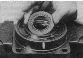
**14.** Check exposed portion of coupling shaft (12) to be sure you have removed all signs of rust and corrosion which might prevent its withdrawal through the seal and bearing. Crocus cloth or fine emery paper may be used.
