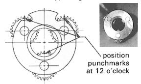
**16.** With shoulder side of ring gear (21) facing down, place ring gear over (into mesh with) large gears. Ensure punch marks remain in correct location during ring gear installation.
