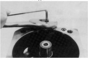
**12.** Remove the threaded pin (stopper - max flow).
