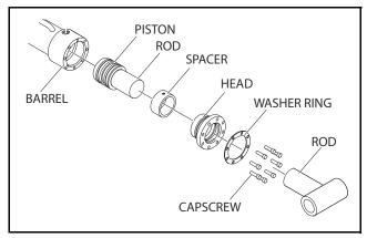
Figure 5-59. Rod Assembly Installation
