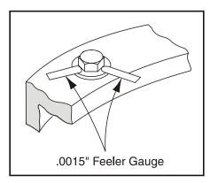
Figure 3-77. Swing Bolt Feeler Gauge Check.
