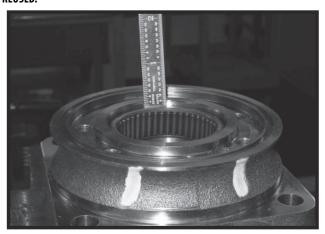
2. The Torqmotor™ inner housing bearing/bushing (13) can now be pressed into its counterbore in housing (18) flush to 0.03 in. (.76 mm) below the housing wear plate contact face. Use the opposite end of the bearing mandrel that was used to press in the outer bearing/ bushing (19).
