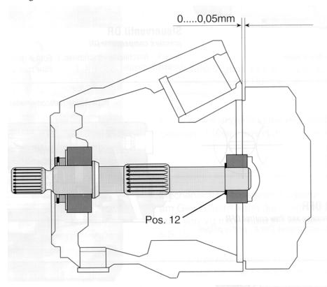
Cast iron pump housing must have initial tension of the bearings: 0......0,05 mm, grind Pos. 12 if necessary.
