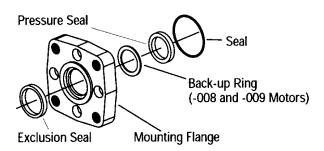
**16.** Exclusion seal, backup ring, pressure seal and seal will come off with flange. Use seal removal tool as shown to remove exclusion and pressure seals.
