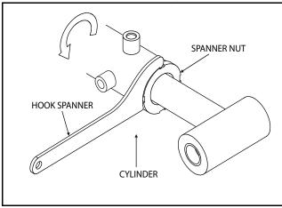
Figure 5-61. Spanner Nut Support
