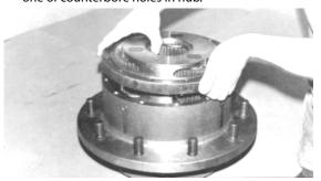
**NOTE:** If gears do not mesh easily or carrier assembly does not rotate freely, then remove carrier and ring gear and check cluster gear timing.
