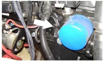
Lube Point(s) - Fill Cap/Spin-on Element Capacity - 4.5 qt. (4.25 L) w/filter Lube - EO Interval - 3 Months or 150 hours of operation Comments - Check level daily/Change in accordance with engine manual.
