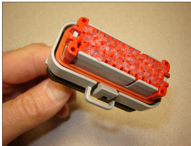
Figure 7-7. Dielectric Grease On Female Contacts
