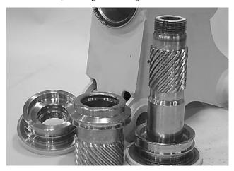
2. Inspect the thrust washers (304) for rough or worn edges and surfaces. Measure it's thickness to make sure it is within specifications (Not less than 0.092" or 2.34 mm).
