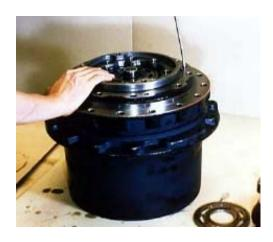
5. Remove brake piston (17) by blowing compressed air from oil passage of parking brake release port. Remove also collar (21) using a jig.
