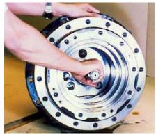
20. Assemble shaft (2) press fitted with inner ring of roller bearing (3), engaging it with spline at tip of drive gear (1-22).
