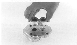
13. Remove the front bearing block.
