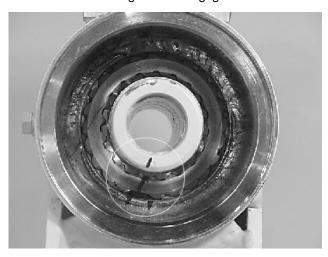
12. Install 2 bolts in the threaded holes in the flange. Using a bar, rotate the shaft in a clockwise direction until the wear guides are seated inside the housing bore.
