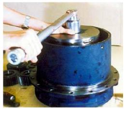
**19.** Loosen plug (1-5), and remove ring nut (1-4) using a jig.
