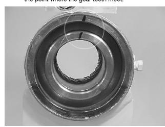
9. Looking from the opposite end of the housing (1) you can see if your timing marks are lining up. When they do, tap the piston (3) in until the gear teeth mesh together. Tap the piston into the housing the rest of the way until it bottoms out.
