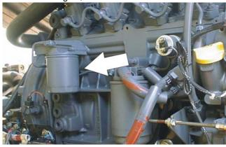
Lube Point(s) - Fill Cap/Spin-on Element
