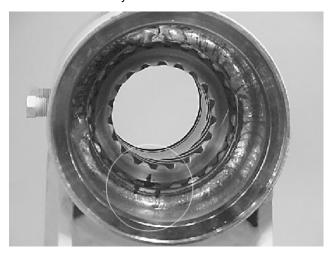
**10.** Install the shaft (2) into the piston (3). Be careful not to damage the seals. Do not engage the piston gear teeth yet.
