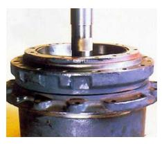
**19.** Press oil seal (4) to flange holder (1-1), and assemble outer ring sub-assembly of roller bearing (3).
