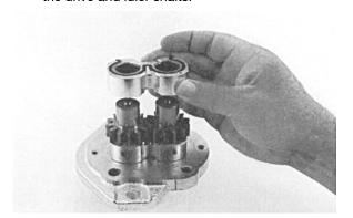
Remove rear bearing block from drive and idler shafts.
