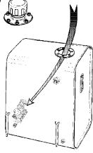
Lube Point(s) - 2 Interval - Every 2 years or 1200 hours of operation, remove and clean at time of hydraulic oil change.
