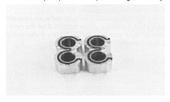
4. Place the E-seals, flat side outward, into the grooves in both bearing blocks. Follow by carefully placing the backup ring, flat side outward, in the groove made by the E-seal and the groove in the bearing block. (Note: in the W900 series pump, in the center of the backup ring and E-seal there is a notch make sure that these notches line up so the backup ring will set flush with the E-seal). The backup ring in the W1500 pump is symmetrical.
