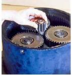
**12.** Assemble needle bearing (1-19) and planetary gear A (1-18) in this order, and then assemble drive gear (1-22).
