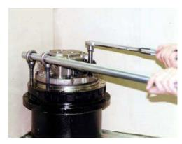
31. Tighten socket head bolts (47) to specified torque.
