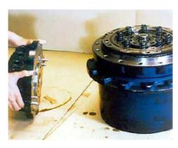
30. Assemble base plate on reduction gear.
