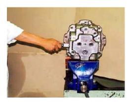
**27.** Grip base plate (32) with vise, and assemble plunger sub assembly (33).
