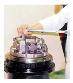
**11.** Loosen plug (55), and pull out spring seat (59), spring (58), and poppet (57).
