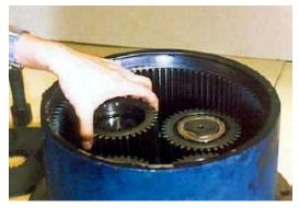
**18.** Remove planetary gear B (1-9), needle bearing (1-10), floating bushing (1-11), and thrust washer (1-12).
