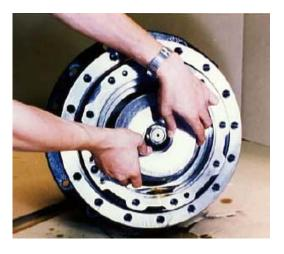
Remove swash plate (5), steel balls (6), piston (24), and spring (25).
