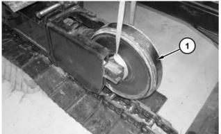
Position suitable cribbing under hydraulic track adjuster (2). Remove bolts (3). Remove front idler (1). The weight of front idler (1) is approximately 68 kg (150 lb).
