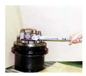
2. Loosen plug (38-6), and remove relief valve (38). Plug (38-6) and relief housing sub assembly (38-1) are lightly press fitted. If they come off, remove them while turning by pinching the circumference of relief housing sub assembly (38-1) with long nose pliers.
