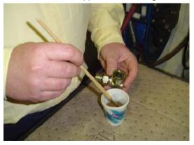
Holding the fitting over the hydraulic oil container, brush an even film of oil around the entire o-ring in the fitting, making sure the entire o-ring is completely saturated.
