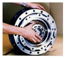
22. Assemble cylinder block sub assembly which have been assembled in foregoing sections 16, 17 and 18, using spline of shaft as a guide. Then, assemble disk (16) and friction plate (62).
