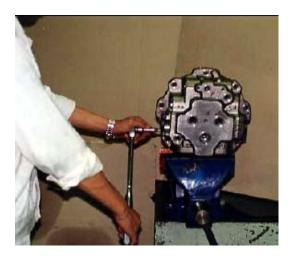
**8.** Grip the base plate (32) with vise. Loosen socket head bolts (60) to remove flange (37).
