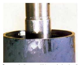
**20.** Secure reduction gears (1) to angular bearing disassembly jig, and place plate on flange holder (1-1). Then, pull out press fit of angular bearing (1-3) by pushing flange holder (1-1) with a press.
