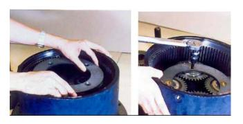
9. Place thrust plate (1-13) and tightly fasten screw (1-14) applied with Loctite #262.
