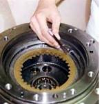
**6.** Pull out cylinder block (7), pin (12), retainer holder (13), retainer plate (14), and piston sub assembly (15).
