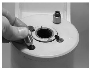
**5.** Using a metal bar, or something similar, unscrew the end cap (4) by turning it counter clockwise.
