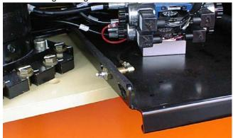
Lube Point(s) - 2 Grease Fittings Capacity - A/R Lube - MPG
