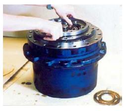
**24.** Assemble collar (21) on brake piston (17), and then assemble it on flange holder (1-1).
