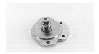
Install new shaft seal in mounting flange with part lumber side facing outboard. Press the seal into the seal lore until the seal reaches the bottom of the bore. Uniform pressure must be used to prevent misalignment or damage to the seal.
