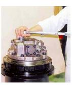
33. Insert spool (39) and spring (40) into base plate, and assemble plugs (41), (43) mounted with O-rings (42), (43), and then tighten them to specified torque. Assemble poppet (57), spring (58) and spring seat (59) in this order, and tighten plug (41) to specified torque.
