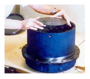
13. Assemble thrust plate (1-23).
