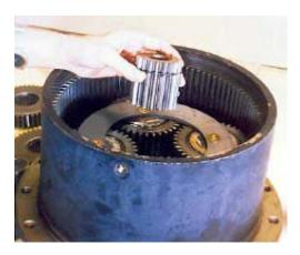
**10.** Assemble sun gear B (1-15) mounted with snap ring (1-16).
