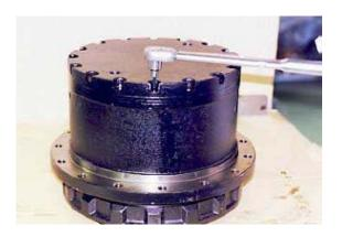
**15.** Apply Loctite #262 (16 locations) to bolt (1-29), and tighten it to specified torque. Apply seal tape to plugs (1-8), (1-5) and tighten them to specified torque.
