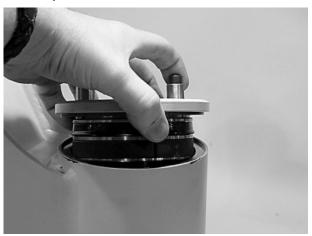
Remove the stop tube if included. The stop tube is an available option to limit the rotation of the actuator.
