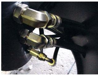
**28.** Repeat hose routing process on LH side frame with correct hoses to drive motor.
