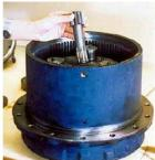
15. Remove thrust plate (1-23) and drive gear (1-22).
