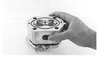
Carefully remove gear housing and place on work bench. Make sure the rear bearing block remains on the drive and idler shafts.
