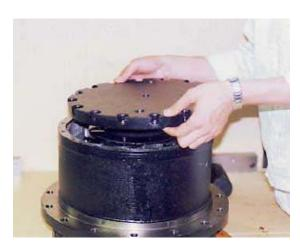
**14.** Apply liquid gasket (ThreeBond 11041) evenly to the circumference of contact surface of cover (1-27) and housing (1-6), and assemble cover so that bolt holes will align.
