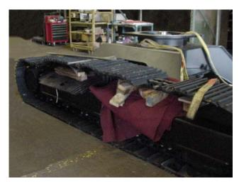
47. Apply never seez to pin. Line up end links. start pin in hole by driving with a hammer. Place portable power pin press over track and pin. place washers in press ends. Actuate switch to operate press, then carefully press in track pin.
