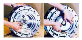
21. Assemble steel ball (6), spring (25) and piston sub assembly (24), and then assemble swash plate (5).
