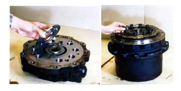
Remove valve plate (26) and O-ring (31), and pull out pins (23), (27) with pliers. Remove also spring (22).
