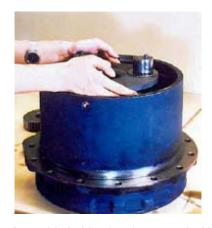
**11.** Assemble holder (1-17) mounted with inner race (1-20) and spring pin (1-21).
