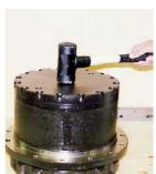
**14.** Remove plugs (1-8), (1-5) and bolt (1-29). Tap the center of cover (1-27) with plastic hammer. When cover (1-27) starts to float up, remove cover (1-27).
