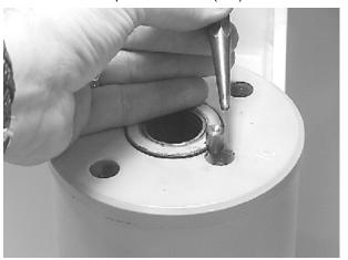
**20.** Remove the piston I.D. seal (200). You may now proceed to the inspection process.
