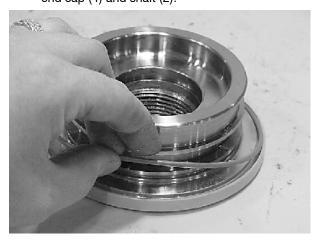
19. Remove the piston O.D. seal (202).
