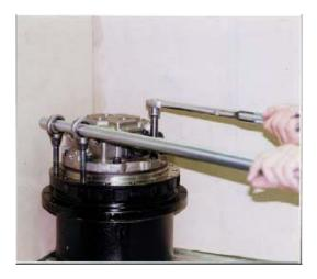
3. Loosen socket head bolts (47), (50) to remove base plate (32). If it is tight to remove, lightly tap it with a plastic hammer in the pulling direction.
