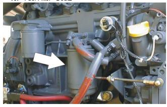
Lube Point(s) - Replaceable Element Interval - Every Year or 600 hours of operation
