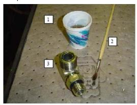
Hold the fitting in one hand while using the brush with the other hand to dip into the container. Remove excess hydraulic oil from the brush so an even film of oil is applied on the o-ring.
