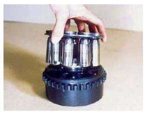
**18.** Assemble piston sub assembly (15) on retainer plate (14), and assemble it on cylinder block (7).
