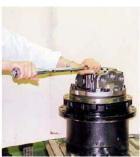
**34.** Assemble bonded seal (51) and socket head bolt (50) in this order. Lubricate one location of socket head bolt (50) with specified amount (2600 cc) of tightening lubricant, and then tighten remaining plug (45) and socket head bolt (50).
