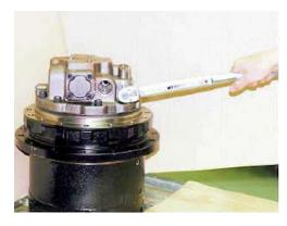
**32.** Assemble relief valve sub assembly (38) on base plate (32), and tighten it to specified torque. Assemble poppet (57), spring (58) and spring seat (59) in this order, and tighten plug (41) to specified torque.
