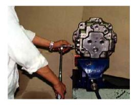
**28.** Assemble spring seat (34) and spring (35) in this order. After assembling flange (37), tighten socket head bolts (60) to specified torque.
