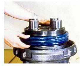
21. Remove angular bearing inner ring sub assembly (1-3) and floating seal (1-2).
