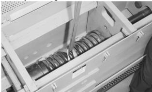
**NOTE:** Do not remove the lifting device from the recoil spring assembly until the unit is leveled, centered, and locked in Tooling (A).
