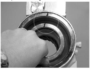
**14.** Remove the o-ring (204) and backup ring (207) from end cap (4) and set aside for inspection.
