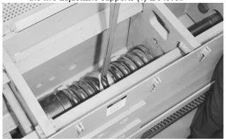
6. Adjust the spacing between reaction plate (2) and movable plate (3) so that the spacing is approximately the same length as the recoil spring assembly.
