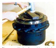
**25.** Place a positioning jig, and insert brake piston by lightly tapping jig head evenly with a plastic hammer.
