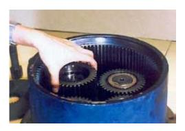
8. Install thrust washer (1-12), floating bushing (1-11), needle bearing (1-10) and planetary gear (1-9) to the flange holder (1-1) in this order.
