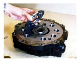
29. Secure base plate (32) on workbench, and assemble outer ring sub assembly (27) of roller bearing (28), pin (27), pins (23) (4 pieces) and O-rings (43) (2 pieces), and then assemble valve plate (26).
