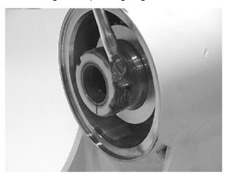
**15.** Install the 0-ring (204) and back-up ring (207) into the inner seal groove on the end cap (4).
