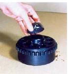
17. Apply grease to pins (12) and insert each pin into three holes on cylinder block (7). Then, assemble retainer holder (13).
