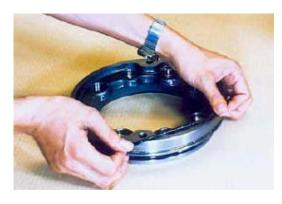
23. Assemble greased O-rings (18), (20) and back-up rings (21), (54) on brake piston (17). Assemble greased O-ring (54) on collar (21).
