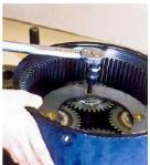
17. Remove sun gear B, and loosen screw (1-14) to remove thrust plate (1-13).
