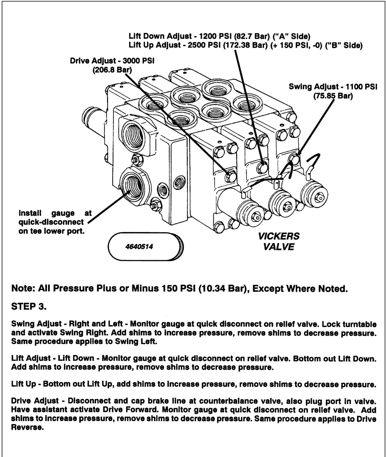
Figure 2-20. Vickers Proportional Valve Pressure Setting, Machines Built Prior To 1989 With Accessory Valve. (Sheet 3 Of 4)
