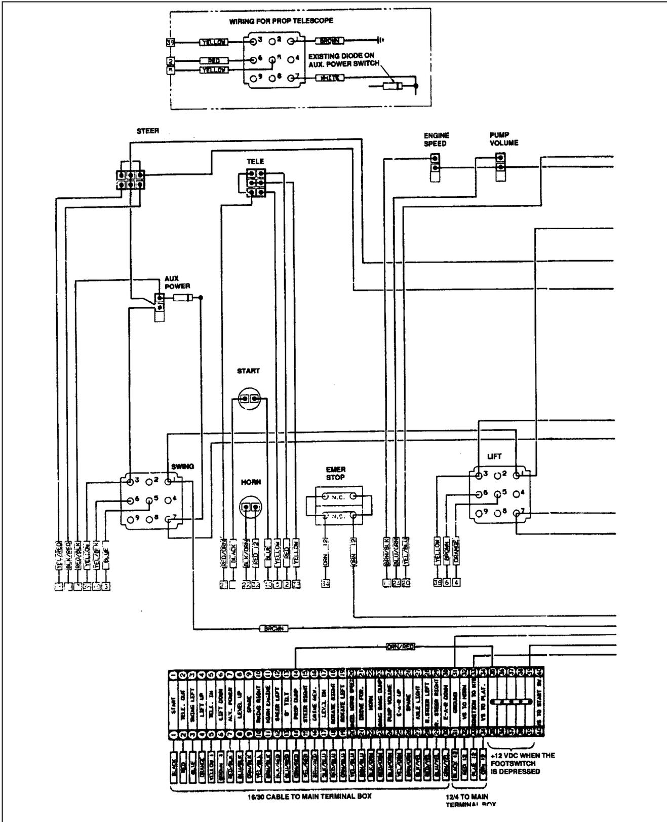
Figure 3-5. Wiring Diagram - Platform Console Standard (Sheet 1 Of 2).
