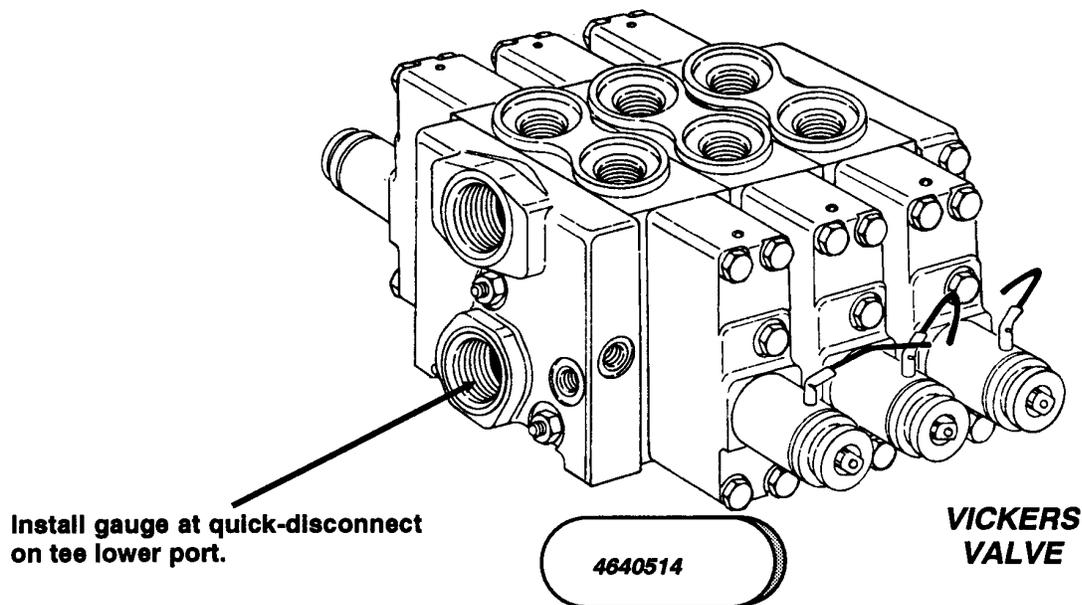
Figure 2-21. Vickers Proportional Valve Pressure Setting, Machines Built Prior To 1989 With Accessory Valve. (Sheet 4 Of 4)
