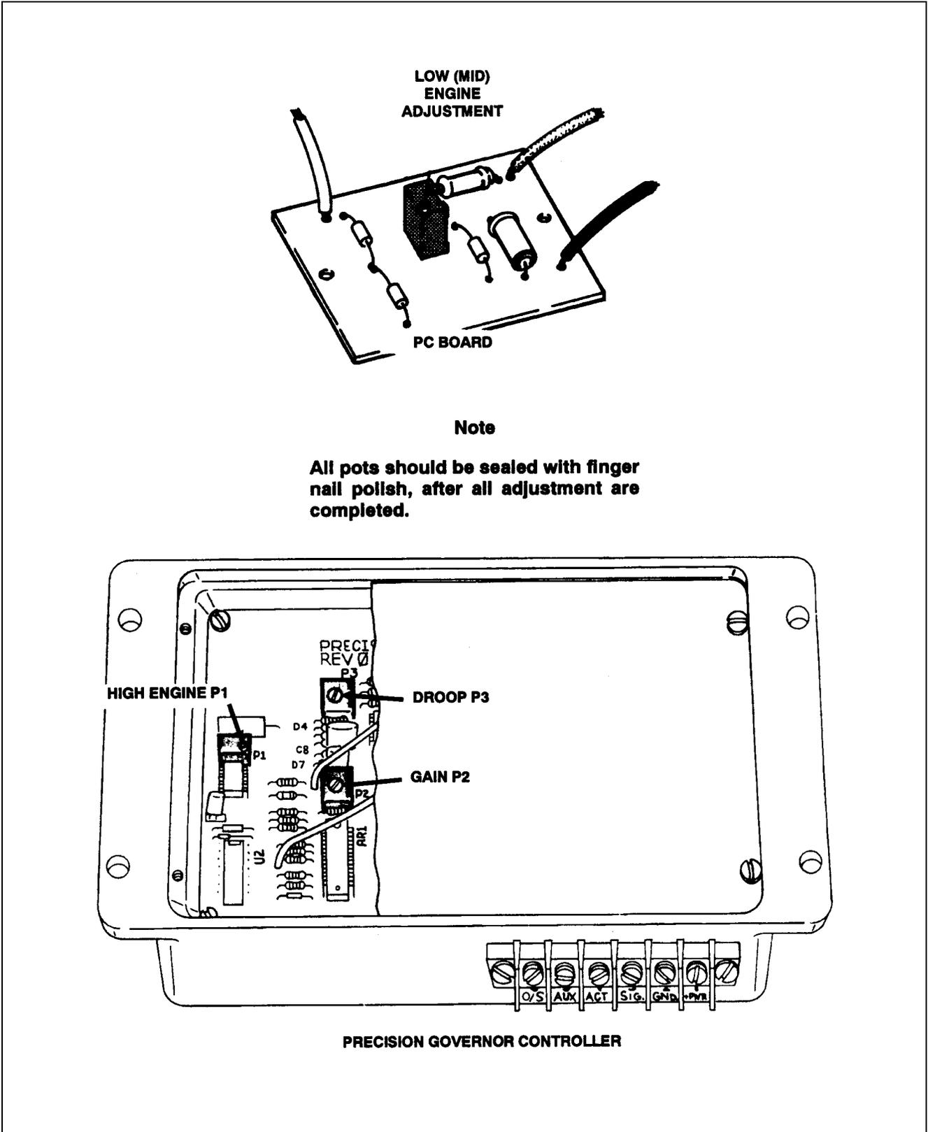
Figure 2-7. Precision governor Adjustment, Ford. (Sheet 2 of 2)
