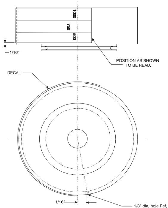
Figure 2-49. Capacity Indicator Dial
