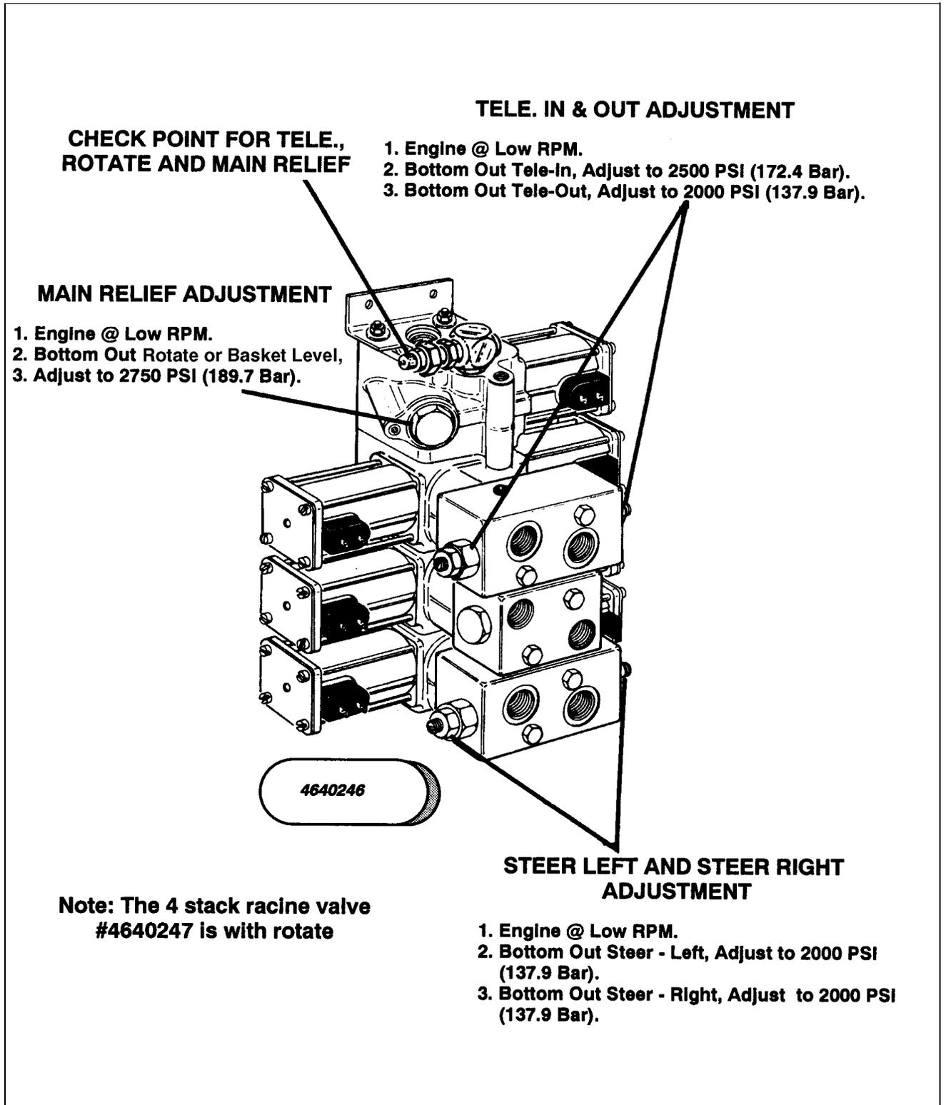
Figure 2-28. Solenoid Valve Pressure Settings, Machines Built Before 1995. (Sheet 1 of 2)
