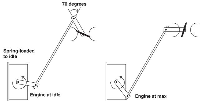
The needed travel of the carburetor determines how far out the Actuator arm the rod is to be attached. In most cases, The carburetor should be moved from closed to above 10 degrees from full open as the Actuator is moved min. to max. THEN ALTER THE LENGTH OF THE ROD SLIGHTLY (PERHAPS .030"), SO THAT THE ACTUATOR IS JUST OFF ITS INTERNAL STOP, AND IS PULLING THE BUTTERFLY AGAINST ITS STOP. This insures that the carburetor can fully close to idle on load dumps, minimizing over speeds.
