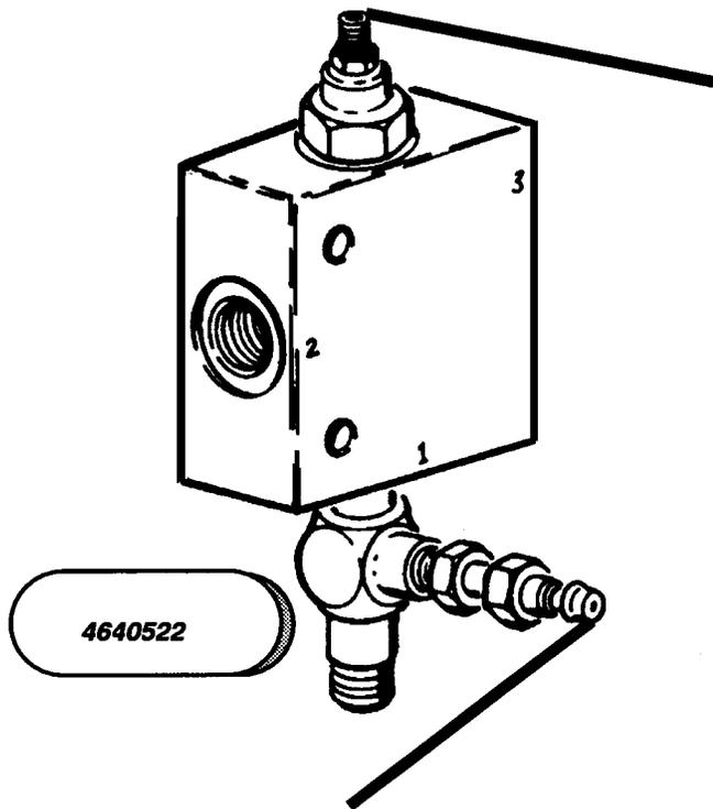
Install Pressure Gauge At Quick Disconnect.
