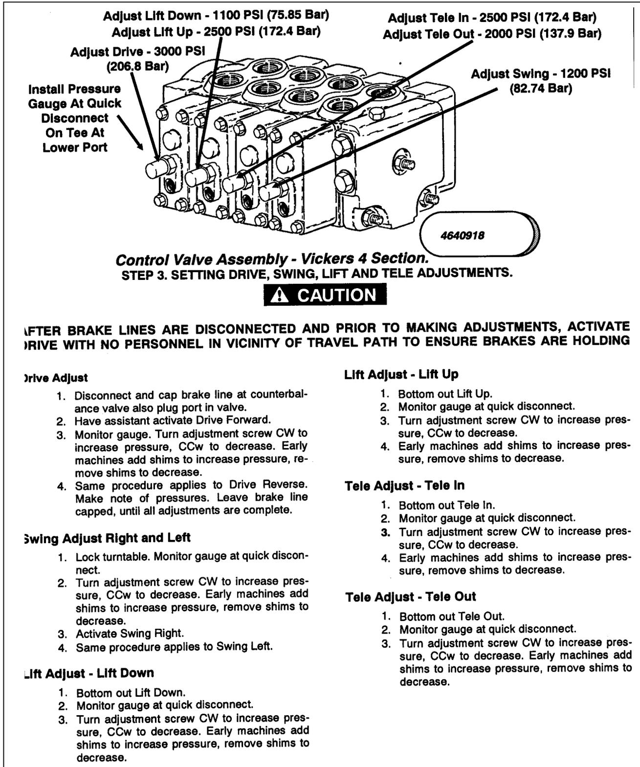
Figure 2-25. Vickers All Hydraulic Machines Pressure Settings (Sheet 2 of 4).
