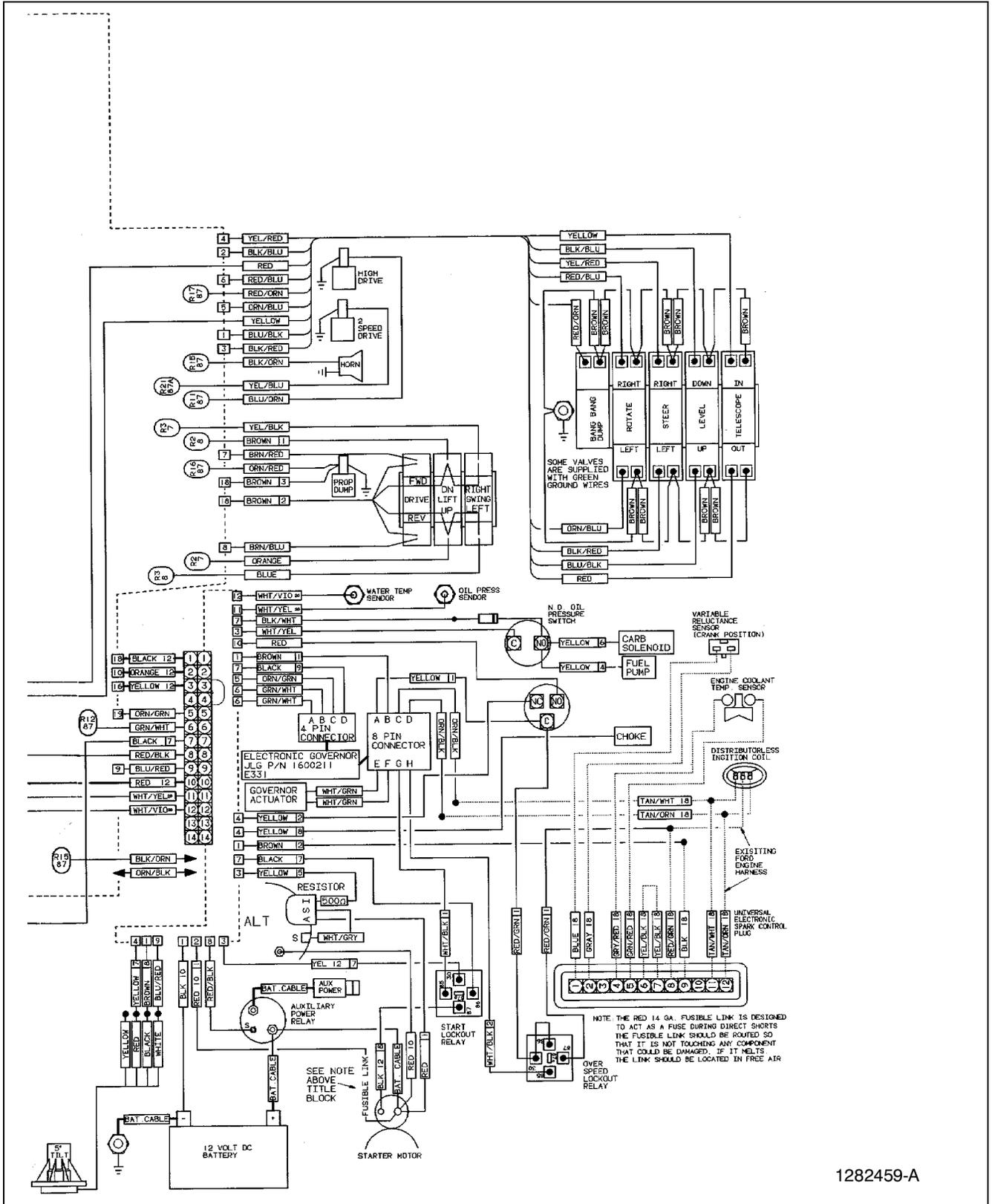
Figure 3-16. Wiring Diagram - Standard (Ford Lrg425 Dis Engine W/ Standard Controls) (Sheet 2 Of 2).
