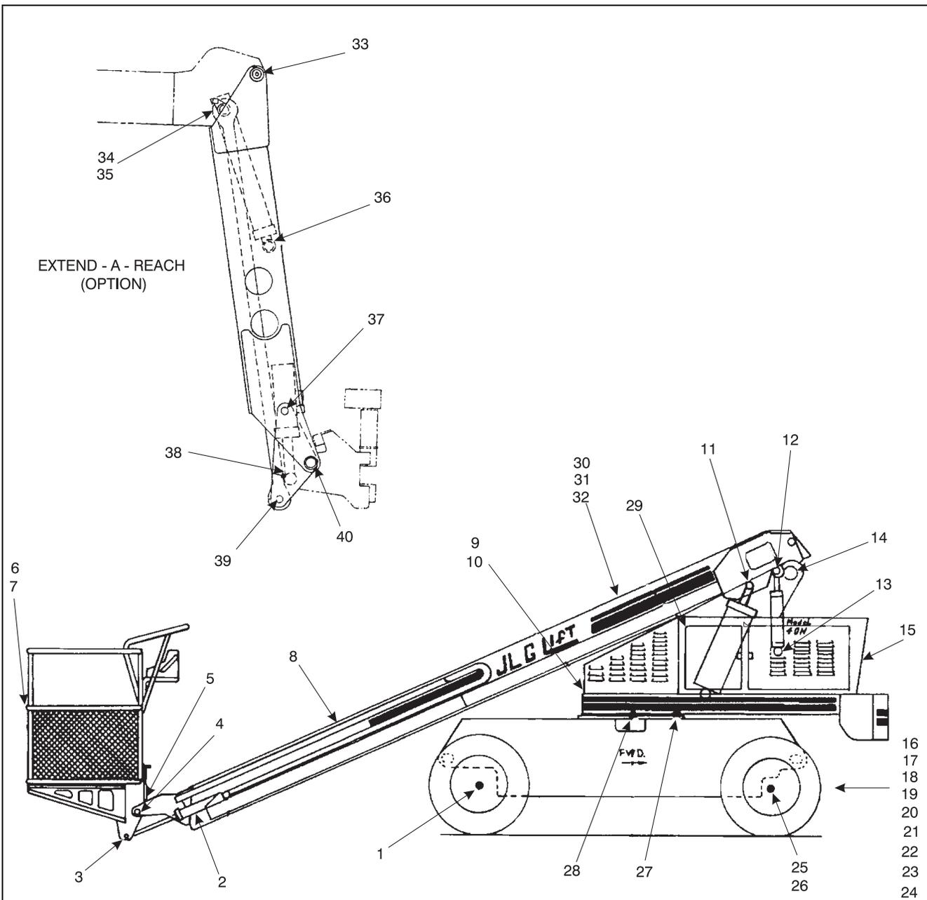
30, 31, 32, ENGINE OIL, HYDRAULIC FILTER ELEMENTS, HYDRAULIC FLUID SIGHT GAUGE ARE ON OPPOSITE SIDE OF MACHINE.
