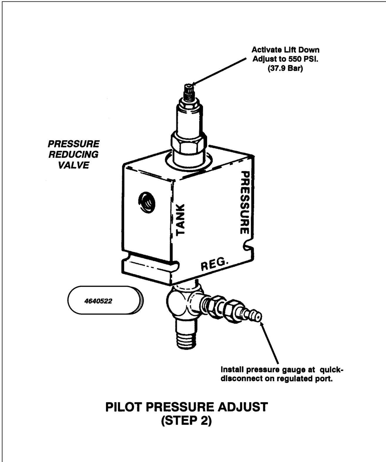
Figure 2-15. Vickers Proportional Valve Pressure Setting, Machines Built To Present. (Sheet 2 of 4)
