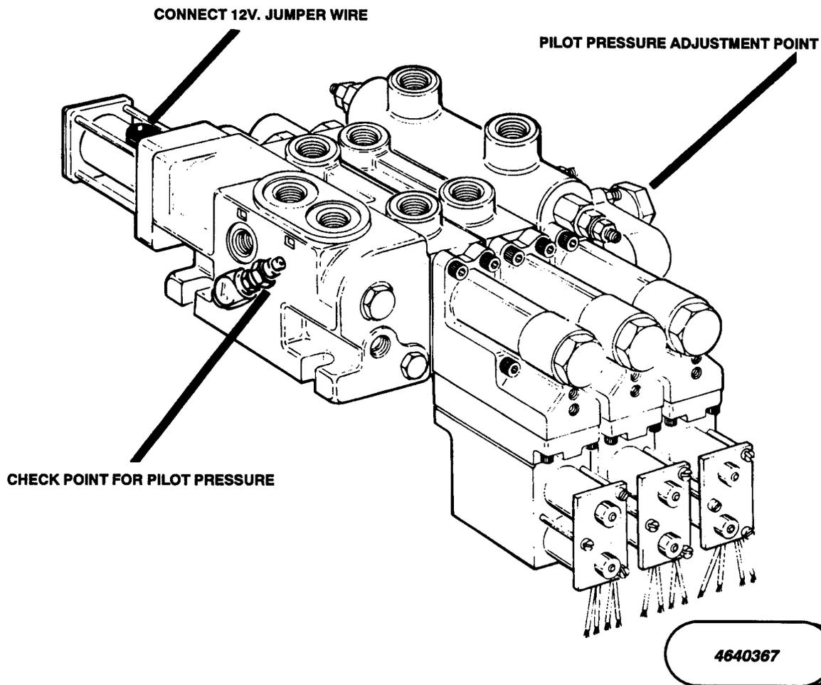
Figure 2-13. Racine Proportional Valve Setting.(Machines Built Prior To Mid 1967) (Sheet 2 of 2)
