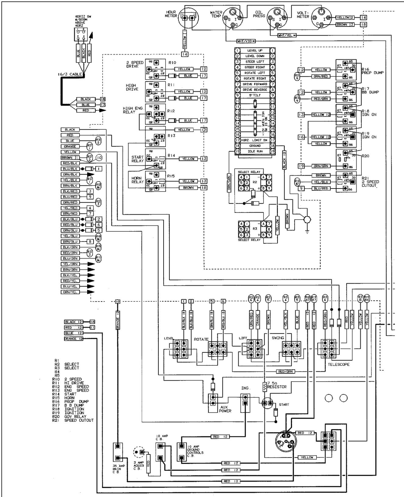
Figure 3-15. Wiring Diagram - Standard (Ford Lrg425 Dis Engine W/ Standard Controls) (Sheet 1 Of 2).
