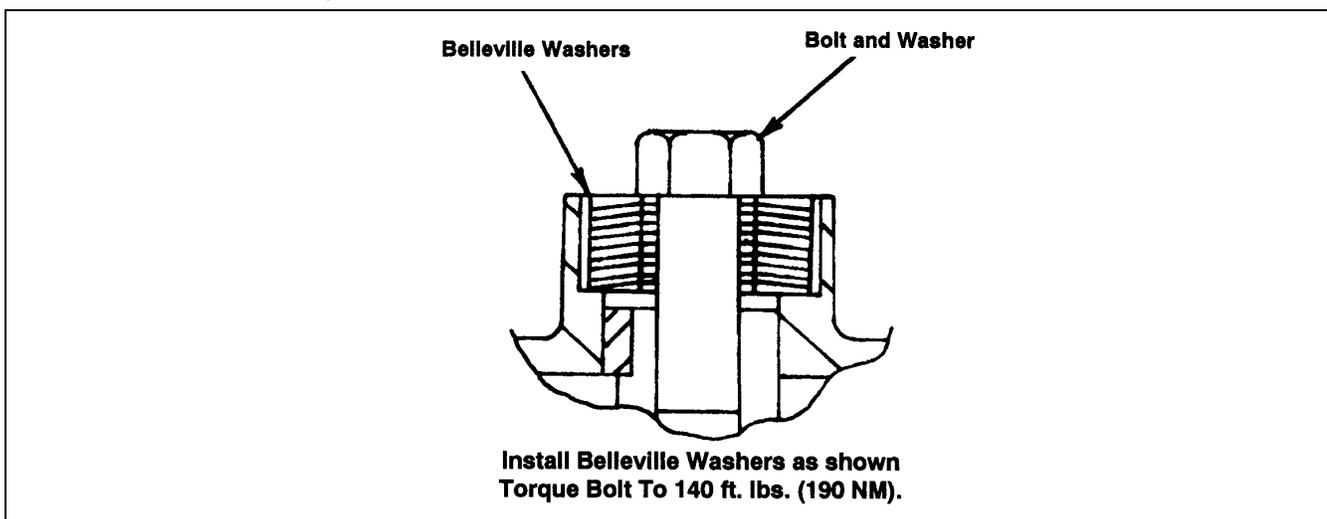
Figure 2-47. Basket Rotator Brake.
