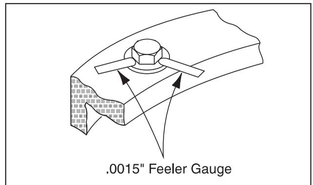
Figure 2-33. Swing Bolt Feeler Gauge Check.
