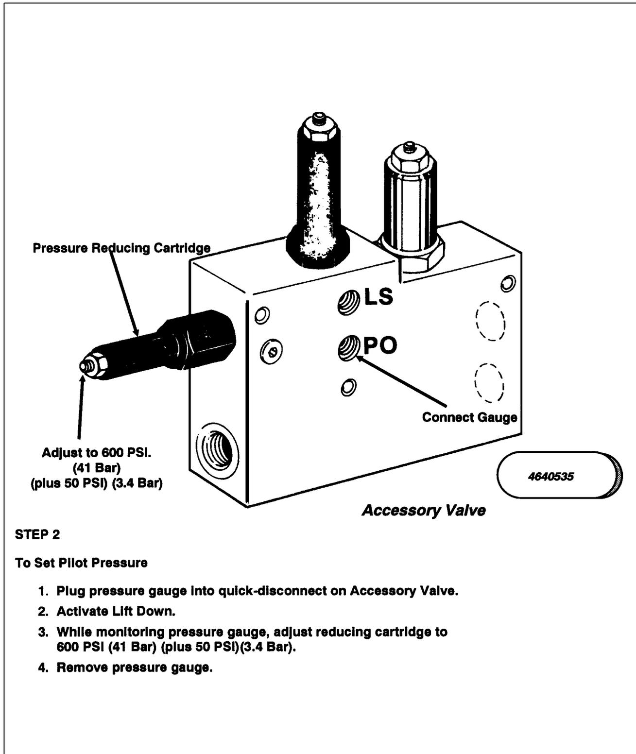
Figure 2-19. Vickers Proportional Valve Pressure Setting, Machines Built Prior To 1989 With Accessory Valve. (Sheet 2 of 4)
