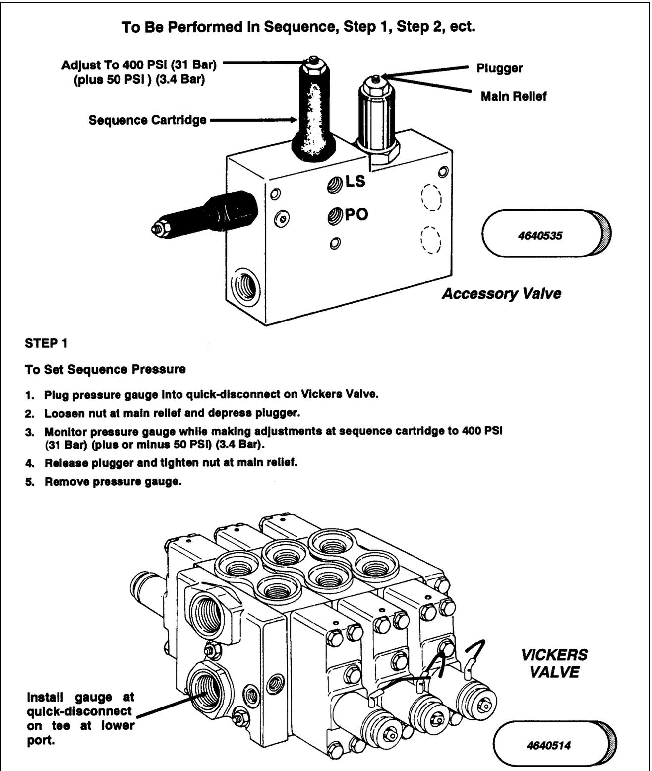
Figure 2-18. Vickers Proportional Valve Pressure Setting, Machines Built Prior To 1989 With Accessory Valve. (Sheet 1 of 4).
