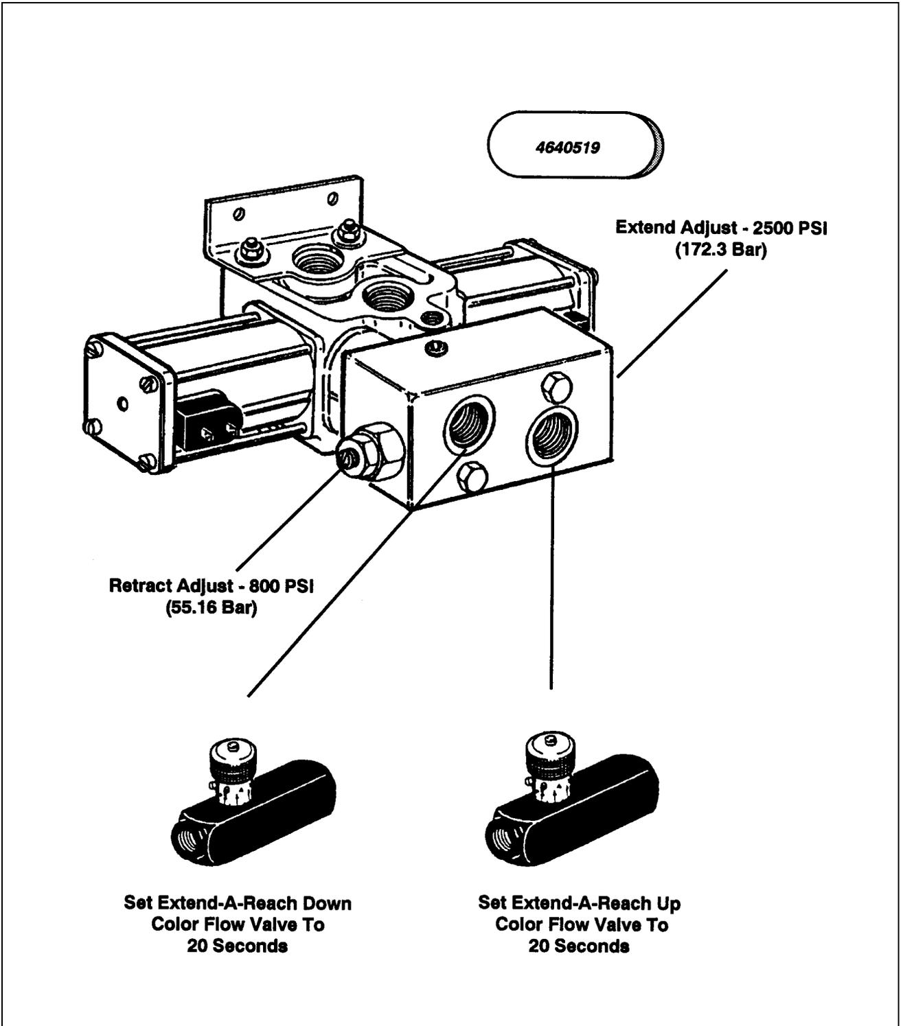
Figure 2-30. Extend-A-Rich Valve Pressure and Speed Settings Model 40+6.
