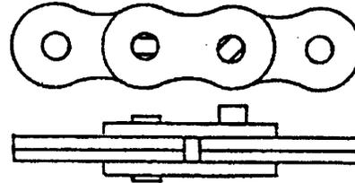
Also, more than one crack can often appear on a link plate. In addition to rusting, this condition can be caused by exposure to an acidic or caustic medium or atmosphere. Stress corrosion is an environmentally assisted failure. Two conditions must be present - corrosive agent and static stress. In the chain, static stress is present at the aperture due to the press fit pin.
