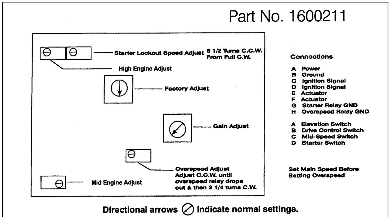
**NOTE:** These settings are factory set, Start Lockout, Factory Adjust and Overspeed. They are conformally coated by P.G. and should not need to be reset.
