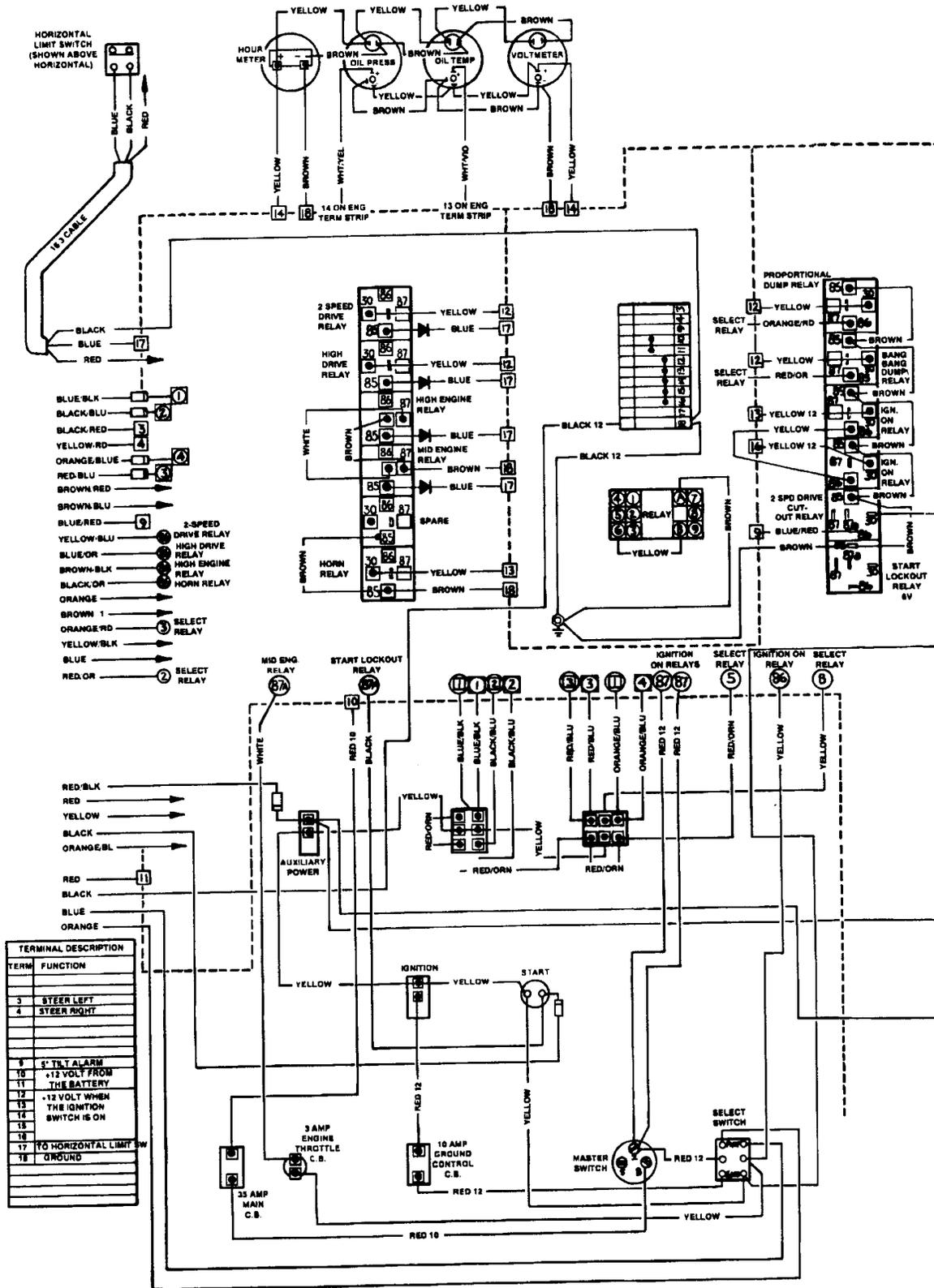
Figure 3-13. Wiring Diagram - Standard (Deutz F31011 Engine W/ Hydraulic Controls) (Sheet 1 Of 2).
