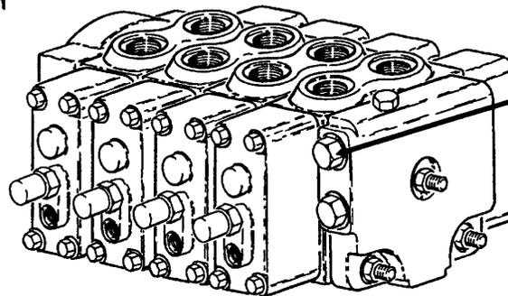
**Control Valve Assembly - Vickers 4 Section.**
