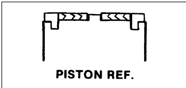
Figure 2-3. Poly-Pak Seal Installation.
