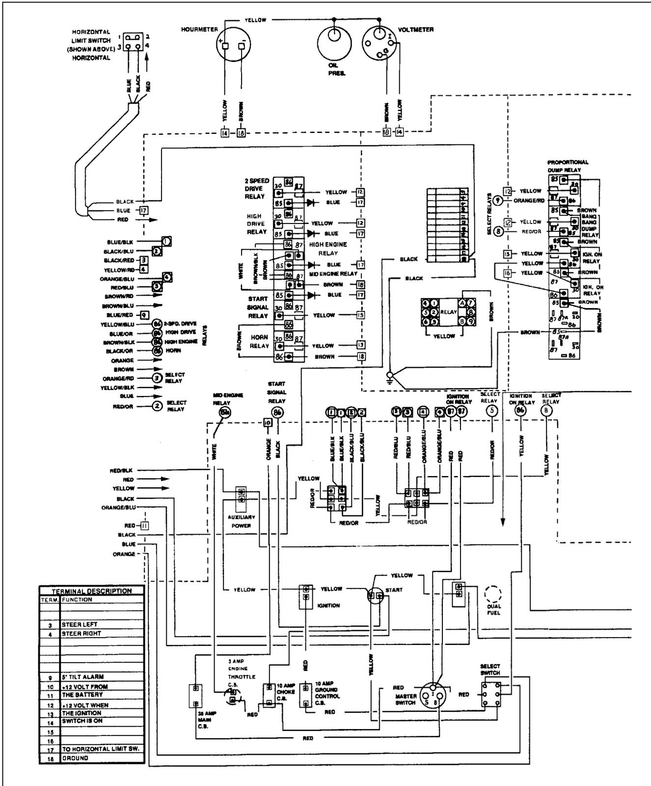
Figure 3-9. Wiring Diagram - Standard (Deutz F21511/f31912 & Engine W/ Hydraulic Controls) (Sheet 1 Of 2).
