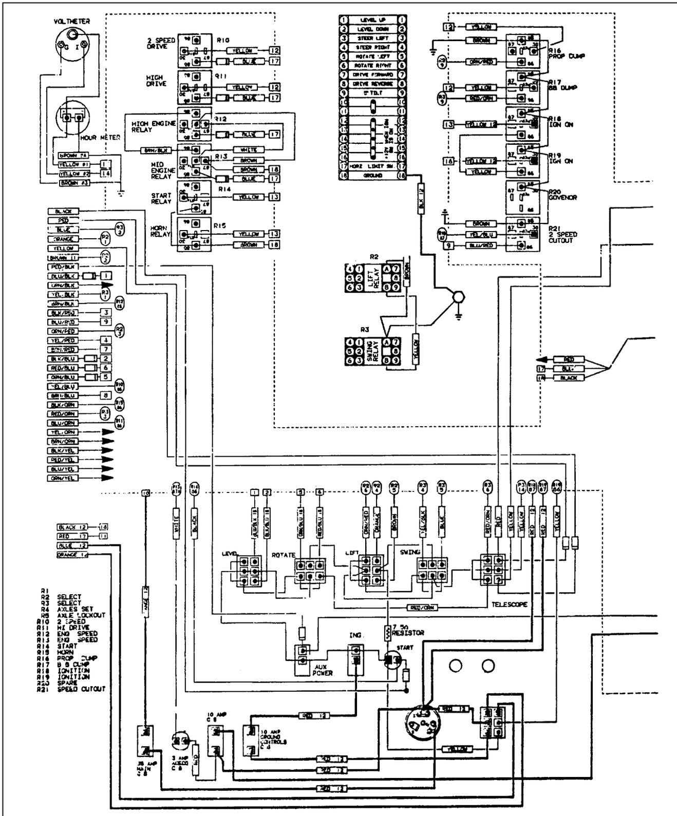
Figure 3-7. Wiring Diagram - Standard (Deutz F21511/f31912 & Wisconsin Engine W/ Standard Controls) (Sheet 1 Of 2).
