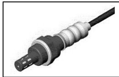
Figure 3-73. Heated Exhaust Gas Oxygen Sensor (HEGO)
