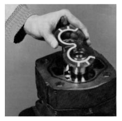
**17.** Position the bearing carrier over the gear housing so the bushings receive the journals of the drive and driven gears. Be sure to line up the dowel holes over the dowel pins. When the parts are parallel, squeeze them together or alternately tap over each dowel until the parts are together.
