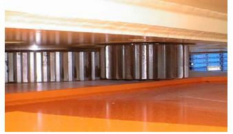
Lube Point(s) - N/A Capacity - A/R Lube - MPG Interval - Every 3 months or 150 hrs of operation Comments - Apply by brush
