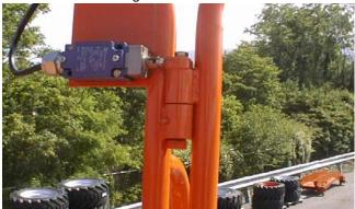
Lube Point(s) - 2 Grease Fittings Capacity - A/R Lube - MPG Interval - Every 3 months or 150 hrs of operation
