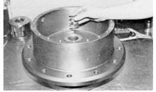
m. Set second spacer washer (42) on top of spring.
