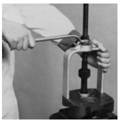
**11.** If the pump is equipped with an outboard bearing, place the shaft end cover in the vise with the mounting face up. Remove the snap ring with snap ring pliers. If the unit is equipped with a spiral lock retaining ring, remove with a small screwdriver or awl.
