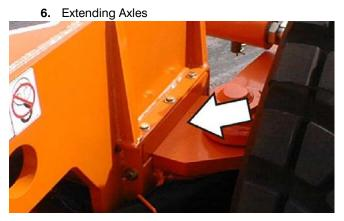
Lube Point(s) - N/A Capacity - A/R Lube - MPG Interval - Every 3 months or 150 hrs of operation Comments - Apply by brush
