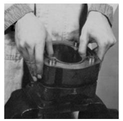
**10.** Inspect all bushings for scoring or discoloration and replace if necessary. Use a bushing puller as shown in the tool list to remove bushings.
