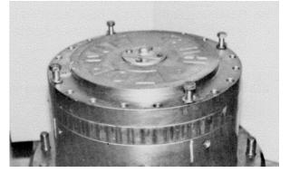
**19.** Install sixteen Grade 8 bolts (1) and lockwashers (3) in remaining holes.
