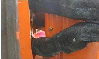
Lube Point(s) - 4 Grease Fittings Capacity - A/R Lube - MPG Interval - Every 3 months or 150 hrs of operation
