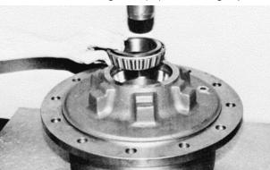
e. Press seal (31) into hub counterbore with flat metal side facing out. Use a flat object to ensure that seal is pressed evenly and is flush with hub face.
