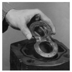
**15.** Slide the driven gear through the housing and into the bushing in the shaft end cover. Coat the steel sleeve tool with grease. Place the lightly greased drive shaft inside the sleeve and slide both through the shaft end cover with a twisting motion until the integral gear rests against the thrust plate. Avoid damaging the double lip seal. Remove the steel sleeve. Squirt clean oil over the gears.
