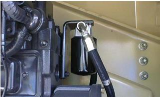
Lube Point(s) - N/A Lube - EO Comments - Refer to Engine Manual for Change interval.
