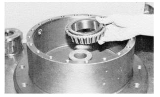
**h.** Place bearing shim (34) over end of spindle and against bearing cone.
