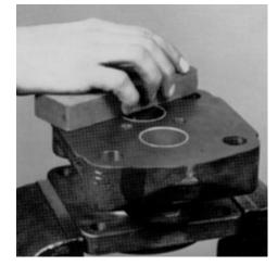
8. See that dowel pins are in place in any new castings. Examine all dowels. Before inserting make sure the hole is clean and free from burrs. Gently start pin straight into hole and tap lightly with a soft hammer.
