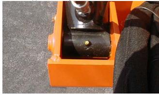
Lube Point(s) - 1 Grease Fitting Capacity - A/R Lube - MPG Interval - Every 3 months or 150 hrs of operation Comments -
