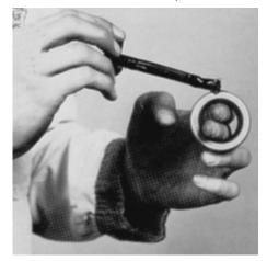
**10.** If the unit is equipped with an outboard bearing, guide the bearing into it's recess in the shaft end cover. This is a light press fit. It may be necessary to lightly tap the bearing into the bore.
