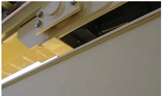
Lube Point(s) - 1 Grease Fitting Capacity - A/R Lube - MPG Interval - Every 3 months or 150 hrs of operation
