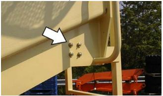
Lube Point(s) - 1 Grease Fitting Capacity - A/R Lube - MPG
