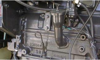
Lube Point(s) - Fill Cap/Drain Plug Capacity - 10 quarts (9.5 L) w/o filter Lube - EO Comments - Check daily. Refer to Engine Manual for Change interval. 19. Engine Oil Filter
