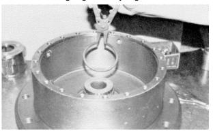
**j.** Install retaining ring keeper ring (40) in location around retaining ring and on bearing shim.
