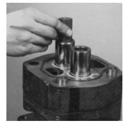
**9.** Lift or pry off the first section gear housing. Be careful not to damage machined surfaces. Examine and replace if necessary.
