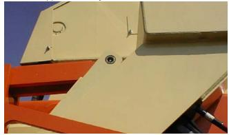
Lube Point(s) - 1 Grease Fitting Capacity - A/R Lube - MPG Interval - Every 3 months or 150 hrs of operation Comments -
