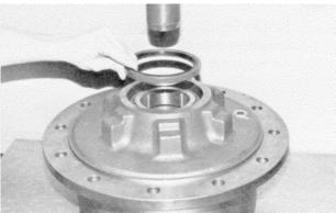
f. Lower hub onto spindle (30) with large open end up.
