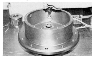
**2.** Position hub/spindle assembly (36 and 30) with large open end up.
