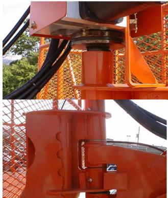
Lube Point(s) - 2 Grease Fittings on pivot; 1 Grease Fitting on worm gear Capacity - A/R Lube - MPG Interval - Every 3 months or 150 hrs of operation 15. Platform Level Links
