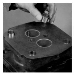
9. Before inserting a new lip seal in the shaft end cover, coat the outer edge of the lip seal and its recess with Permatex Aviation Form-A-Gasket No. 3 non hardening sealant or equivalent. With the metal side of the lip seal up, press it into the mounting flange side of the shaft end cover with an arbor press and bar. Be careful not do damage the lip of the seal. Press in until flush with the recess. Wipe off excess sealant.
