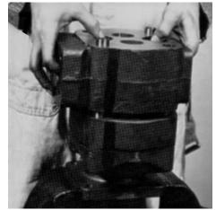
8. Remove the connecting shaft. Remove the thrust plate. Examine and replace if necessary. Remove the driven gear and the integral gear and drive shaft. Keep these together as they are a matched set. Examine and replace if necessary. Be careful not to damage the machined surfaces of the gears.
