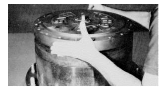
**18.** Secure cover assembly and ring gear to hub with four shoulder bolts (2) and lockwashers 3. Shoulder bolts fit into four counterbored holes in hub. It may be necessary to start bolts into hub by tapping lightly on bolts with a hammer.
