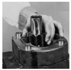
6. Lift the gear housing from the bearing carrier. If prying is necessary, take care not to damage machined surfaces. Examine and replace if necessary.
