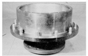
3. Lower internal gear (21) onto spindle.
