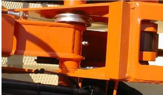
Lube Point(s) - 3 Grease Fitting Capacity - A/R Lube - MPG Interval - Every 3 months or 150 hrs of operation Comments - 27. Upper Master Cylinder Rod End
