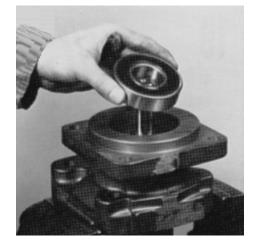
**11.** If the pump is equipped with an outboard bearing, place the shaft end cover in the vise with the mounting face up. Install the snap ring in the groove to retain the outboard bearing.
