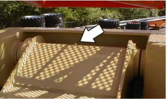
Lube Point(s) - 1 Grease Fitting Capacity - A/R Lube - MPG Interval - Every 3 months or 150 hrs of operation
