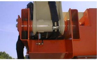
Lube Point(s) - 1 Grease Fitting Capacity - A/R Lube - MPG Interval - Every 3 months or 150 hrs of operation
