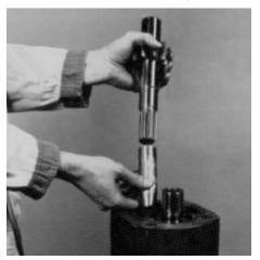
**16.** Slip the thrust plate with seal over gear journals and into the housing bore. The flat side of the seal should face up with the relief groove facing the outlet side.
