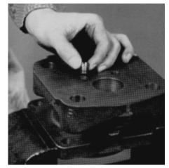
4. New plugs should be screwed in tightly. Stake plug with a prick punch at both ends of screwdriver slot and around edges. Peen edge of hole 0.031 to 0.062 inches with a 1.5 inch diameter steel ball.
