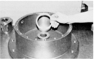
**k.** With large open end of hub/spindle assembly facing up, place one spacer washer (42) into spindle counterbore.
