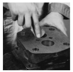
**3.** Grip shaft end cover in a vise with the mounting face down. Examine the plug or plugs to be sure they're tightly in place. Replacement is necessary only if parts are damaged. Remove with a screwdriver.
