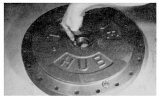
**b.** Install o-ring (8) over cover cap (7).
