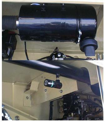
Lube Point(s) - Replaceable Element Interval - Every 6 months or 300 hours of operation or as indicated by the condition indicator
