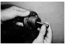
Locate large clearance hole in cover cap over pipe plug in cover and install cover cap in cover. Use two bolts (12) torqued to 70 to 80 in.lbs. (81-92 kgcm).
