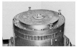
**19.** Install sixteen Grade 8 bolts (1) and lockwashers (3) in remaining holes.
