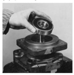
11. If the pump is equipped with an outboard bearing, place the shaft end cover in the vise with the mounting face up. Install the snap ring in the groove to retain the outboard bearing.
