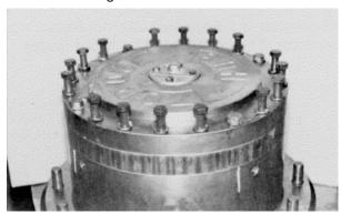
**20.** Tighten bolts and shoulder bolts evenly and torque to 100-110 ft.lbs. (14-15 kgm).
