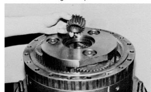
**15.** Place one thrust bearing (16) between two thrust washers (15) and place into carrier counterbore.
