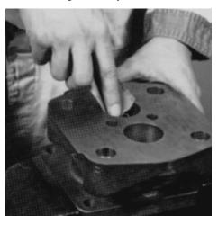
3. Grip shaft end cover in a vise with the mounting face down. Examine the plug or plugs to be sure they're tightly in place. Replacement is necessary only if parts are damaged. Remove with a screwdriver.
