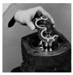
17. Position the bearing carrier over the gear housing so the bushings receive the journals of the drive and driven gears. Be sure to line up the dowel holes over the dowel pins. When the parts are parallel, squeeze them together or alternately tap over each dowel until the parts are together.
