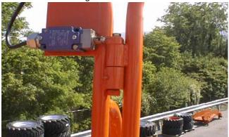
Lube Point(s) - 2 Grease Fittings Capacity - A/R
