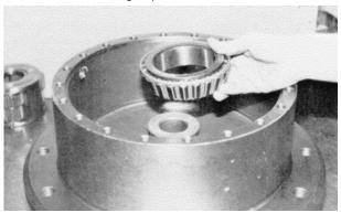
**h.** Place bearing shim (34) over end of spindle and against bearing cone.
