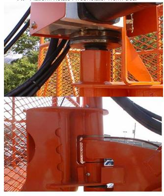
Lube Point(s) - 2 Grease Fittings on pivot; 1 Grease Fitting on worm gear Capacity - A/R Lube - MPG
