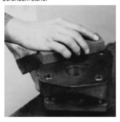
2. If bushings have been removed, deburr the bushing bores with emery cloth. Rinse parts in solvent. Air blast all parts and wipe with a clean lint less cloth before starting assembly.
