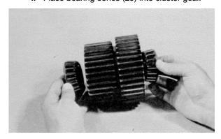
j. Place cluster gear into carrier with large gear up.
