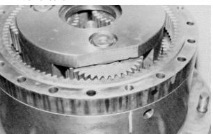
14. Thrust spacer (18) and input gear (17) are installed onto input shaft (20). Counterbore in input gear should be facing thrust spacer.
