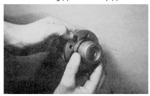
**c.** Install o-ring (10) into bore of cover cap 7. Disconnect rod (9) may be used to push o-ring down to groove in cover cap bore.
