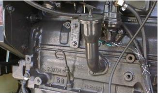
Lube Point(s) - Fill Cap/Drain Plug
