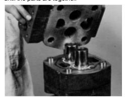
**18.** Insert the connecting shaft in the spline of the drive gear. Position and place the second gear housing on the bearing carrier as outlined in step 12.
