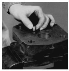
**4.** New plugs should be screwed in tightly. Stake plug with a prick punch at both ends of screwdriver slot and around edges. Peen edge of hole 0.031 to 0.062 inches with a 1.5 inch diameter steel ball.
