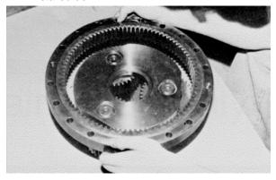
**12.** While holding ring gear in mesh with carrier assembly, lower into internal gear (21). Small diameter cluster gear will mesh with internal gear. Slight rotation of ring gear may be necessary.
