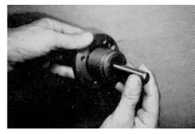
e. Locate large clearance hole in cover cap over pipe plug in cover and install cover cap in cover. Use two bolts (12) torqued to 70 to 80 in.lbs. (81-92 kgcm).
