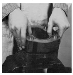
**10.** Inspect all bushings for scoring or discoloration and replace if necessary. Use a bushing puller as shown in the tool list to remove bushings.
