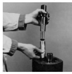
**16.** Slip the thrust plate with seal over gear journals and into the housing bore. The flat side of the seal should face up with the relief groove facing the outlet side.
