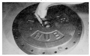
b. Install o-ring (8) over cover cap (7).
