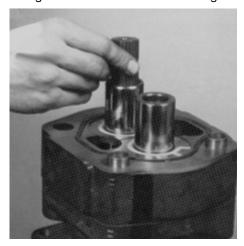
**9.** Lift or pry off the first section gear housing. Be careful not to damage machined surfaces. Examine and replace if necessary.
