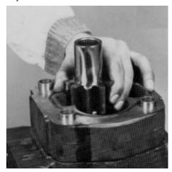
Lift the gear housing from the bearing carrier. If prying is necessary, take care not to damage machined surfaces. Examine and replace if necessary.
