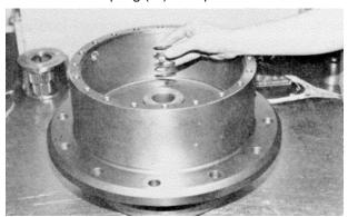
m. Set second spacer washer (42) on top of spring.
