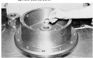
I. Place spring (43) into spindle counterbore.
