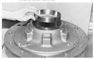
d. Install bearing cone (32) into bearing cup.
