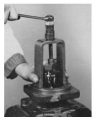
13. Grip the shaft end cover in a vise with the mounting face down. Remove the double lip seal by inserting the special seal removal tool into the notch between the double lip seal and the shaft end cover. Tap the seal out and discard. Remove and discard all rubber and polymer seals.
