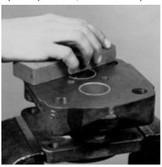
8. See that dowel pins are in place in any new castings. Examine all dowels. Before inserting make sure the hole is clean and free from burrs. Gently start pin straight into hole and tap lightly with a soft hammer.
