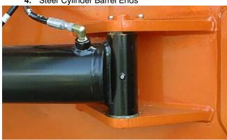
Lube Point(s) - 2 Grease Fittings Capacity - A/R Lube - MPG Interval - Every 3 months or 150 hrs of operation
