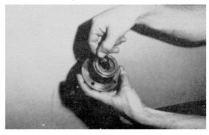
d. Push disconnect rod into bore of cover cap.
