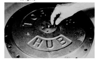
f. Install disconnect cap (11) to cover cap with two remaining bolts (12) torqued to 70 to 80 in.lbs. (81-92 kgcm).
