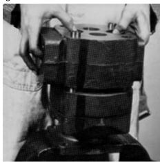
8. Remove the connecting shaft. Remove the thrust plate. Examine and replace if necessary. Remove the driven gear and the integral gear and drive shaft. Keep these together as they are a matched set. Examine and replace if necessary. Be careful not to damage the machined surfaces of the gears.
