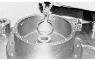
**j.** Install retaining ring keeper ring (40) in location around retaining ring and on bearing shim.
