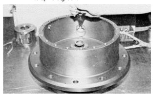
2. Position hub/spindle assembly (36 and 30) with large open end up.
