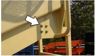
Lube Point(s) - 1 Grease Fitting Capacity - A/R Lube - MPG
