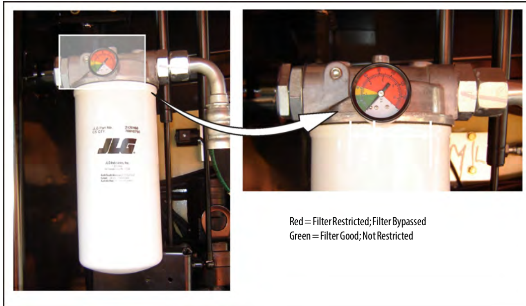
Figure 7-7. Hydraulic Return Filter Condition Indicator
