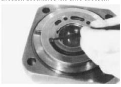
Pumps counterclockwise driven must have a position of the valve plate 4 degrees decentered in the ccw position.
