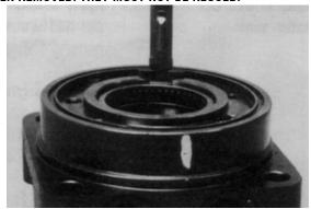
2. The Torqlink™ inner housing bearing/bushing (13) can now be pressed into its counterbore in housing (18) flush to 0.03 inch (.76 mm) below the housing wear plate contact face. Use the opposite end of the bearing mandrel that was used to press in the outer bearing/bushing (19).
