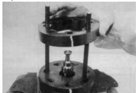
If assembly alignment studs are not being utilized, align stator bolt holes with wear plate and housing bolt holes and turn two bolts (1) finger tight into bolt holes approximately 180 degrees apart to retain stator and wear plate stationary. **3.** Assemble the rotor (8A), counterbore down if applicable, into stator (8B), and onto wear plate (9) with rotor splines into mesh with drive link (10) splines.
