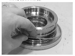
19. Remove the piston O.D. seal (202).
