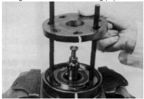
**12.** Apply a small amount of clean grease to a new seal ring (4) and assemble it into the seal ring groove on the wear plate side of the rotor set stator (8B).
