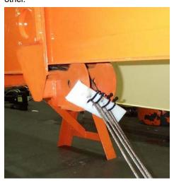
4. Insert the fly into outer mid boom keep it out far enough, about 2 feet (0.6 m, to enable access for installation of the level cylinder pivot pin. **5.** Install the front lower wear pads and shims to the outer mid boom as marked during disassembly.
