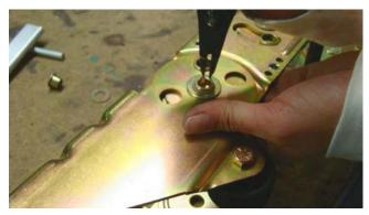
**10.** Push down with slight pressure on the link and slide the bracket side up and over the extrusion on the link.
