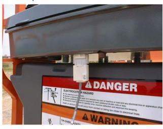
Pull out the Emergency Stop switch and Start the engine.
