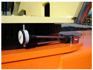
Next, position the main boom fully extended and horizontal as shown in Figure 3-49., Swing Bearing Tolerance Boom Placement - Sheet 2 of 2. Read the measurement recorded on the dial indicator gauge.
