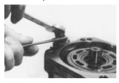
**8.** Loosen the fixing nut of the stopper max flow and disassemble it.
