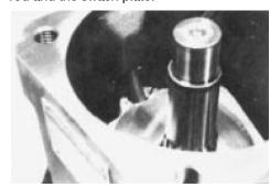
3. Pumps clockwise driven must have a position of the valve plate 4 degrees out of center in the same direction decentered like drive direction.
