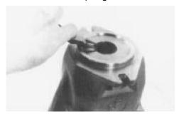
21. Disassemble the sealing ring.
