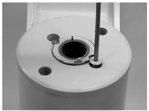
2. Using a 1/8" (3.18mm) drill bit, drill a hole in the center of each lock pin to a depth of approximately 3/16" (4.76mm).
