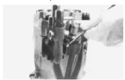
**2.** Mark the position of the port plate and remove the socket screw of the port plate.
