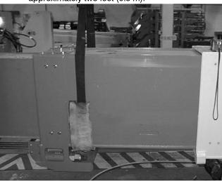
Pull out the wire ropes between the base boom and mid boom.
