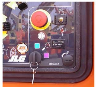
**2.** Plug the analyzer into the connector at the base of the platform control box.
