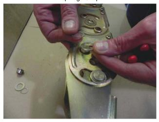
**6.** Remove the screws from the bar. Remove the snap ring and pin.
