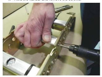
5. Remove the snap rings and pins.
