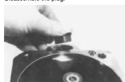
**14.** Disassemble the control piston while moving the swash plate.
