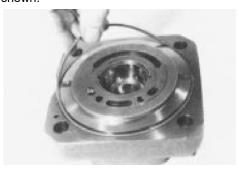
**24.** A bearing puller is used to disassemble the external bearing ring of the taper roller bearing inside the port plate. Take care of the surface of the port plate.
