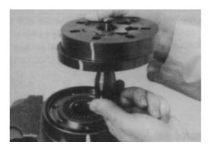
**NOTE:** Series TG Torqlinks<sup>™</sup> may have a rotor set with two stator halves (8B) with a seal ring (4) between them and two sets of seven vanes (8C). Discard seal ring only if stator halves become disassembled during the service procedures.
