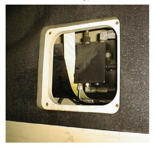
Loosen and remove the bolt that secures the retaining pin and remove the retaining pin.
