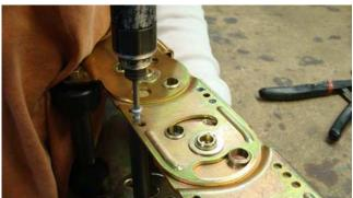
**3.** Remove the screws from the flat bar on the other side of the powertrack.
