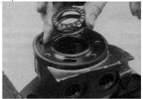
**18.** Remove seal (16) and back up washer (17) from Small Frame, housing (18). Discard both.
