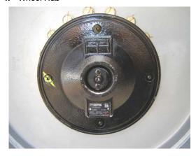
Lube Point(s) - Level/Fill Plug Capacity - 0.5 quarts (0.5 liters) ± 10% Lube - EPGL
