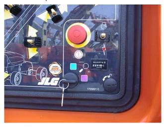
Plug the analyzer into the connector inside the Ground control box.
