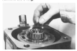
Disassemble the taper roller bearing (nearby port plate).
