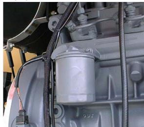
Wipe the area around the filter to clean any dirt from the area. **2.** Using a suitable oil filter removal tool, loosen the lube oil filter cartridge and spin off.
