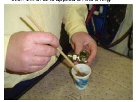
2. Holding the fitting over the hydraulic oil container, brush an even film of oil around the entire o-ring in the fitting, making sure the entire o-ring is completely saturated.
