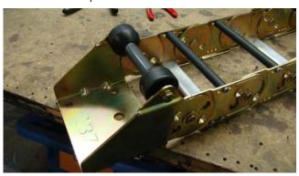
**2.** Remove the screws from the bars on one side of the powertrack on the first link.
