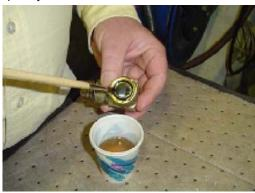
**3.** Turn the o-ring on the other side of the fitting and repeat the previous step, ensuring the entire o-ring is coated with hydraulic oil.
