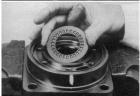
**9.** Apply a small amount of clean grease to a **new** seal ring (4) and insert it into the housing (18) seal ring groove.
