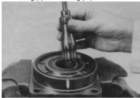
**13.** Remove thrust bearing (11) from top of coupling shaft (12). Inspect for wear, brinelling, corrosion and a full complement of retained rollers.
