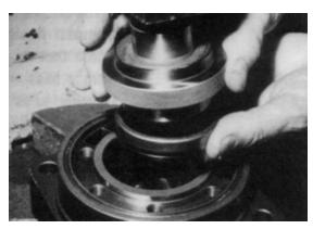
**3.** Press a **new** dirt and water seal (20) into the housing (18) outer bearing counterbore.
