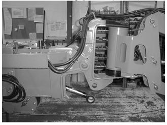
Tag and disconnect the two jib leveling cylinder hoses. Cap or plug all openings.
