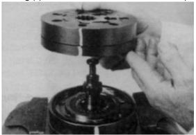
NOTE: The rotor set (8) components may become disassembled during service procedures. Marking the surface of the rotor and stator that is facing UP, with etching ink or grease pencil before removal from Torqlink™ will ensure correct reassembly of rotor into stator and rotor set intoTorqlink™.Marking all rotor components and mating spline components for exact repositioning at assembly will ensure maximum wear life and performance of rotor set andTorq-link™.
