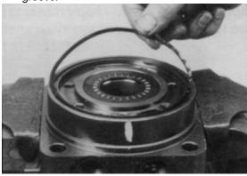
NOTE: One or two alignment studs screwed finger tight into housing (18) bolt holes, approximately 180 degrees apart, will facilitate the assembly and alignment of components as required in the following procedures. The studs can be made by cutting off the heads of either 3/8-24 UNF 2A or 5/16-24 UNF 2A bolts as required that are over 0.5 inch (12.7 mm) longer than the bolts (1) used in the Torqlink<sup>TM</sup>.
