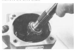
20. Disassemble the snap ring.
