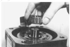
6. Remove the adjustment shim.
