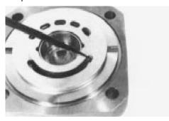
5. Note the correct position of the drilling that connects high pressure to the control valve. Check control valve drilling position at the pump housing and fit together.
