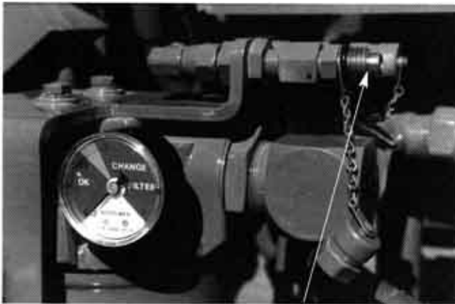
TAKE HYDRAULIC OIL SAMPLE FROM THIS PORT
