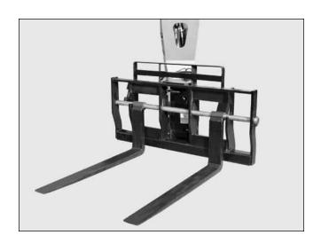
The swing carriage allows the operator to maneuver loads through openings and tight spaces by swinging the carriage to the right or left.
