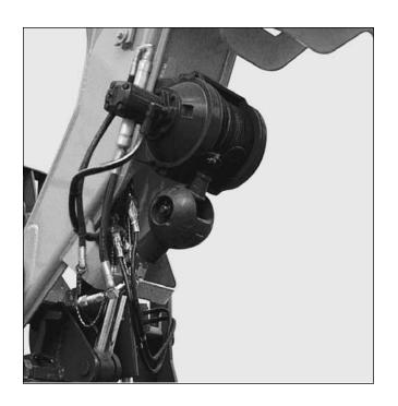
Job site performance and versatility are enhanced with the boom head mounted winch. The boom head mounted winch features (11 mm) 7/16 in IPS wire rope and can be used with or without the carriage and forks attached.
