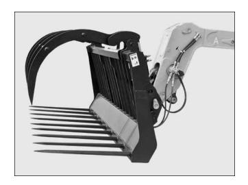
The light duty manure fork and grab is designed for loading and handling loosely-packed manure and silage in farming and agricultural applications. The grab is ideal for grasping manure and bedding materials and provides superior load penetration and reduced spillage.
