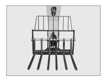
Cubing forks have a smaller width and are used to load, unload and place cubes of brick or block. Forks can be ordered in sets of four or six. A set of four is ideal for moving brick. A set of six will work better when handling concrete blocks.
