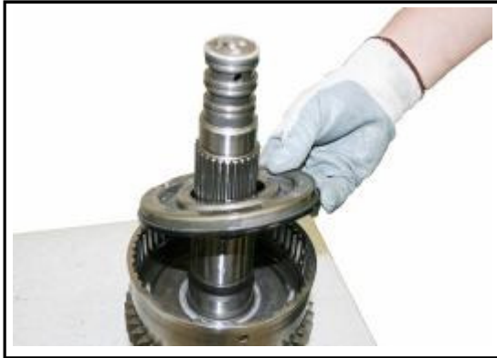
9:1 Replace the piston into the Forward High clutch housing. Lubricate the piston before reassembly
