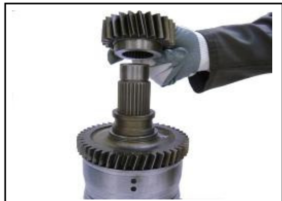
6:30 Replace the gear to the splined shaft.
