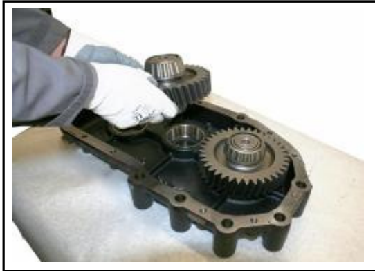
2:13 Remove the intermediate gear assembly.
