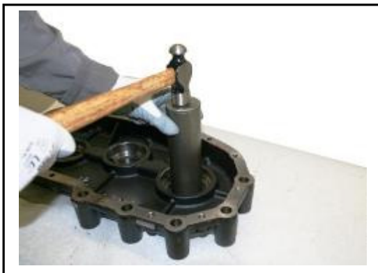
2:17 Using a suitable tool remove and discard the oil seal from the input shaft.
