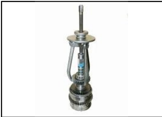
8:15 Invert the shaft and install the appropriate bearing puller to remove the gear and bearing.
