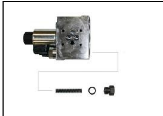
13:4 The Dual Modulating Valve with the modulation components removed.
