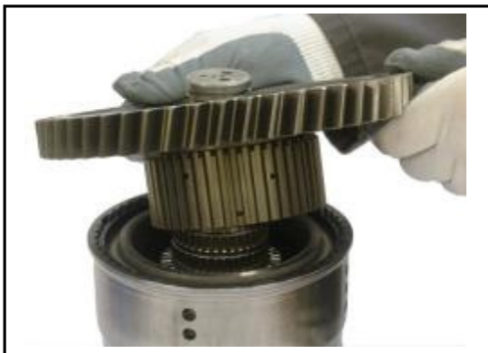
6:11 Replace the hub gear to the 1st clutch pack.
