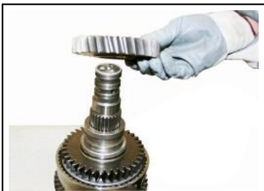
8:17 Remove the gear from the forward High clutch
