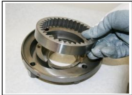
12:4 Remove the pump annulus gear
