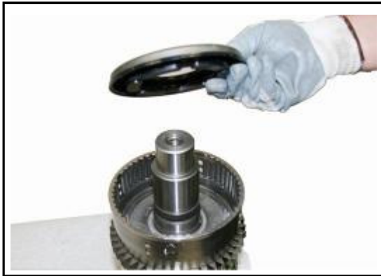
8:13 Remove the piston assembly
