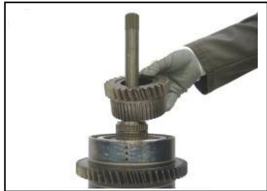
11:10 Replace the Reverse clutch hub gear.
