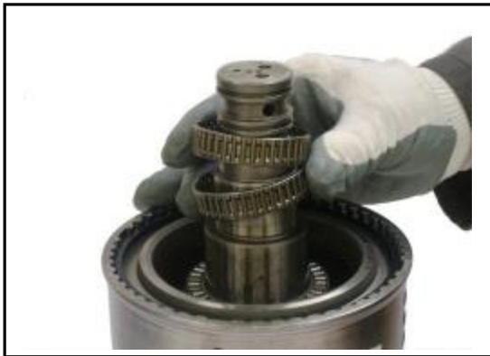
5:21 Remove the hub gear support bearings from the 1st clutch pack.
