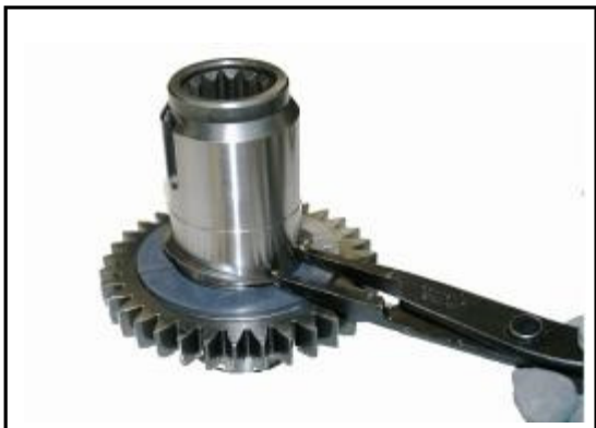
14:17 Fit the lower thrust disc snap ring.
