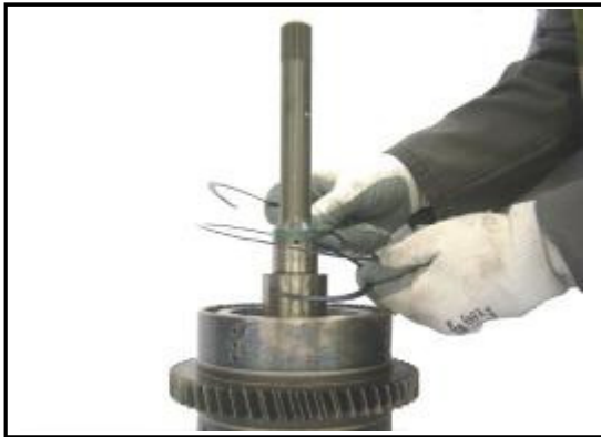
11:7 Replace the double snap ring to the Reverse clutch housing.
