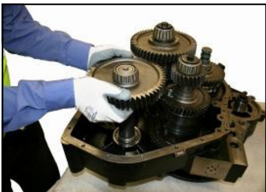
4:15 Using suitable lifting equipment remove the rear transmission case. Lever slots are provided to assist removal. Caution! The bearing Cups and shims may fall from the case during removal
