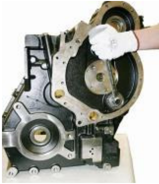
4:57 With the gear locked onto the bolt on the shaft. Remove the Bolt and washer.
