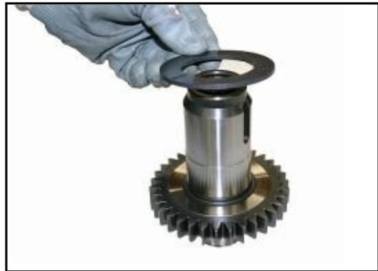
14:16 Replace the lower thrust disc to the pump drive shaft assembly
