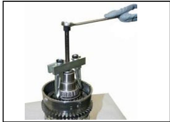
8:8 Install the appropriate bearing puller to remove the 3rd clutch internal bearing.
