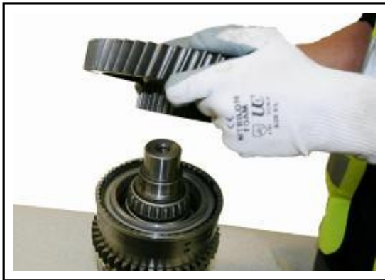
9:27 Fit the hub gear to the 3rd clutch housing.
