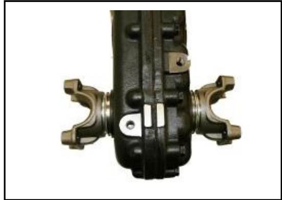
3:20 Install the front and rear drive yokes.
