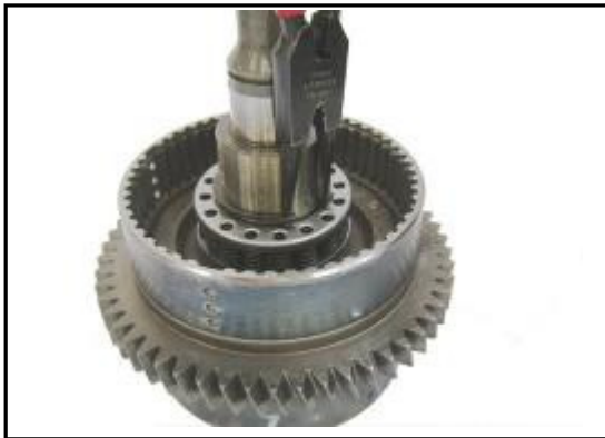
11:3 Loosely fit the circlip to the shaft and push down onto the spring pack.
