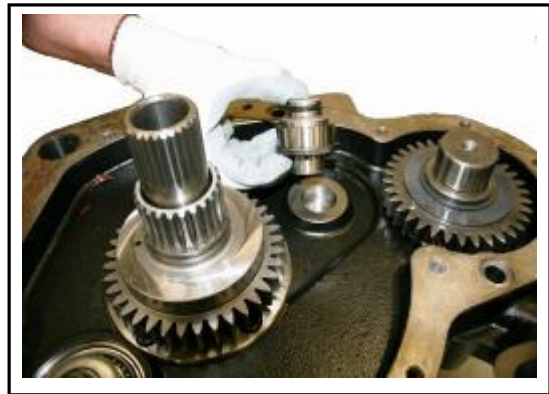
14:22 Replace the support shaft & bearing assembly into the front casing.
