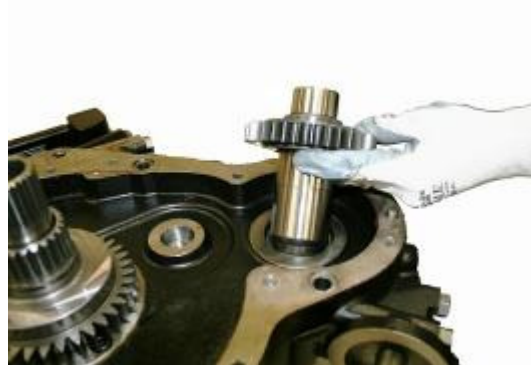
4:44 Lift out the Pump drive shaft assembly
