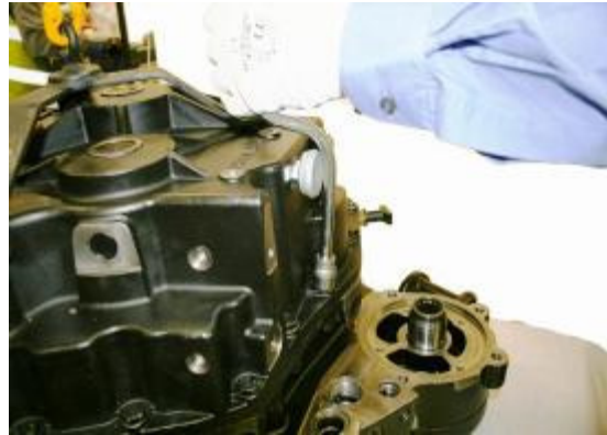
4:14 Remove the 20 Screws securing the casing.
