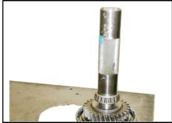
6:32 Using a suitable tube carefully drive the bearing fully onto the shaft
