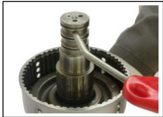
5:28 Using an air line with a low pressure supply pressurise the 1st Clutch to remove the piston from the clutch housing.
