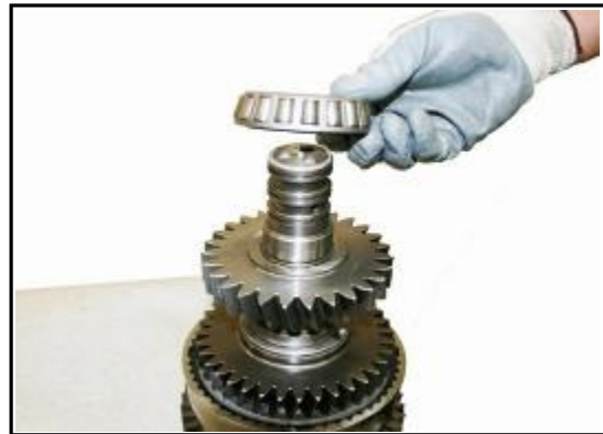
8:16 Remove the bearing from the forward High clutch
