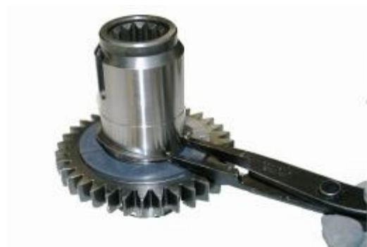
4:47 Invert the Pump drive shaft and remove the bottom snap ring.
