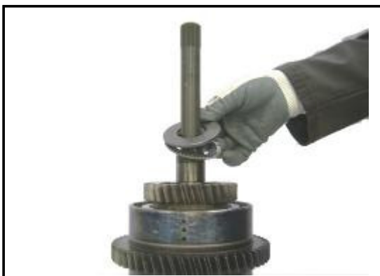
11:11 Replace the outer thrust washer and bearing.
