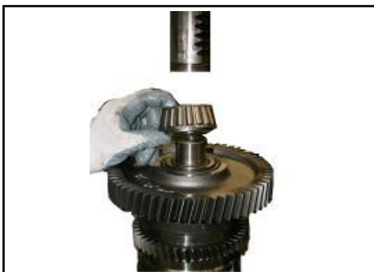
9:29 Use a suitable tube or press drive the upper bearing onto the shaft.
