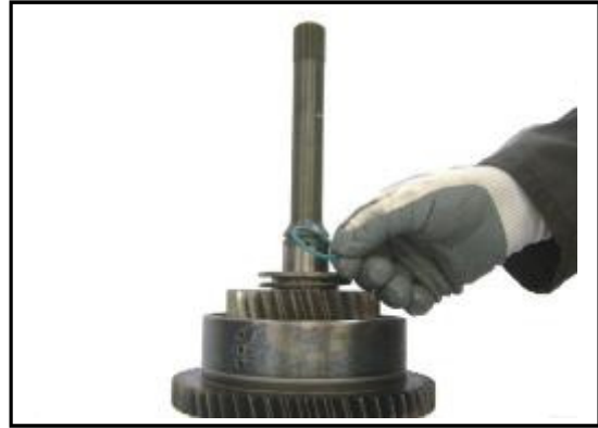
10:25 Remove and discard the seal from the shaft.
