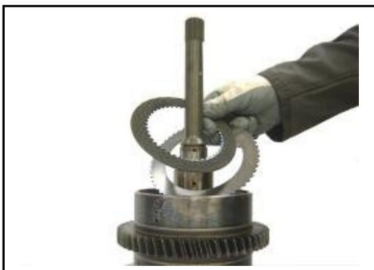
11:5 Refit the counter and friction plates to the clutch assembly. Note! The counter plate is placed adjacent to the piston
