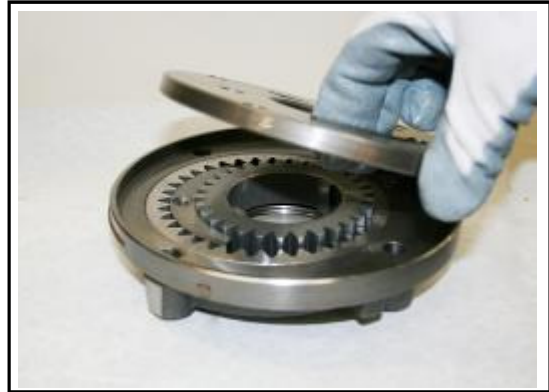
12:2 Remove the pump back plate
