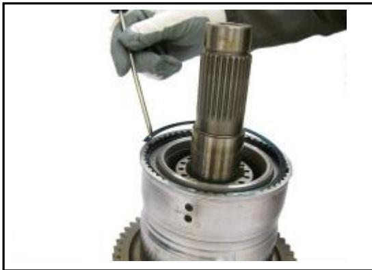
5:9 Using an appropriate tool remove the double snap ring from the 2nd clutch pack.
