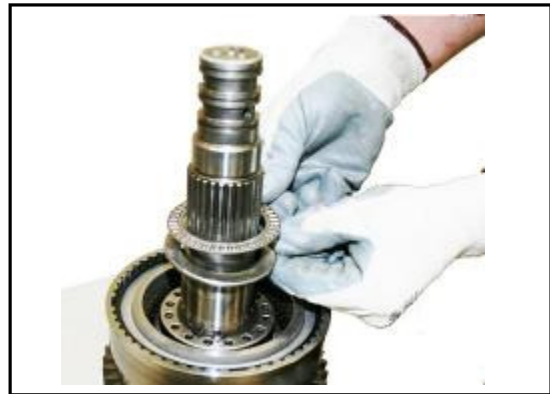
8:22 Remove the Two thrust bearings
