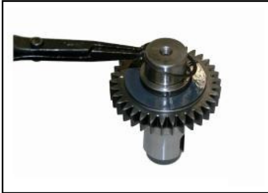
14:19 Fit the upper snap ring to the Pump drive shaft assembly
