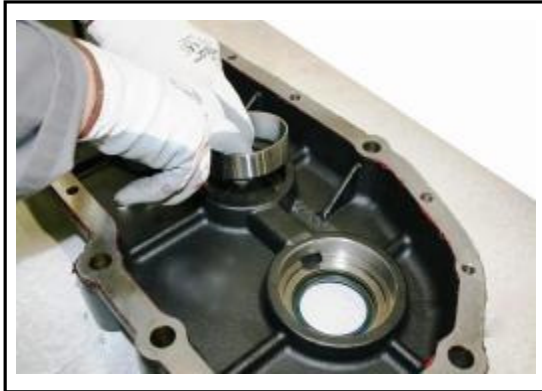
2:15 Remove & retain the bearing cups and shims from the rear casing & the bearing cups from the front case.
