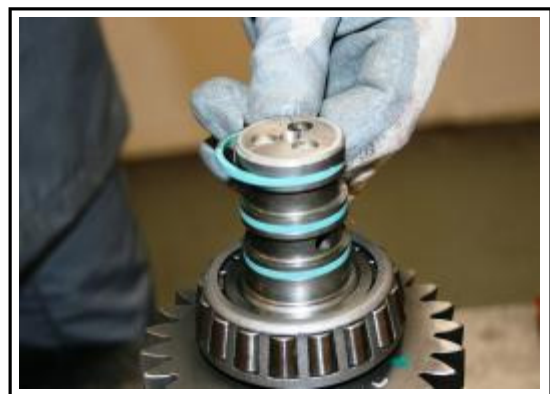
9:30 Carefully install the 3 sealing rings to the end of the shaft.
