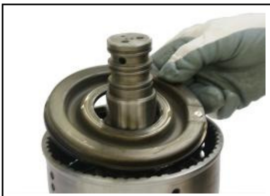
5:29 Remove the piston from the clutch housing.
