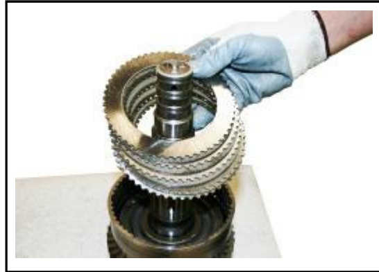
9:2 Replace the counter and friction plates. Ensure the counter plate is placed against the piston.
