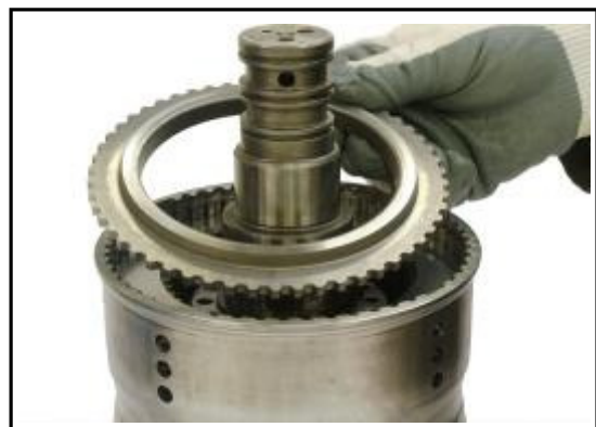
6:6 Replace the retainer plate.
