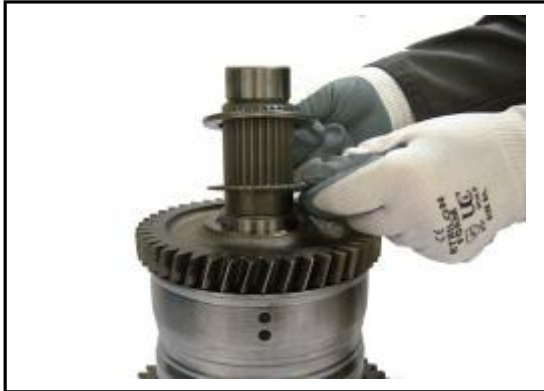
6:27 Replace the outer thrust washer and bearing.
