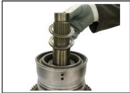
5:8 Remove the inner thrust washer and bearing.
