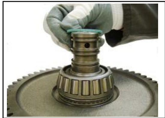
5:16 Remove and discard the 3 sealing rings from the end of the shaft.
