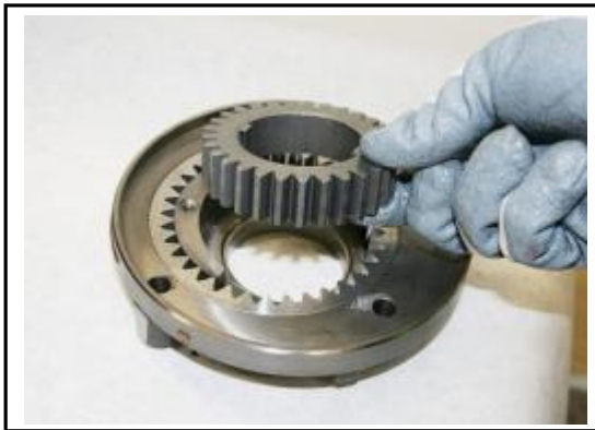
12:3 Remove the pump hub gear
