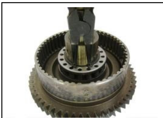
11:17 Loosely install the circlip onto the shaft and push down onto the spring pack.
