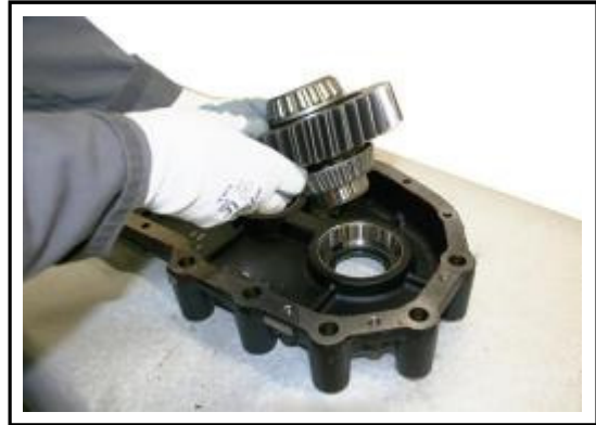
2:14 Remove the Input gear assembly.
