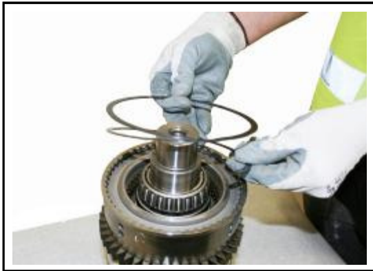
9:25 Replace the double snap ring from the 3rd Clutch
