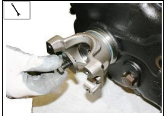
3:22 Install the retaining bolts and washers to each yoke. Tighten to the correct torque. 63 - 88 Nm ( 50 - 65 lb ft)
