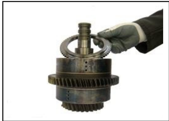
10:10 Lift out the Clutch pack retaining plate.
