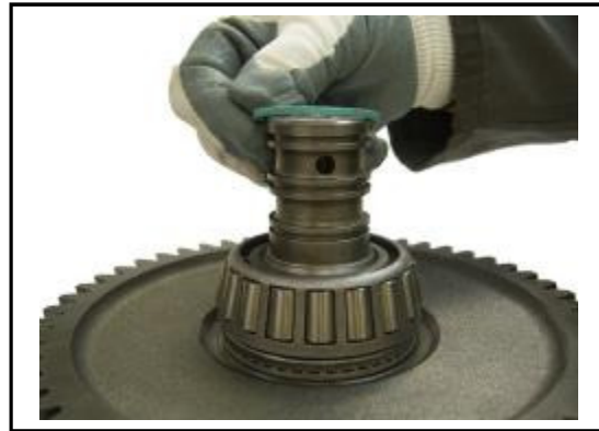
8:14 Remove and discard the 3 sealing rings from the end of the shaft.
