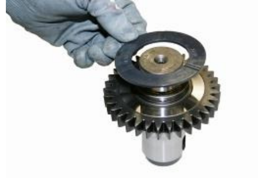
4:46 Remove the top Thrust Disc
