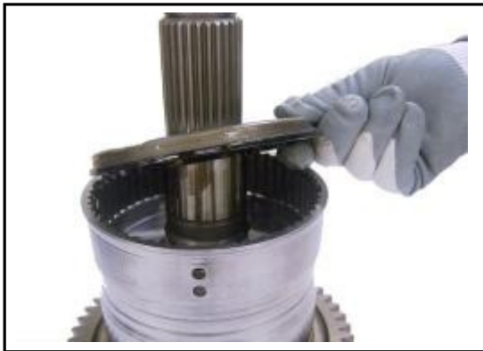
5:15 Remove the piston from the clutch housing.
