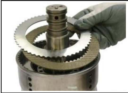
5:25 Remove the clutch counter plates and friction plates.
