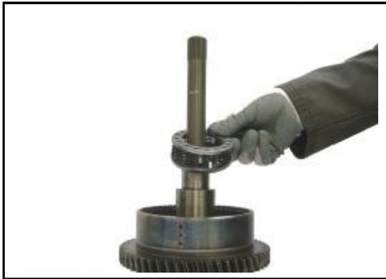
10:30 Lift out the spring pack assembly.
