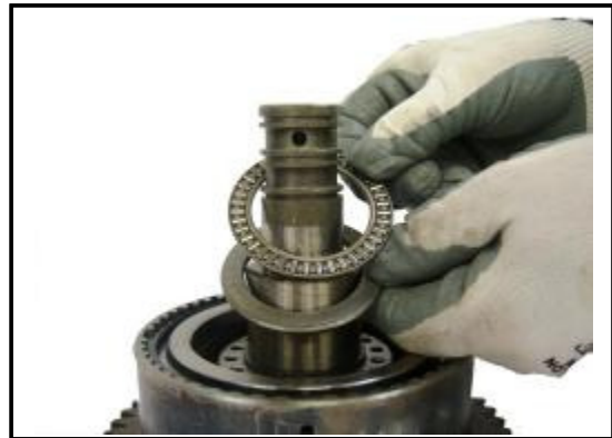
11:22 Replace the inner thrust washer and bearing
