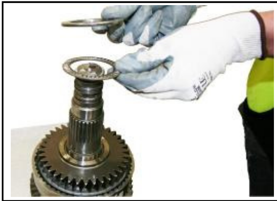
8:19 Remove the Two thrust bearings
