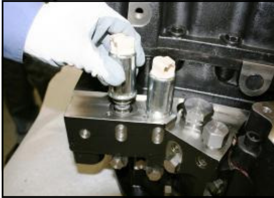
4:7 Prise out the Solenoid valve assemblies from the Transmission Casing
