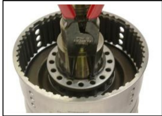
5:26 Push down on the spring pack and using a suitable tool remove the circlip.
