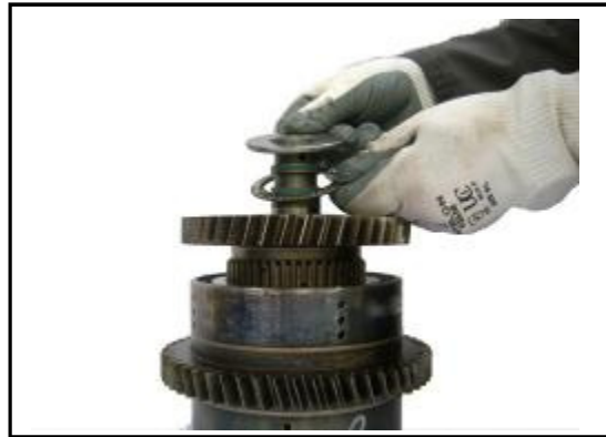
11:26 Replace the outer thrust washer and bearing
