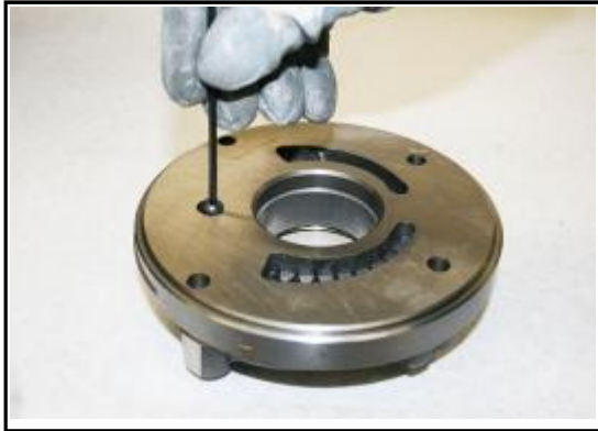
12:1 Remove the single screw from the pump back plate
