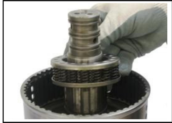
6:2 Replace the spring pack assembly into the 1st clutch housing.
