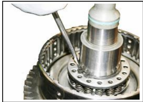
6:4 Use a flat blade screwdriver or other suitable tool to push down on the Circlip until the spring pack is compressed sufficiently for the Circlip to snap into the groove.
