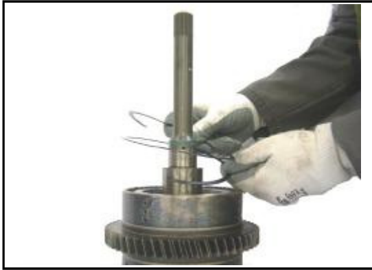
10:24 Remove the double snap ring from the Reverse clutch.
