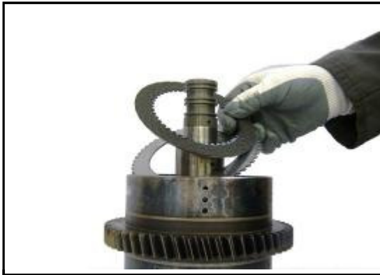
11:19 Replace the counter and friction plates. Note! The counter plate is placed against the piston.
