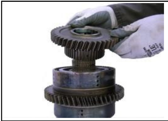
11:25 Replace the Forward Low clutch Hub gear
