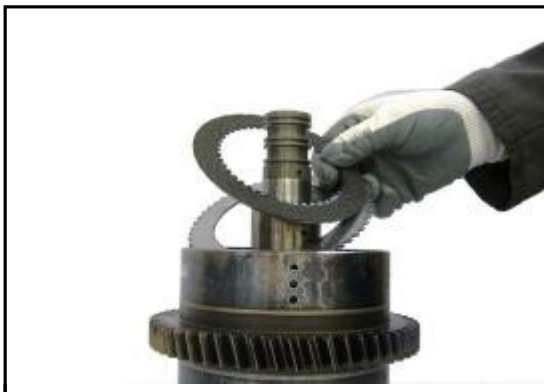
10:11 Remove the counter and friction plates. Note! The counter plate is placed against the retainer.
