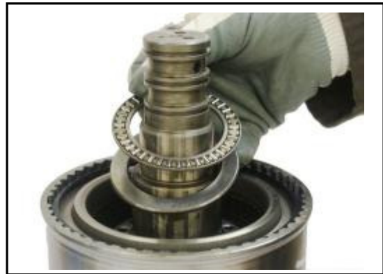
5:22 Remove the inner thrust washer and bearing.
