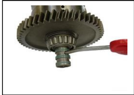
5:14 Using an air line with a low pressure supply pressurise the 2nd Clutch to remove the piston from the clutch housing.
