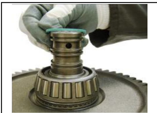
11:29 Replace the 3 sealing rings to the shaft
