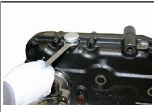
3:23 Reinstall the breather assembly to the casing.
