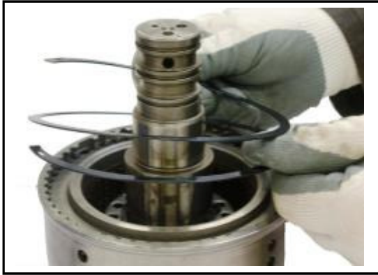
6:7 Replace the double snap ring into the 1st clutch pack.
