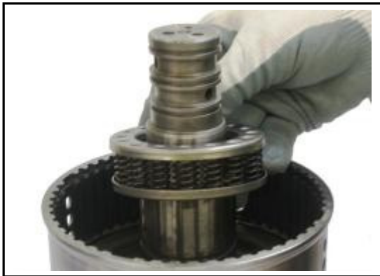
5:27 Remove the spring pack assembly from the 1st clutch housing.
