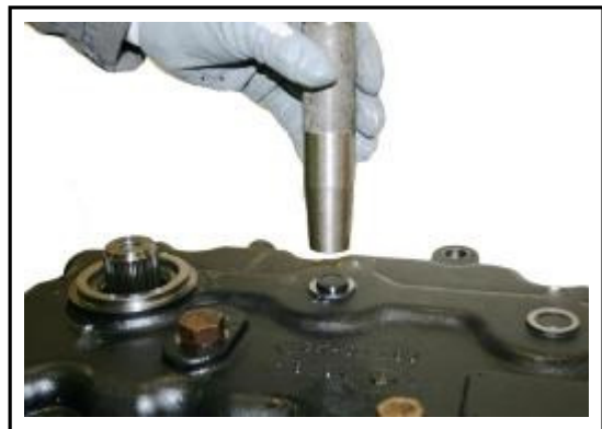
3:18 Insert replacement shimming plugs to each shaft.
