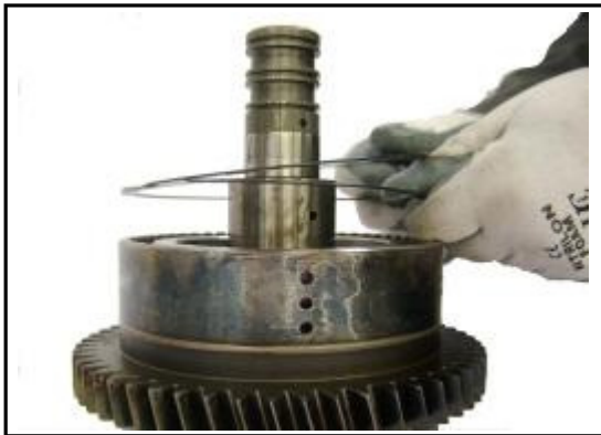
11:21 Replace the double snap ring to the Forward Low clutch.
