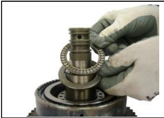
10:7 Remove the inner thrust washer and bearing
