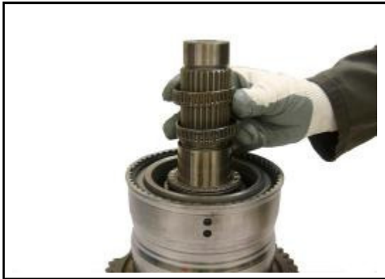
5:7 Remove the hub gear support bearings from the 2nd clutch pack.
