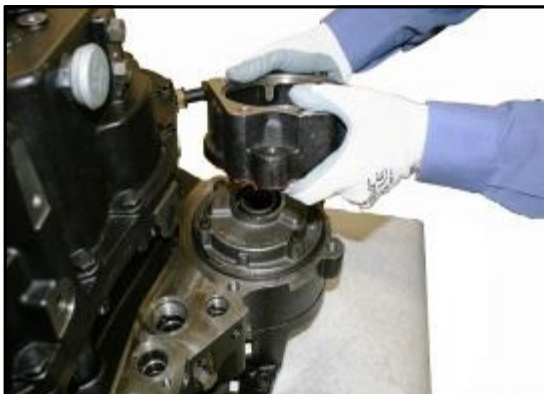
4:11 Lift the Pump housing away from the pump.
