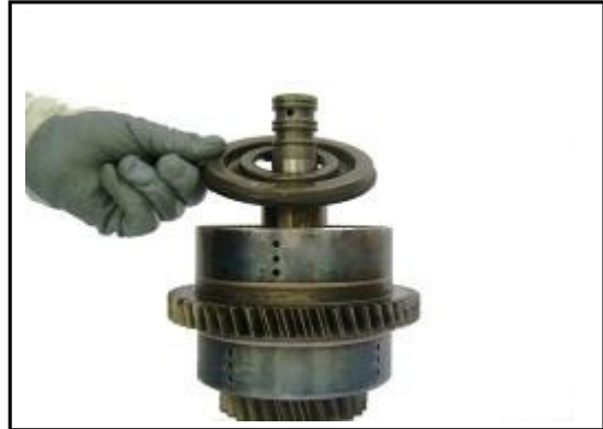
10:16 Remove the Piston from the cylinder
