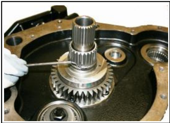
14:15 Re-install the pump drive gear O ring.
