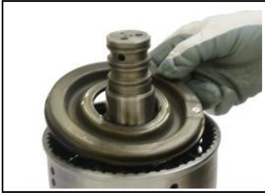
6:1 Replace the piston into the 1st clutch housing. Lubricate the piston before reassembly
