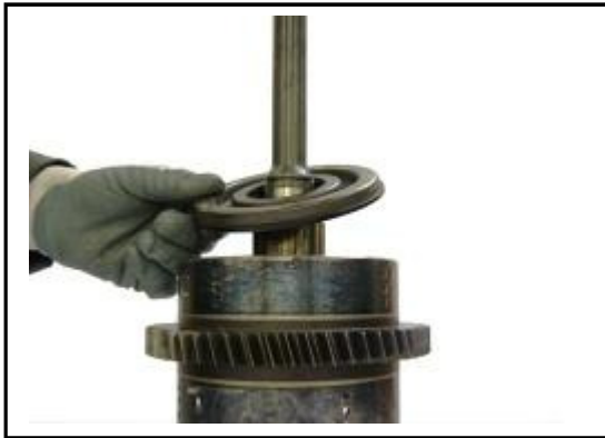
11:1 Replace the Piston to the Reverse clutch cylinder. Lubricate the piston before reassembly
