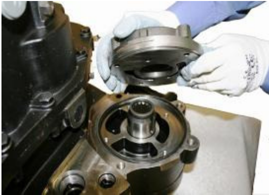
4:13 Remove the Pump assembly from the transmission and recover the O ring seal
