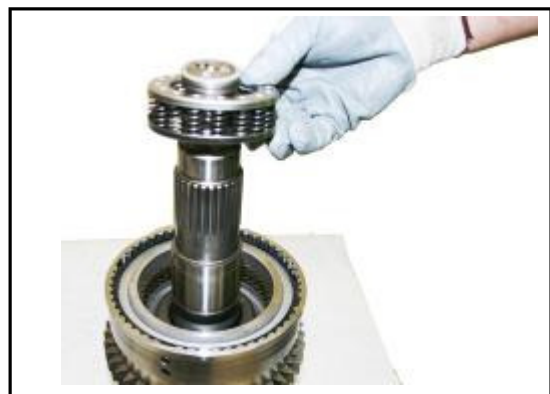
8:24 Remove the spring pack assembly
