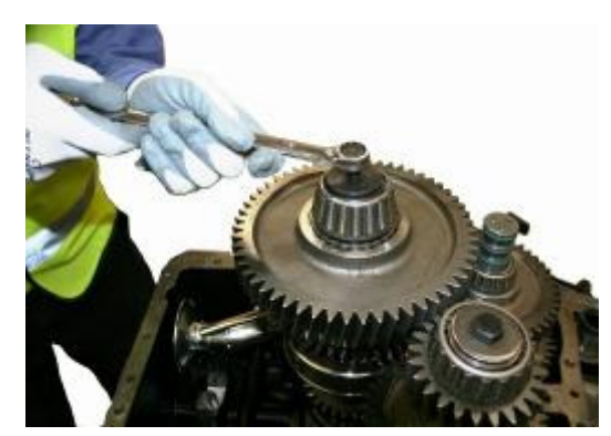
4:18 Remove the Screw and Washer from the end of the Forward High / Third clutch shaft.
