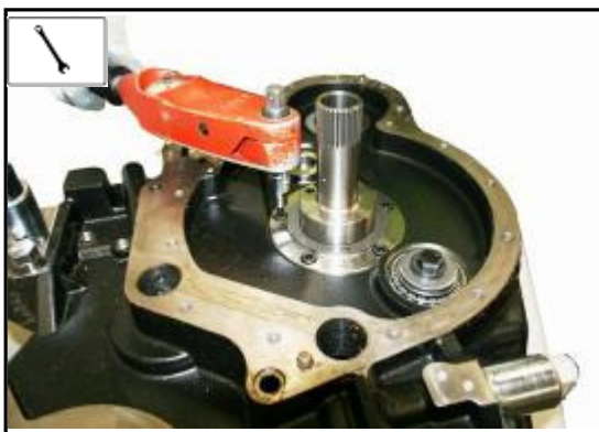
14:11 Tighten the retaining capscrews to the required torque. 18 - 31 Nm (13 -23 lb ft)
