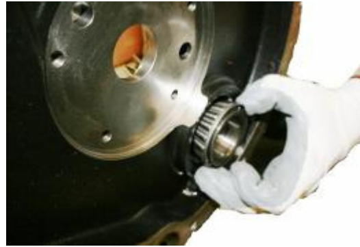
4:58 Remove the bearing from the front casing.
