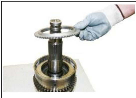
9:3 Refit the Clutch pack retaining plate.
