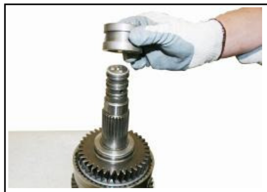
8:18 Remove the spacer from the forward High clutch
