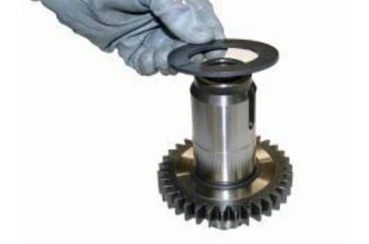
4:48 Remove the bottom Thrust Disc
