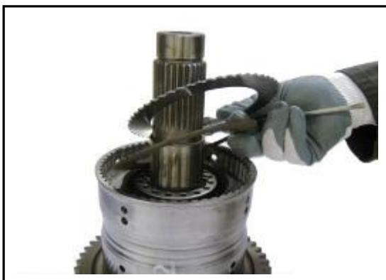
5:11 Remove the clutch counter plates and friction plates.
