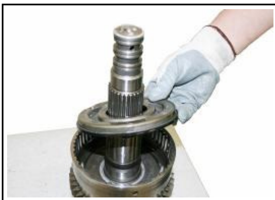
8:29 Remove the piston from the clutch housing.
