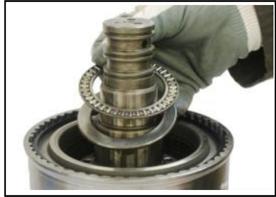
6:8 Replace the inner thrust washer and bearing.
