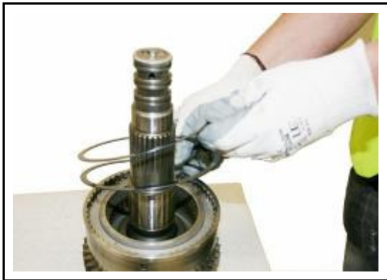
9:9 Replace the double snap ring to the Forward High clutch pack.
