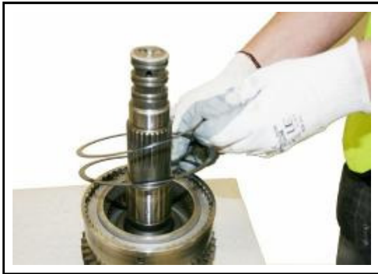
8:25 Remove the double snap ring from the Forward High clutch pack.
