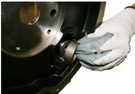
4:59 Remove the bearing spacer from the front casing.
