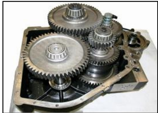
4:16 The Transmission with the rear casing removed.
