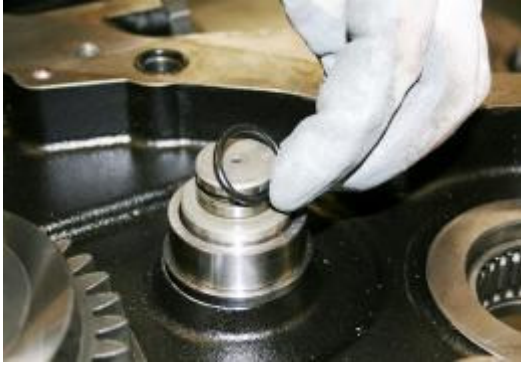
4:43 Remove the O ring from the support shaft.
