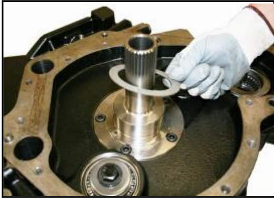
14:13 Replace the Pump drive gear thrust washer.
