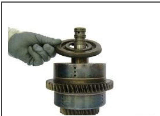
11:15 Fit the Piston to the Forward Low clutch cylinder Lubricate the piston before reassembly
