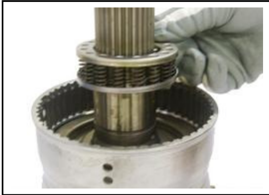
5:13 Remove the spring pack assembly from the 2nd clutch housing.
