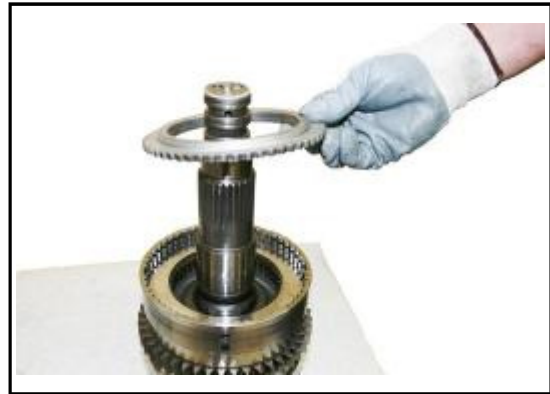
8:26 Lift out the Clutch pack retaining plate.
