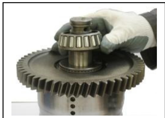
5:18 Remove the bearing from the shaft.
