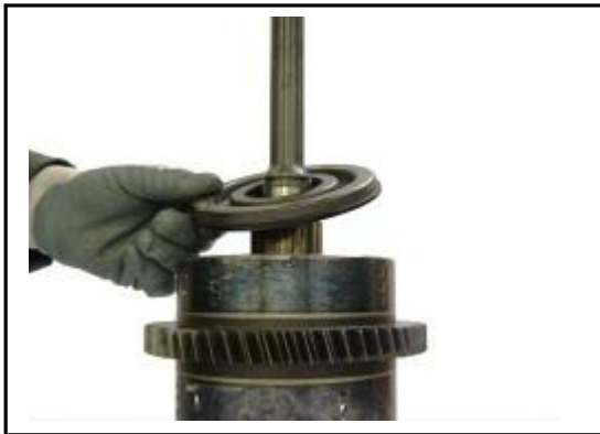
10:32 Remove the Piston from the cylinder
