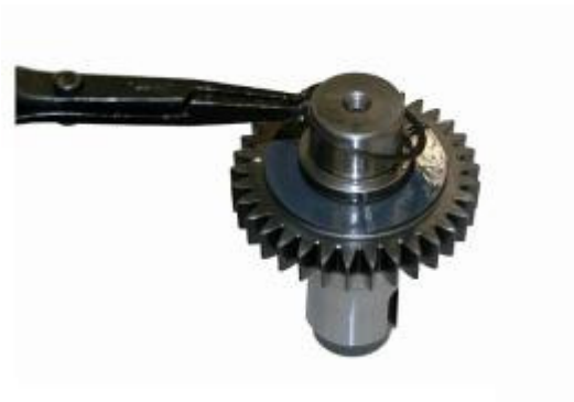
4:45 Remove the top snap ring from the Pump drive shaft assembly
