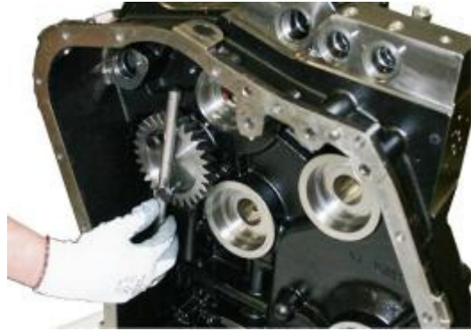
4:56 Remove the Reverse idler gear. Insert two suitable pins into the holes in the gear and lock the gear into position.
