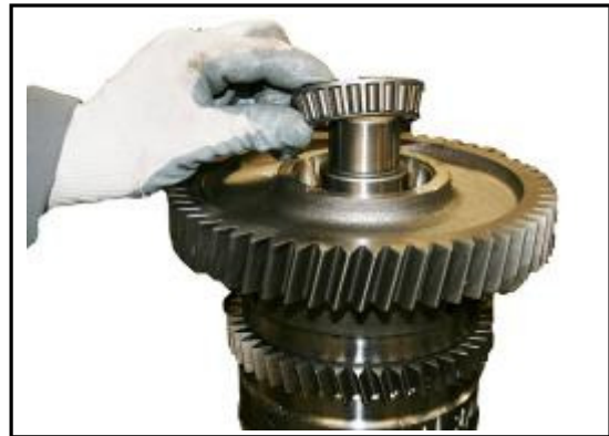
9:28 Replace the bearing to the 3rd clutch gear
