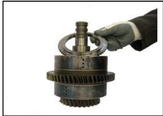
11:20 Refit the Clutch pack retaining plate.
