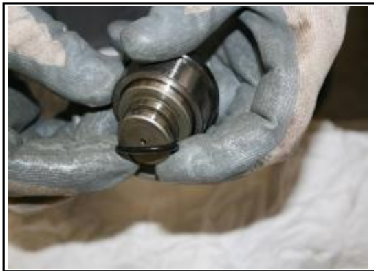
14:21 Replace the O ring to the support shaft assembly
