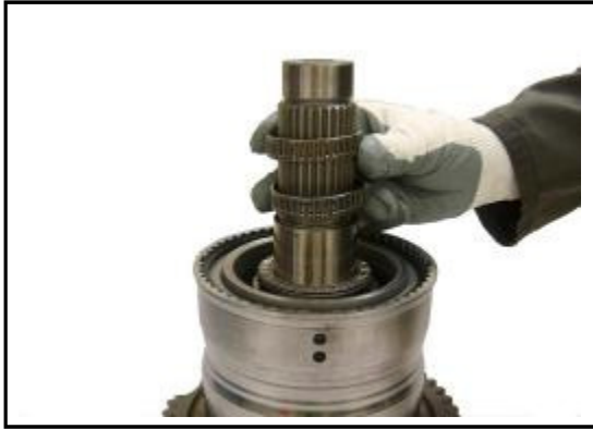
6:25 Replace the hub gear support bearings to the 2nd clutch pack.
