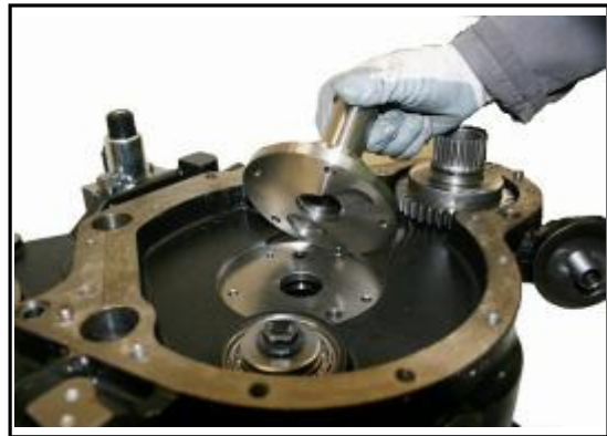
14:10 Clean the mating surfaces and replace the Stator support hub to the front casing.
