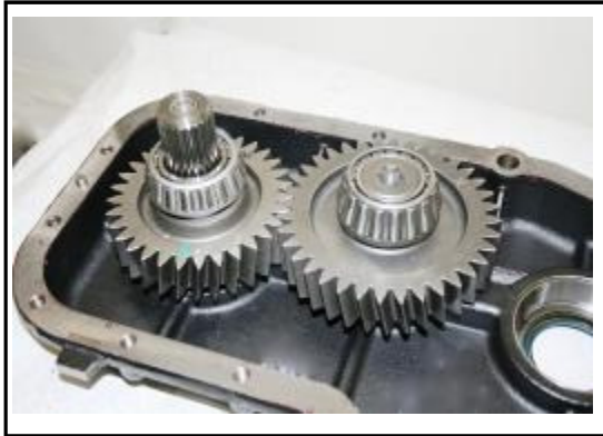
3:13 Reinstall each of the gear shafts
