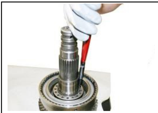
9:5 Loosely install the Circlip onto the shaft. The circlip has a flat face ensure this is placed facing upwards.
