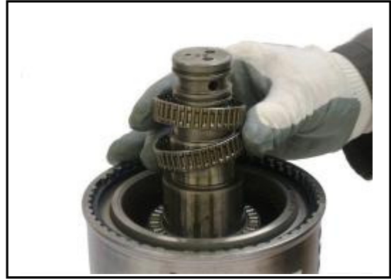
6:10 Replace the hub gear support bearings for the 1st clutch pack.
