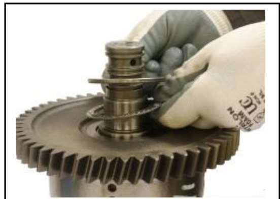
6:12 Replace the outer thrust washer and bearing.
