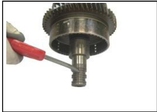
10:31 Using an air line with a low pressure supply pressurise the Reverse Clutch to remove the piston from the clutch housing.
