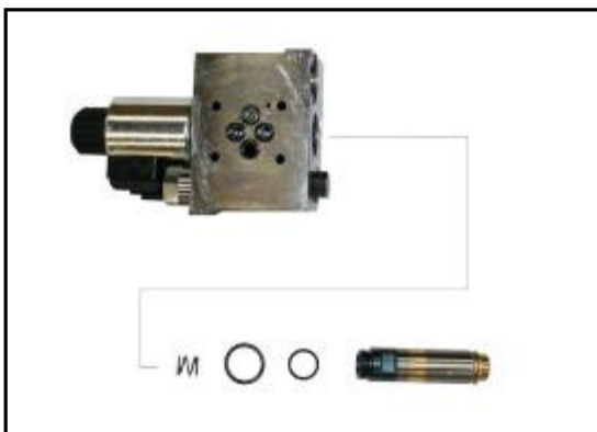
13:5 The Dual Modulating Valve with the Solenoid spool and O ring seals removed.
