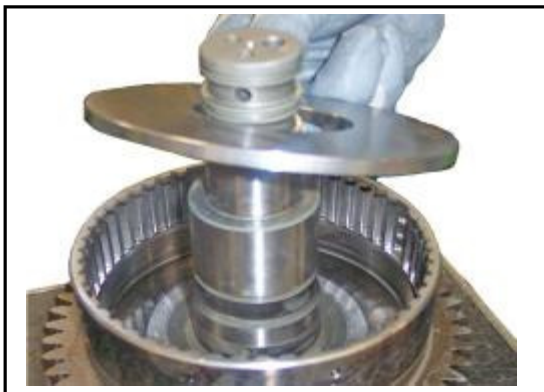
10:17 Remove the Piston Spacer from the cylinder
