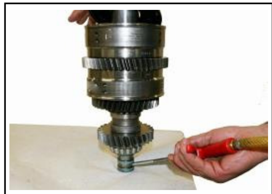
8:12 Using an air line with a low pressure supply pressurise the 3rd Clutch to remove the piston from the clutch housing.
