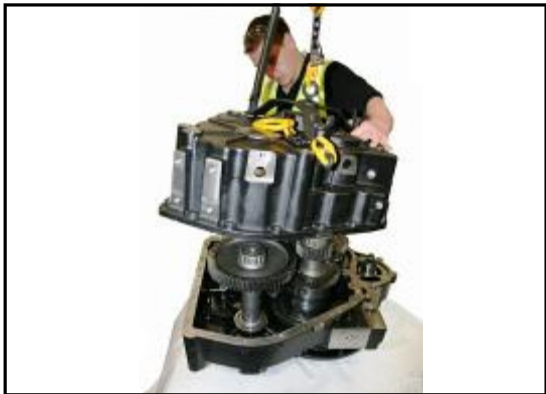
4:15 Using suitable lifting equipment remove the rear transmission case. Lever slots are provided to assist removal. Caution! The bearing Cups and shims may fall from the case during removal
