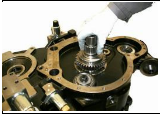
14:14 Replace the Pump drive gear.
