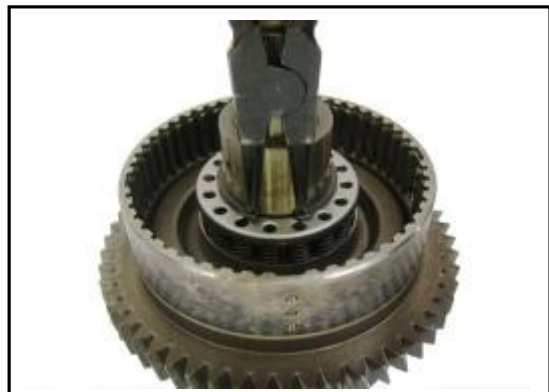
10:12 Push down on the spring pack and remove the circlip.
