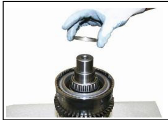
9:26 Replace the spacer to the shaft.
