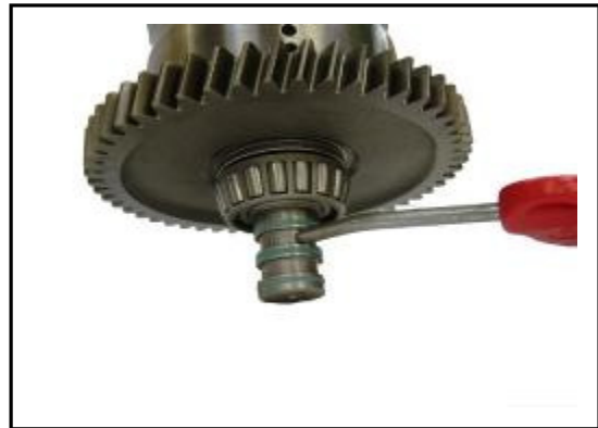
8:28 Using an air line with a low pressure supply pressurise the Forward High Clutch to remove the piston from the clutch housing.
