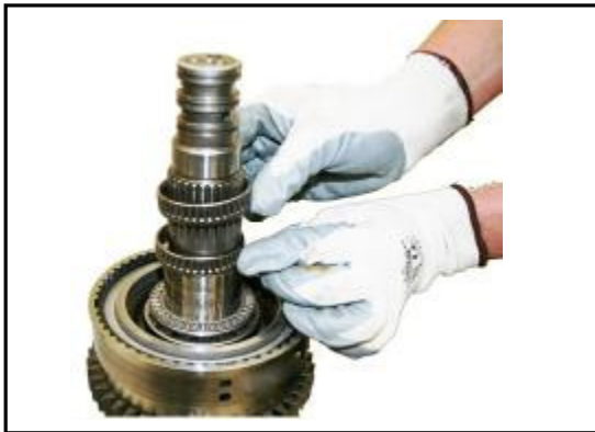
8:21 Remove the Two support bearings
