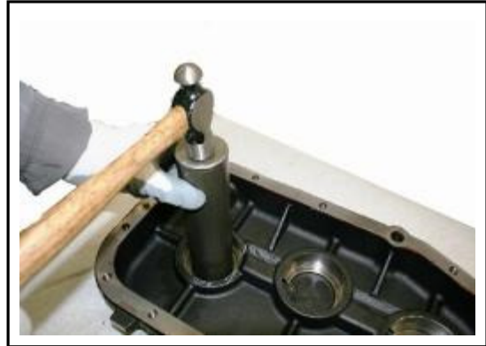
2:16 Using a suitable tool remove and discard the oil seal from the output shaft. Repeat for the front case.
