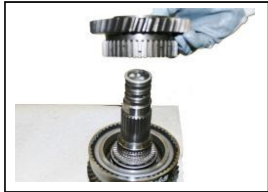
8:20 Remove the gear from the Forward High clutch
