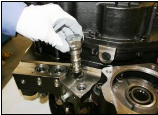
4:9 Remove the Main Pressure regulator valve cartridge
