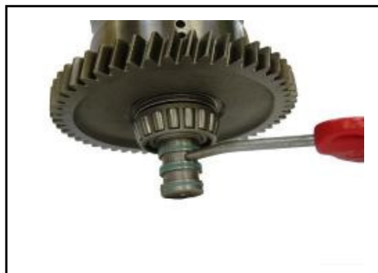
11:30 Using an air line with a low pressure supply pressurise the clutches to test operation.
