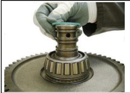
6:33 Carefully install the 4 seal rings to the shaft.
