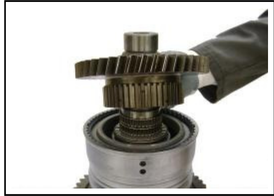
6:26 Replace the hub gear to the 2nd clutch pack.
