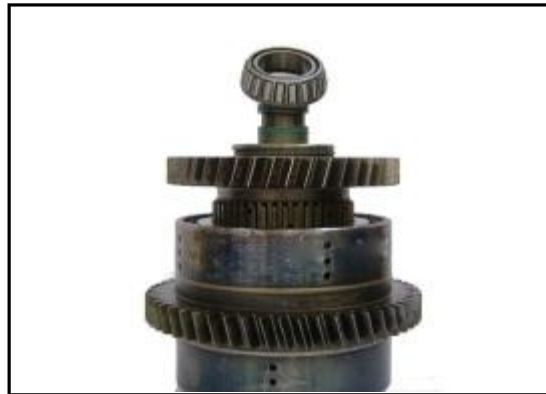
11:28 Using a suitable tool refit the bearing to the Forward Low clutch shaft.
