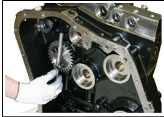
14:8 Insert Two suitable pins to lock the gear into position.
