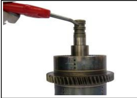
10:15 Using an air line with a low pressure supply pressurise the Forward Low Clutch to remove the piston from the clutch housing.
