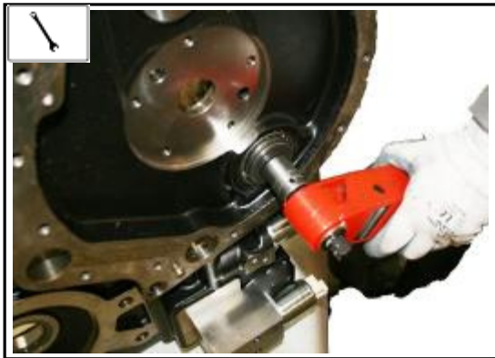
14:9 Tighten the retaining bolt to the required torque. 66-88 Nm (50—65 lb ft)
