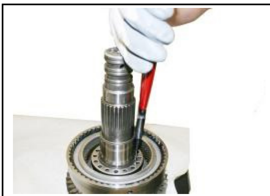
8:23 Push down on the spring pack and remove the circlip.
