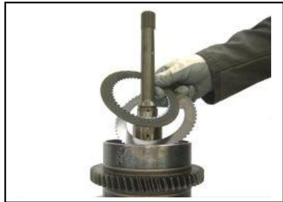
10:27 Remove the counter and friction plates. Note! The counter plate is placed against the retainer.
