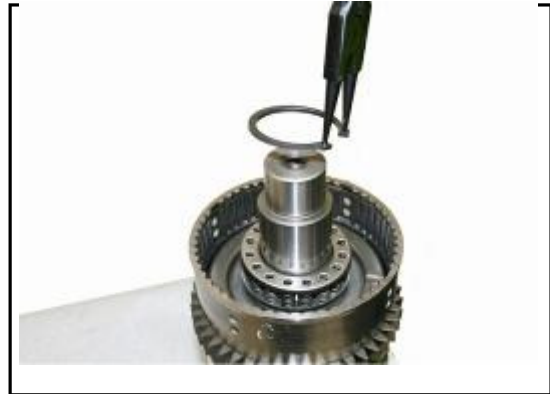
8:10 Push down on the spring pack and remove the circlip.
