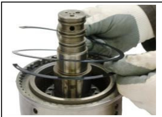
5:23 Using an appropriate tool remove the double snap ring from the 1st clutch pack.
