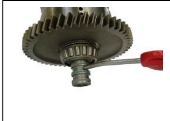
6:34 Using an air line with a low pressure supply pressurise the clutches to test operation..
