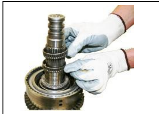
9:10 Replace the Two hub gear support bearings
