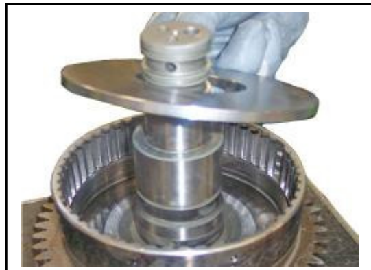
11:14 Invert the shaft and replace the Piston spacer to the Forward Low clutch cylinder Lubricate the piston before reassembly
