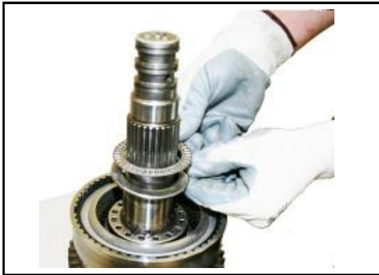
9:7 Replace the inner thrust washer and bearing.
