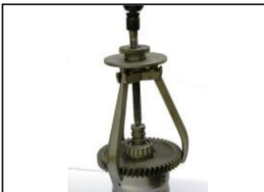
5:17 Invert & support the 1st / 2nd clutch shaft and install the appropriate bearing puller to remove the gear and bearing from the 1st clutch.
