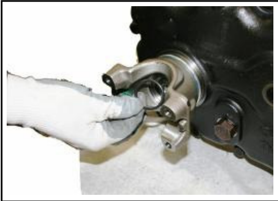
3:21 Install O ring seals to each yoke
