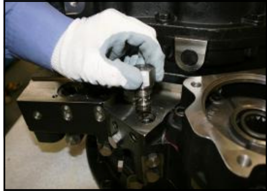
4:8 Remove the Relief valve cartridge
