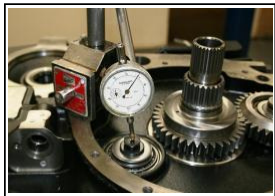
14:12 Fit a Dial test indicator and check the preload / endfloat of the reverse idler gear. -0.0508 to +0.0254mm (-0.002" to +0.001") Repeat steps 14:4 to 14:9 Inserting shims as required until correct.
