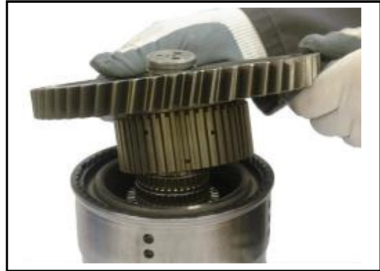
5:20 Withdraw the hub gear from the 1st clutch pack.
