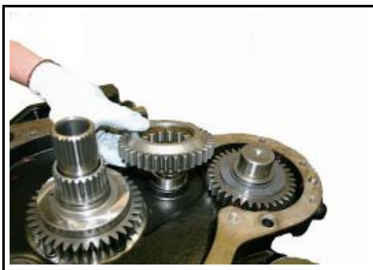
14:23 Refit the Pump idler gear to the support shaft. Check that the bearing retaining circlip is on the underside.
