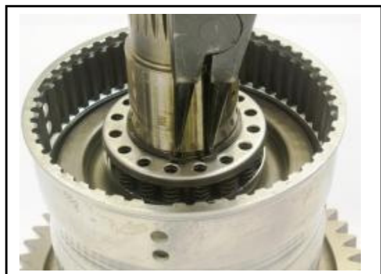
5:12 Push down on the spring pack and using a suitable tool remove the circlip.
