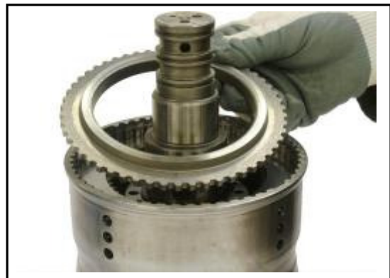
5:24 Remove the retainer plate.
