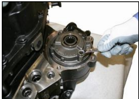
4:12 Remove the 4 Bolts that secure the pump to the Main transmission casing
