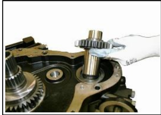
14:20 Refit the Pump drive shaft assembly
