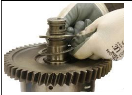
5:19 Remove the outer thrust washer and bearing.
