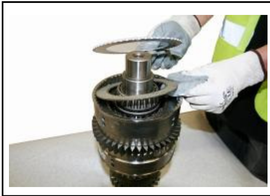
8:7 Remove the counter and friction plates. Note! The counter plate is placed against the retainer.
