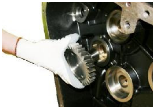
4:60 Remove the Reverse Idler gear.
