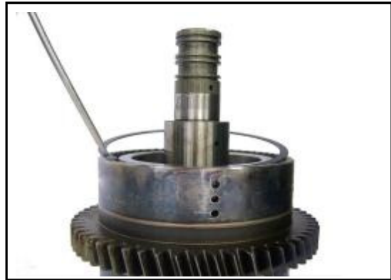
10:8 Use a suitable tool to carefully prise the snap ring from its retaining groove.
