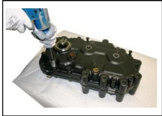
3:14 Fit the front casing and tighten the bolts equally to the correct torque.
