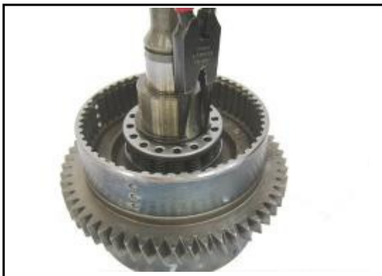
10:28 Push down on the spring pack and remove the circlip.
