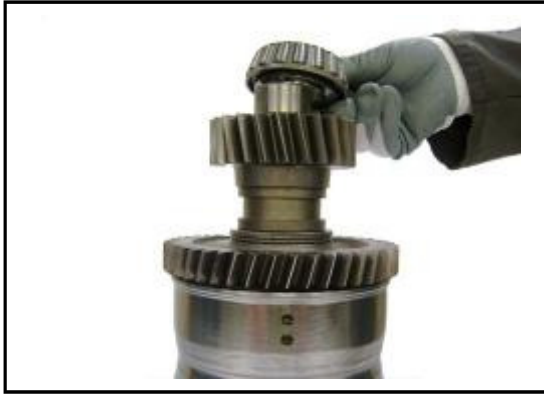
6:31 Reinstall the bearing to the shaft.
