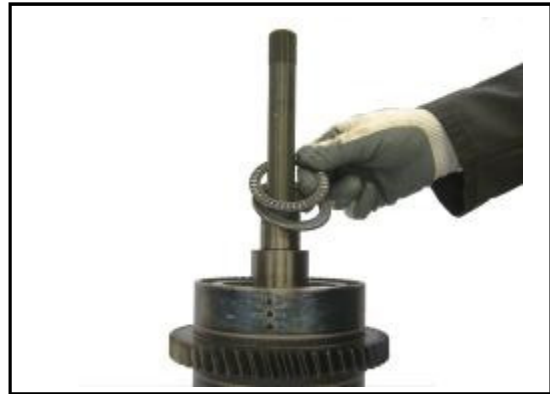
11:8 Replace the inner thrust washer and bearing.
