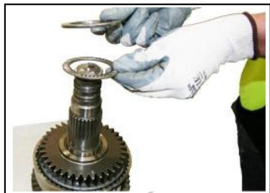
9:12 Replace the outer thrust washer and bearing.
