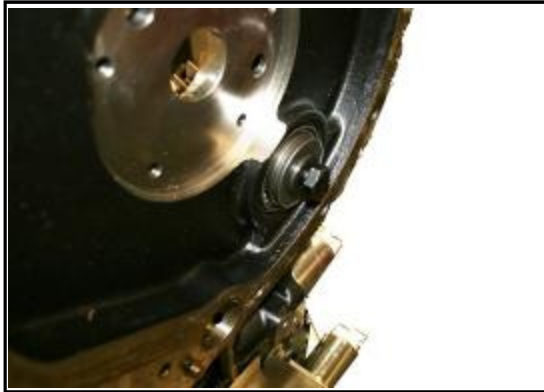
14:7 Install the Thrust plate and retaining bolt.
