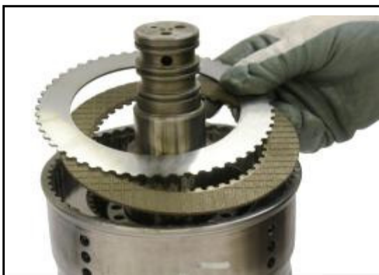
6:5 Replace the Friction and Counter plates into the clutch housing. Ensure the counter plate is installed first adjacent to the piston.
