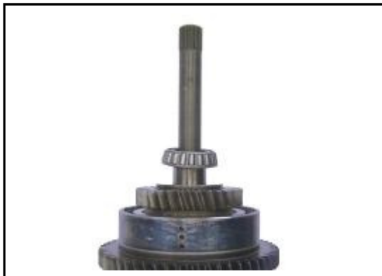
11:13 Use a suitable tube and install the bearing to the shaft.
