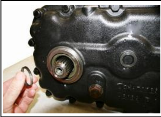
3:19 Install the spacers to the front and rear shafts.
