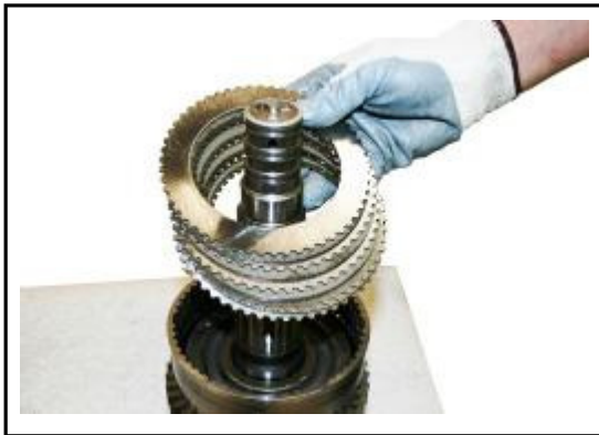
8:27 Remove the counter and friction plates. Note! The counter plate is placed against the retainer.
