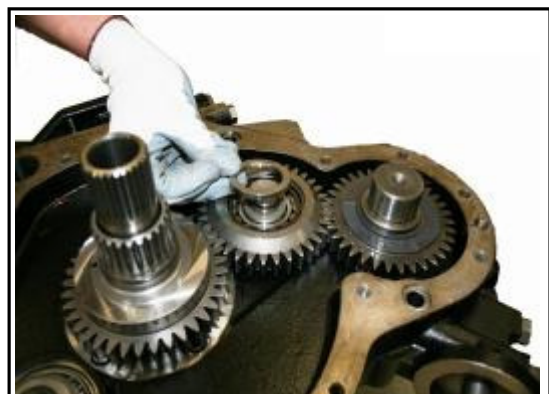
14:24 Refit the Spacer to the Pump idler gear
