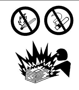
Gases from a battery can explode. Keep any open flames or sparks away from the top of a battery. Do not smoke in battery charging areas.
