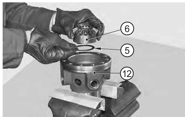
FIGURE 12: Remove tool T1 (See drawing T1 p. 131) and remove the last two planetary gears (7), the 2nd differential side gear (6) and the relative shim washer (5) from the differential carrier.
