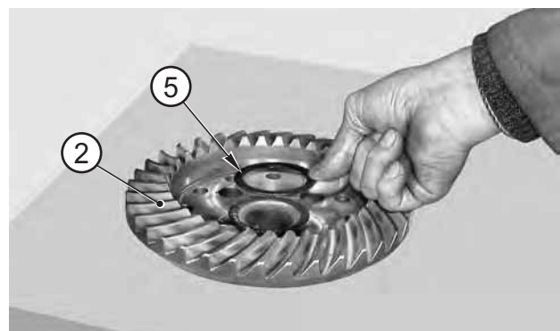
FIGURE 24: Position the shim washer (5) on the crown (2).
