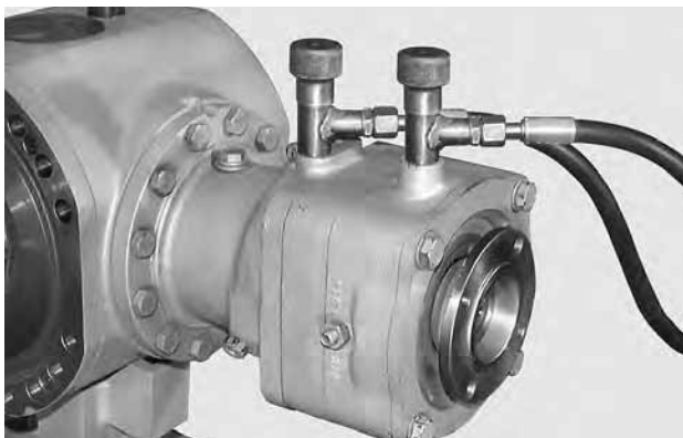
FIGURE 47: 3-FUNCTION VERSION ONLY Connect the service and negative brakes to an external pump; introduce pressure up to a value of 20 - 25 N·m.
