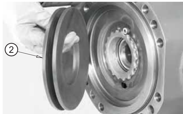
FIGURE 10: Remove the Belleville washers (2) and write down direction of assembly.
