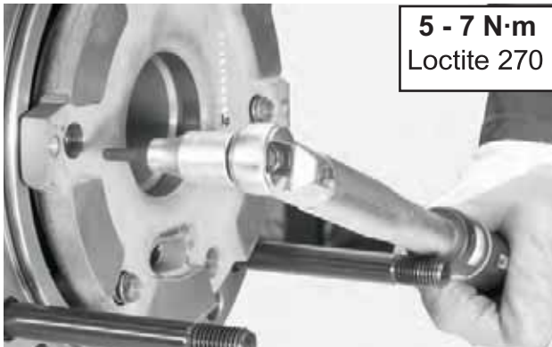
FIGURE 33: Fit the pin screws making sure that they are all of the same color. Apply Loctite 270 to the thread. Torque wrench setting: 5 - 7 N·m.
