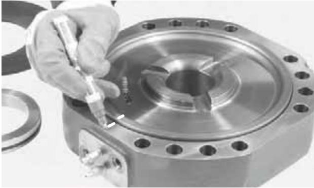
FIGURE 12: Write down their order of assembly and mark and remove negative piston sign the position.
