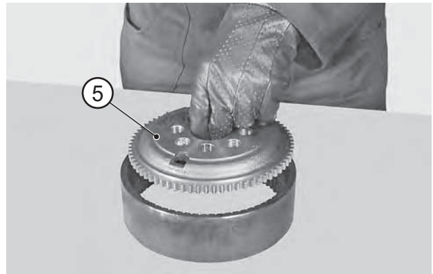
FIGURE 10: Remove the crown flange (5).
