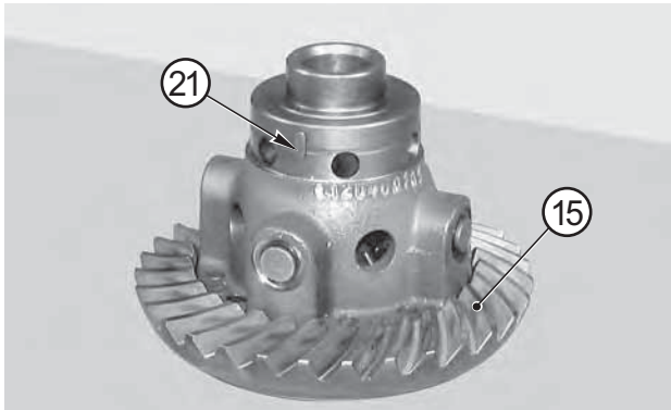
FIGURE 15: ONLY IF PREVIOUSLY DISASSEMBLED Assemble the differential unit (15). (For details, see DIFFERENTIAL UNIT p. 61). Position the key (21) in the differential unit (19).
