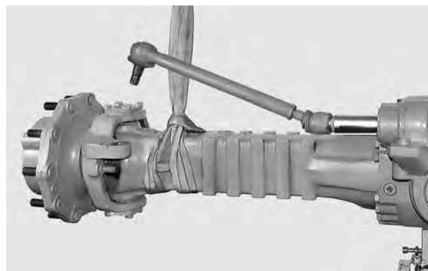
FIGURE 19: Re-install the complete arms. For details, see CHECKING WEAR AND REPLACING THE BRAKING DISCS p. 19.
