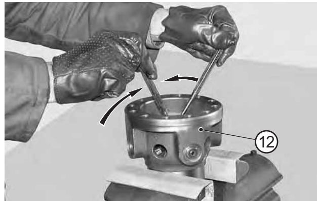
FIGURE 10: Remove tool T1 (See drawing T1 p. 131) together with the pin (9) of the planetary gear.
