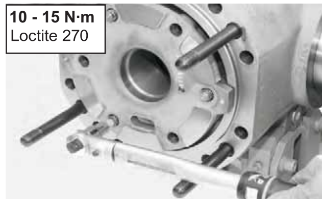
FIGURE 31: Apply LOCTITE 270 to the thread of the piston adjustment nut. Tighten with torque wrench setting of 10 - 15 N·m
