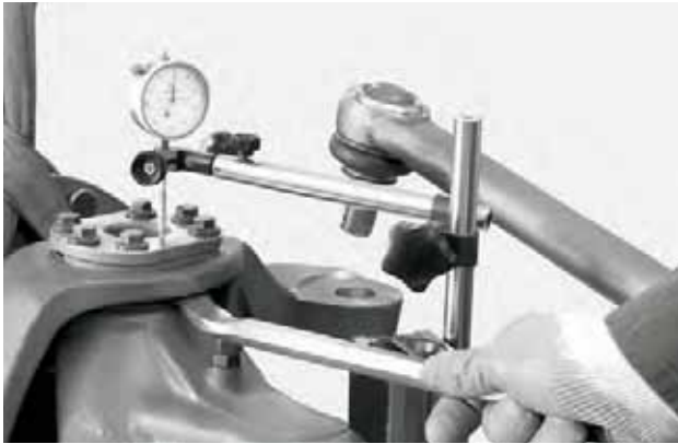
FIGURE 11: Check with a lever that there is no vertical gap. In case there is any gap, determine the width and reduce it by removing shims.
