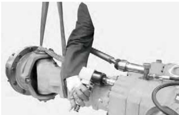
FIGURE 2: Sling the arm to be removed and connect it to a hoist.
