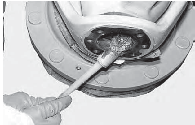
FIGURE 8: Lubricate steering case.
