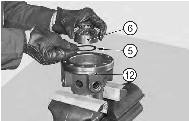
FIGURE 13: Insert the shim washer (5) and the differential side gear (6) in the differential carrier (12).
