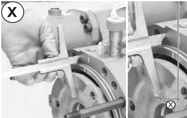
FIGURE 34: Take the measurement from the surface of the intermediate disk to the cover sealing surface with 30 bar of pressure introduced. EXAMPLE: 25.4 mm
