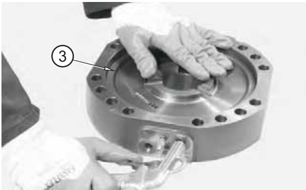
FIGURE 13: Slowly introduce low-pressure compressed air through the connection member for the negative brake, in order to extract the piston (3).
