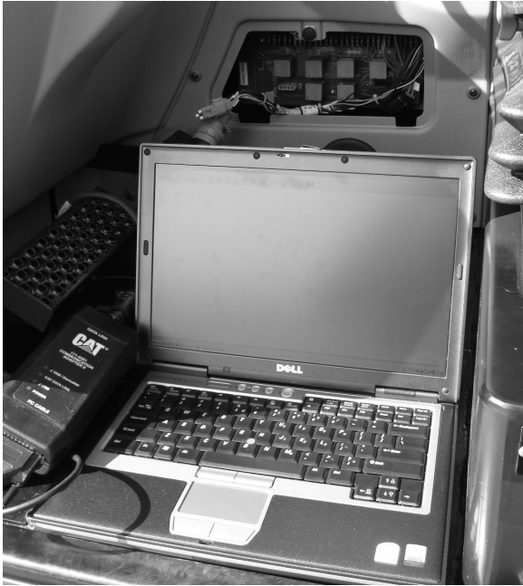
Illustration 53 This is the location of the service connector that contains the CAT data link. The connector is located to the side and rear of the seat.
