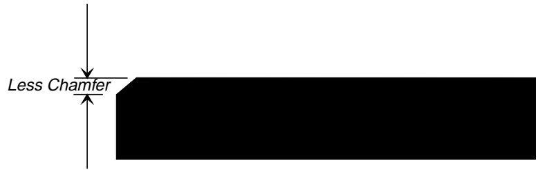
Fig. 6-30: Pad Worn, But Still OK
